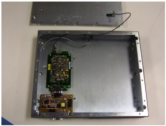
Cover and Antenna Assembly removed to show component layout.
