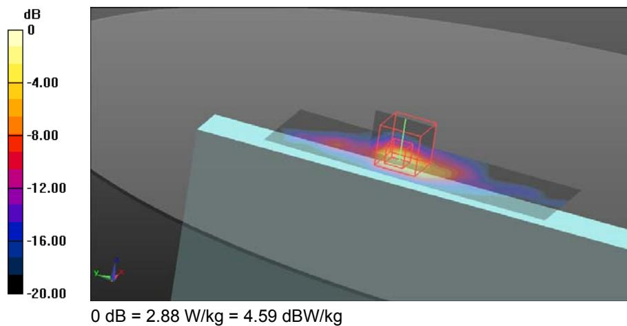
**6. 5.3GHz - 802.11a, CH52, Aux Antenna – Tablet PL**
