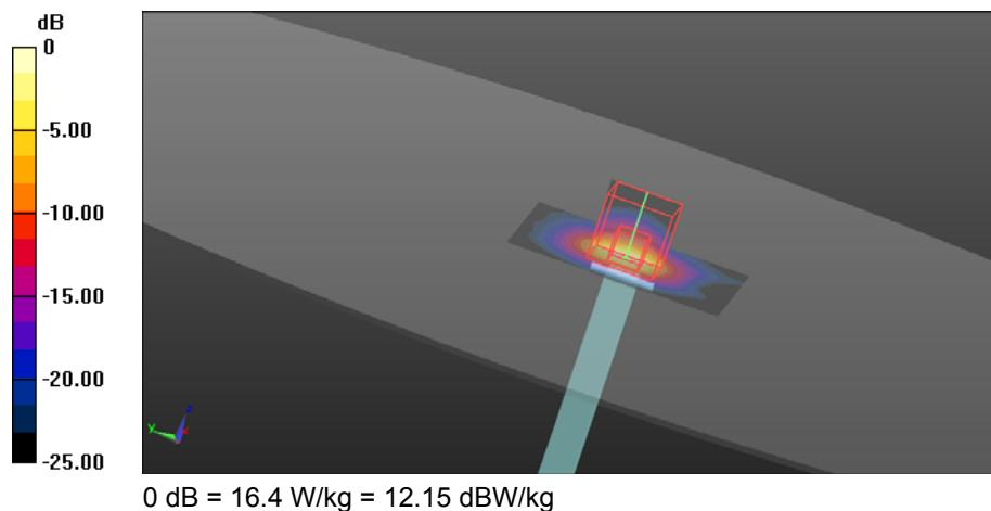
**15. System Check Body Liquid 5800MHz**
