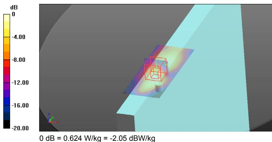
**3. 5.2GHz - 802.11n40, CH46, Main Antenna – Tablet PL**
