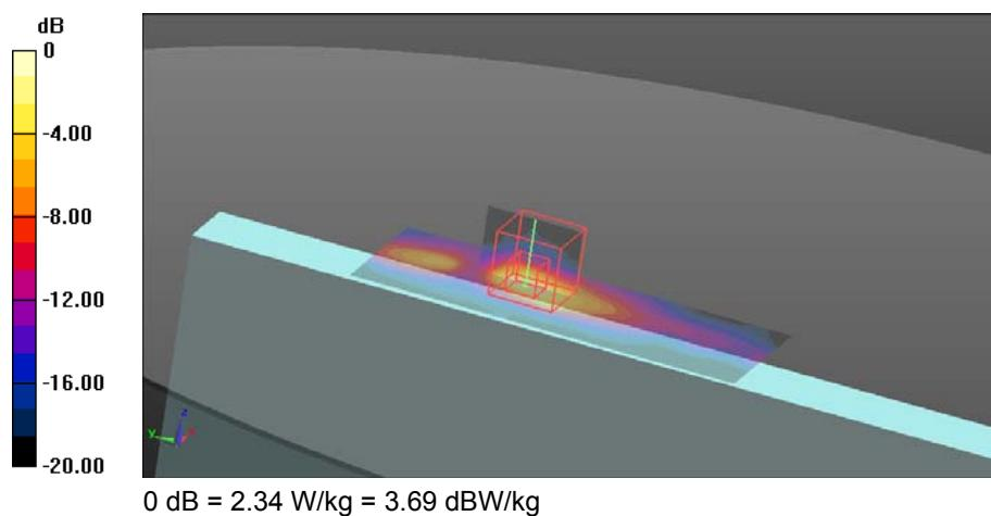
**8. 5.6GHz - 802.11a, CH104, Aux Antenna – Tablet PL**
