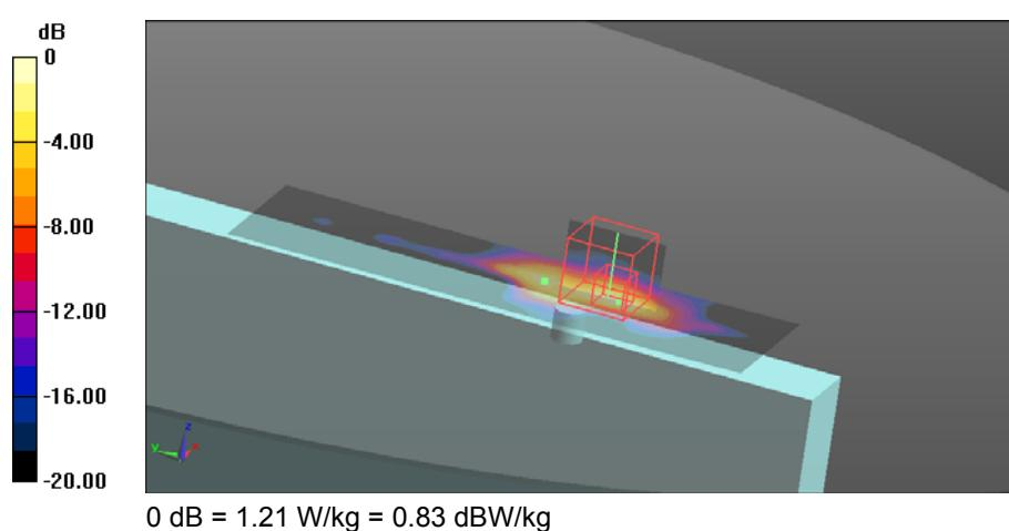
**9. 5.8GHz - 802.11ac80, CH155, Main Antenna – Tablet PL**
