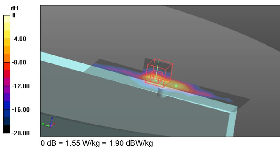
**5. 5.3GHz - 802.11a, CH60, Main Antenna – Tablet PL**
