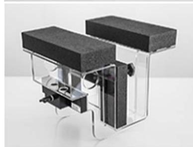
A simple but effective and easy-to-use extension for the Mounting Device; facilitates testing of larger devices according to IEC 62209-2 (e.g., laptops, cameras, etc.); lightweight and fits easily on the upper part of the Mounting Device in place of the phone positioner. The extension is fully compatible with the Twin SAM, ELI and other Flat Phantoms.
