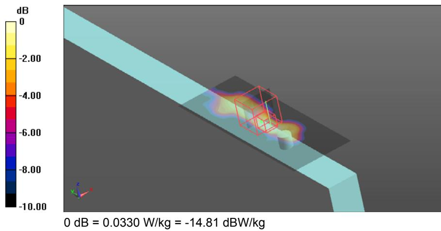
**12. System Check Body Liquid 2450MHz**
