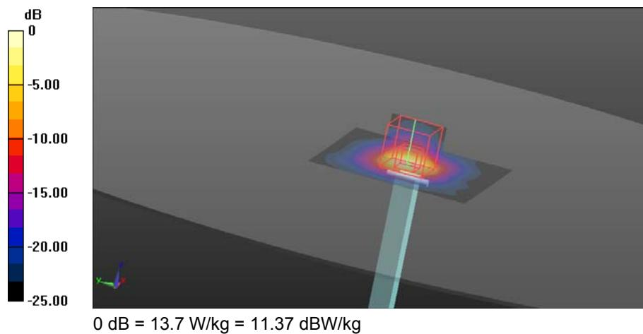
**14. System Check Body Liquid 5600MHz**
