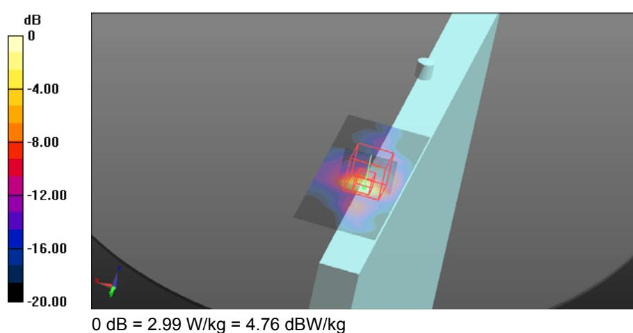
**4. 5.2GHz - 802.11n40, CH46, Aux Antenna – Tablet PL**
