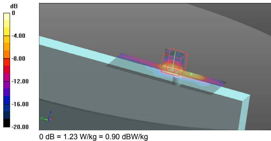
**7. 5.6GHz - 802.11ac80, CH138, Main Antenna – Tablet PL**
