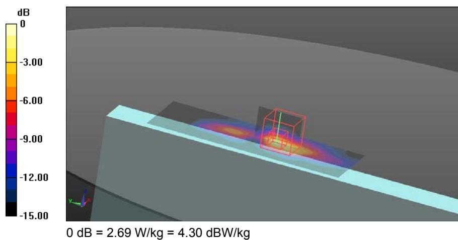
**10. 5.8GHz - 802.11n40, CH151, Aux Antenna – Tablet PL**
