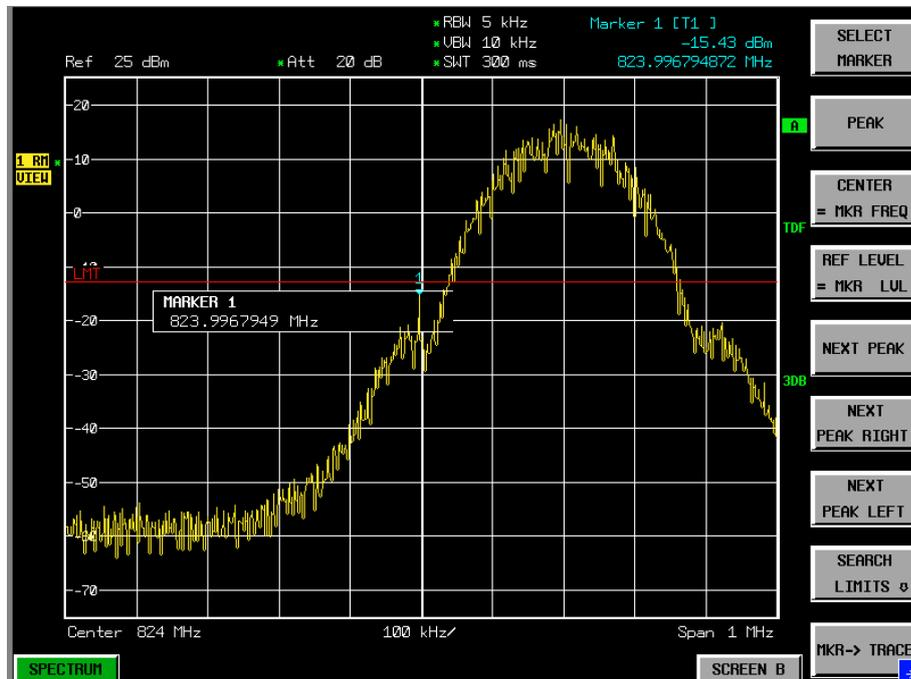
**HIGH BAND EDGE BLOCK-C (GSM850) –Channel 251**
