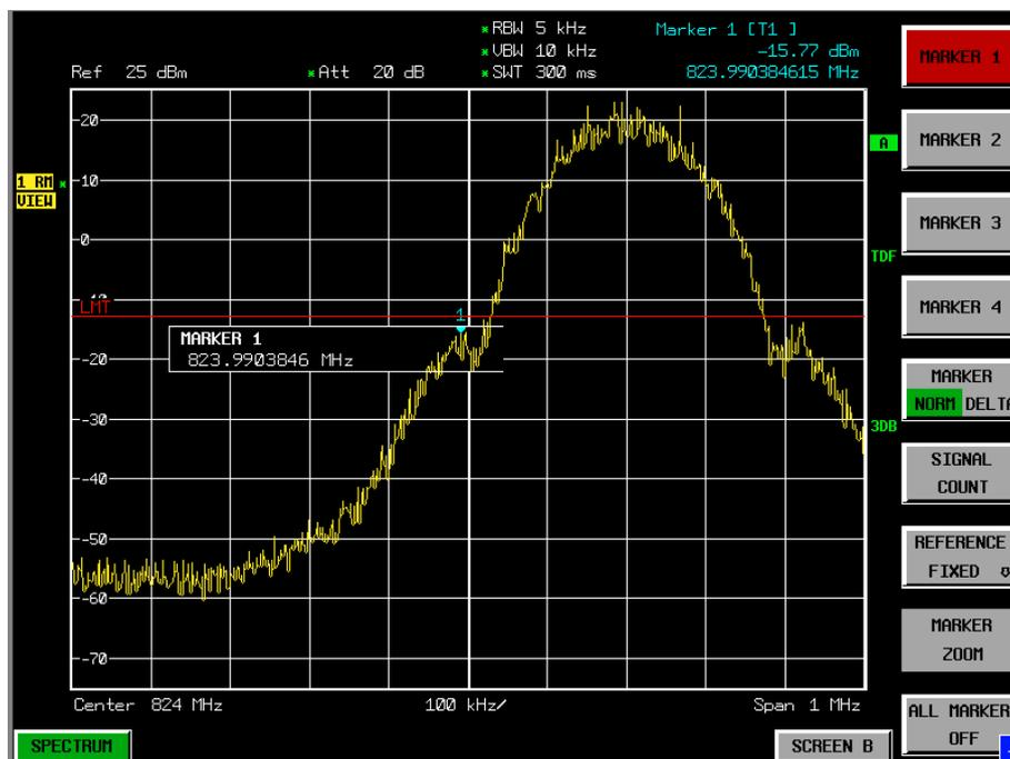
**HIGH BAND EDGE BLOCK-C (GSM850) –Channel 251**
