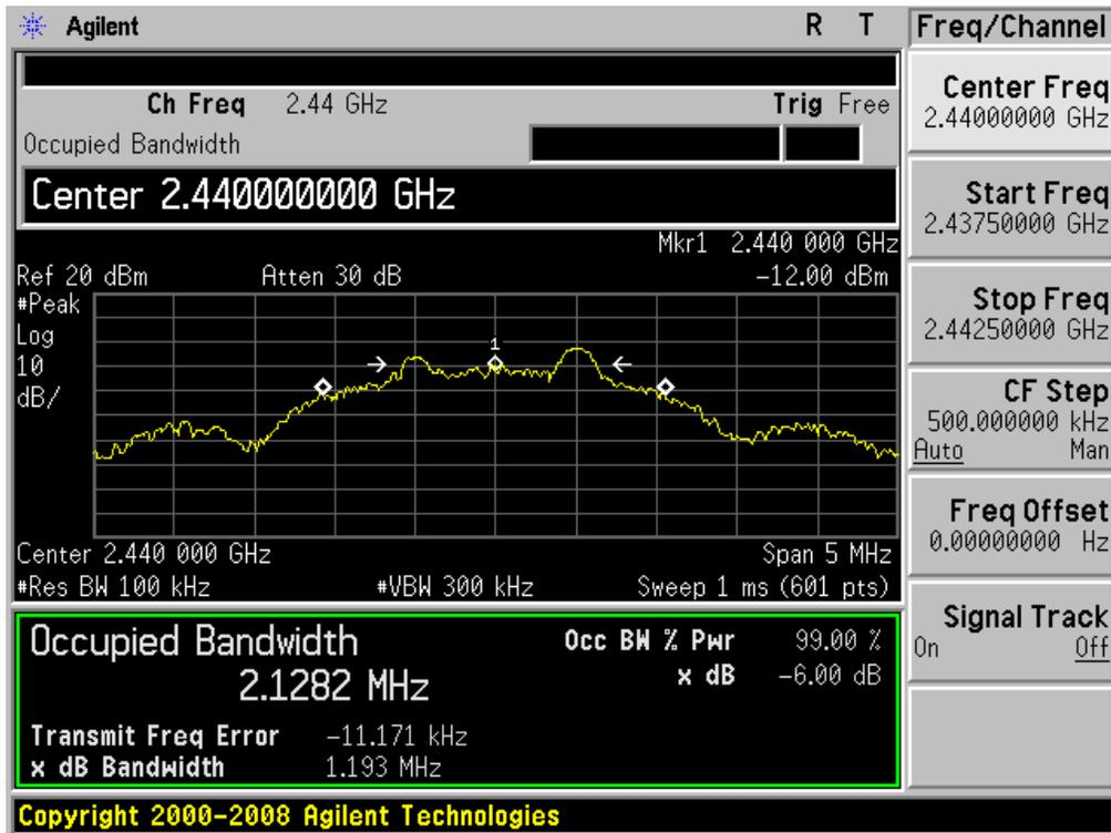
6dB Bandwidth plot on channel 34
