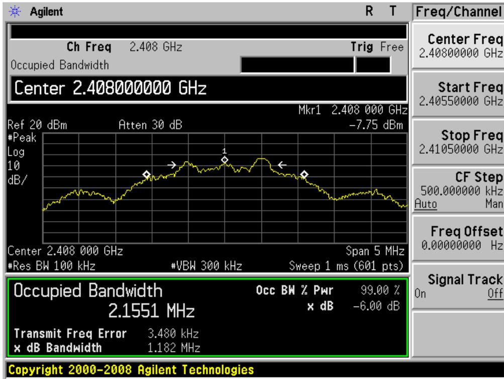
6dB Bandwidth plot on channel 17
