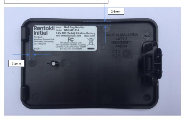
The adhesive backed barcode label should be adhered within the recessed detail on the underside of the base moulding (BBM Base A017) in the orientation shown
