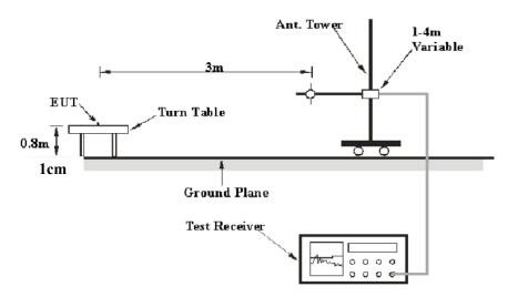
The radiated emission tests were performed in the 3 meters chamber test site, using the setup accordance with the ANSI C63.10-2013. The specification used was the FCC 15.209 and FCC 15.205 limits.
