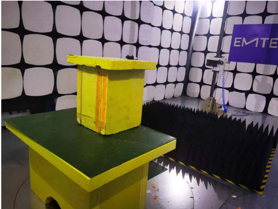
Spurious Emission Test Setup (Above 1GHz)
