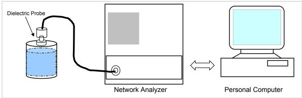
Set-up for liquid parameters check
