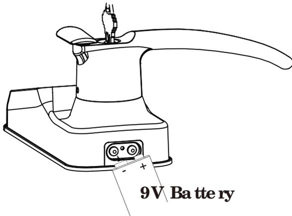
Your LOCKLY will automatically detect battery polarity. So hold your 9V battery lead in place against bottom of the LOCKLY to **temporarily** activate the screen to enter your **Access Code**. Be sure to hold the 9V battery against the contact points located at the bottom of the lock until you have successfully unlocked your door with your **Access Code**. Once unlocked, batteries should be replaced immediately.
