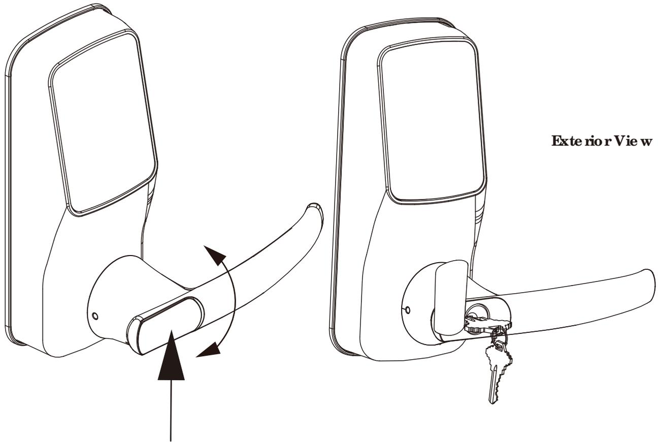
To **unlock** your lock using the **physical key (included)**, open the key cover on the handle by turning the cover to reveal the **keyhole**.
