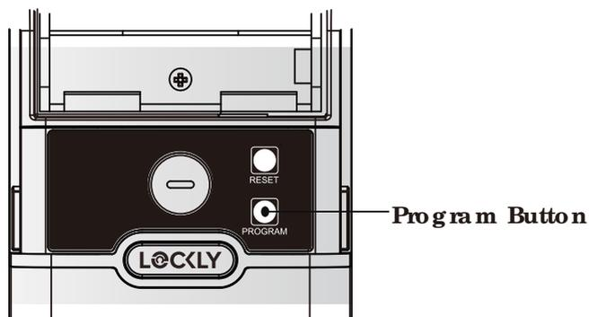
To enter **Programming Mode**, remove the battery compartment cover on the interior side of the lock to expose the **Reset** and **Program** buttons.
