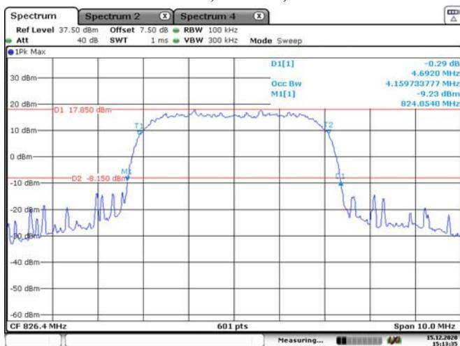
**WCDMA Band V, HSUPA, Middle Channel**
