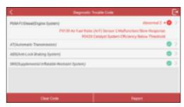
In above figure, the tested system with fault code appears in red and the system with OK displays in black (normally).
