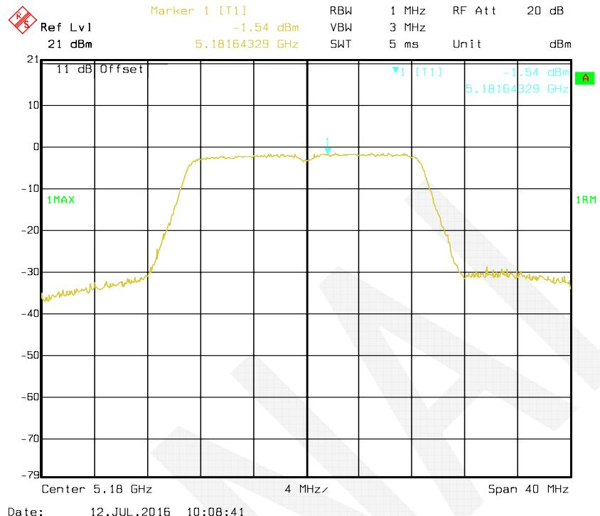
**802.11n HT20 mode, Antenna 2: Power Spectral Density-5220 MHz**
