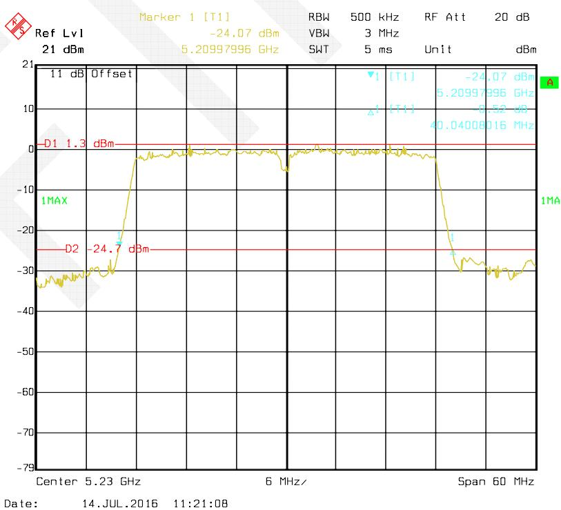
**802.11ac 80 mode, Antenna 1: 26 dB Bandwidth-5210 MHz**
