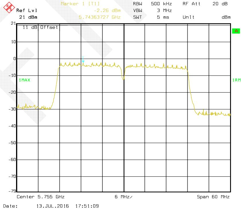
**802.11n HT40 mode, Antenna 2: Power Spectral Density-5795 MHz**
