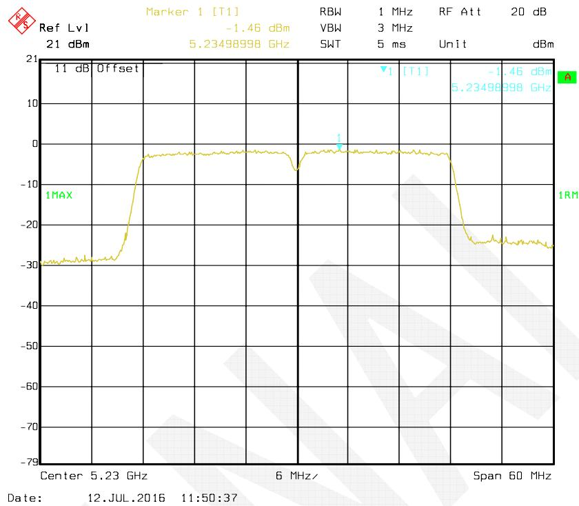
**802.11ac 80 mode, Antenna 2: Power Spectral Density-5210 MHz**
