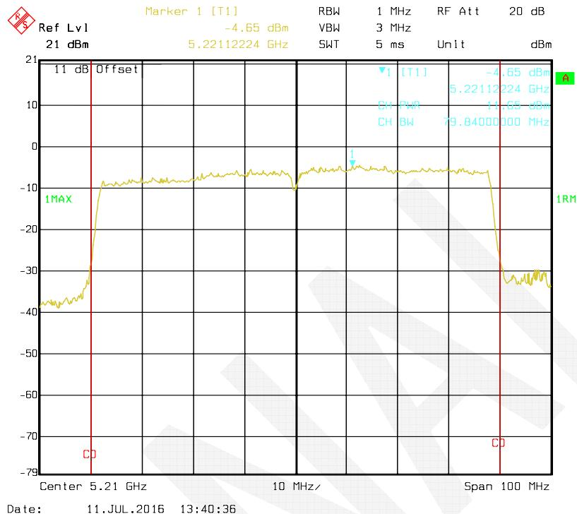
**802.11a, Antenna 2: RF Output Power-5180 MHz**
