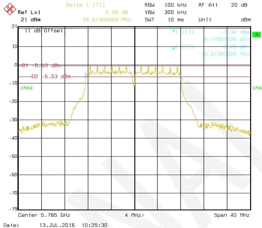
**802.11a mode, Antenna 2: 6 dB Bandwidth-5825 MHz**
