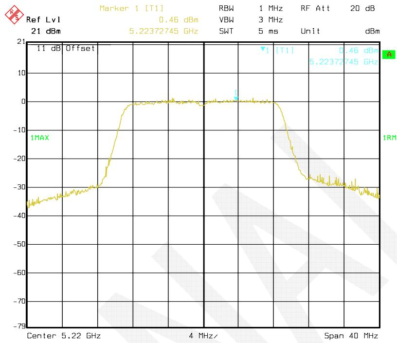
**802.11n HT20 mode, Antenna 1: Power Spectral Density-5240 MHz**
