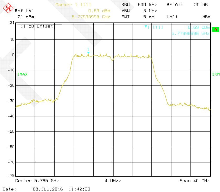
**802.11a mode, Antenna 1: Power Spectral Density-5825 MHz**
