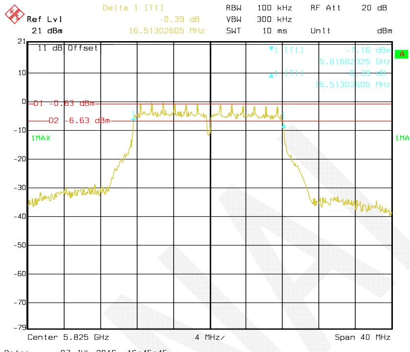
**802.11n HT20 mode, Antenna 1: 6 dB Bandwidth-5745 MHz**
