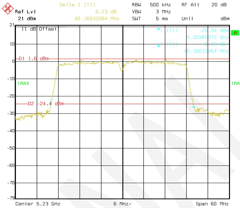
**802.11ac 80 mode, Antenna 2: 26 dB Bandwidth-5210 MHz**
