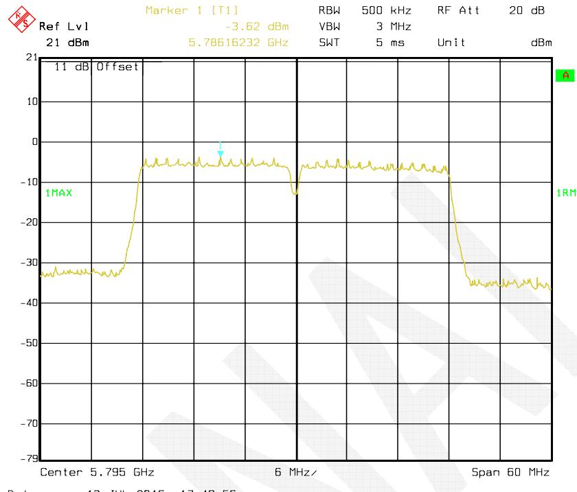
**802.11ac 80 mode, Antenna 2: Power Spectral Density-5775 MHz**
