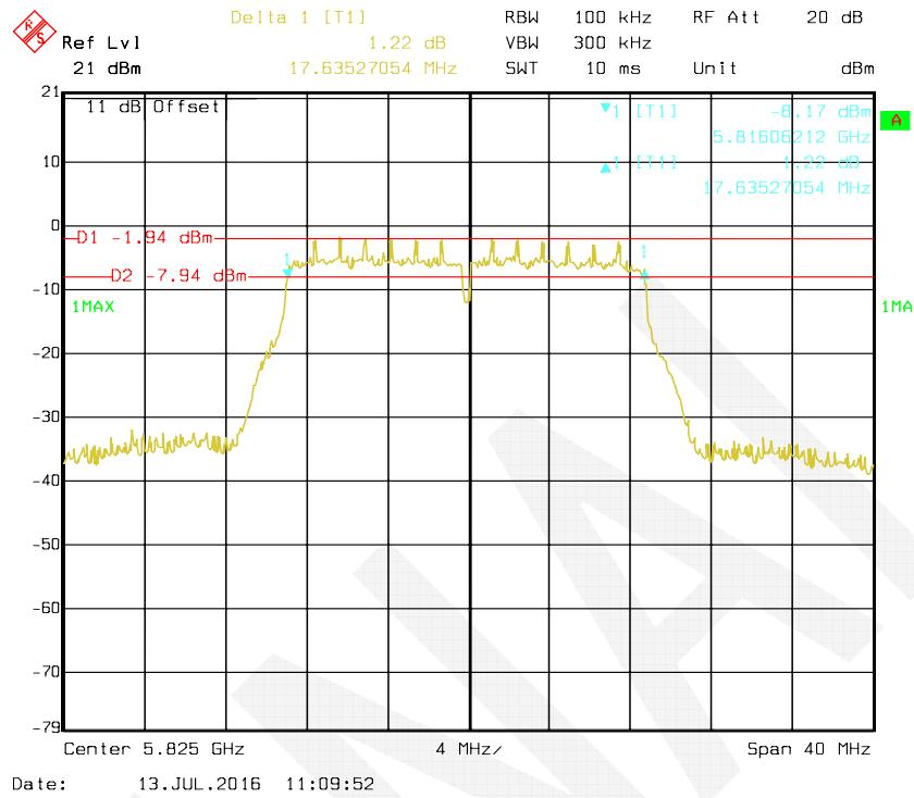
**802.11n HT40 mode, Antenna 2: 6 dB Bandwidth-5755 MHz**
