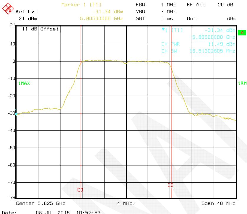
**802.11n HT20 mode, Antenna 1: RF Output Power-5745 MHz**
