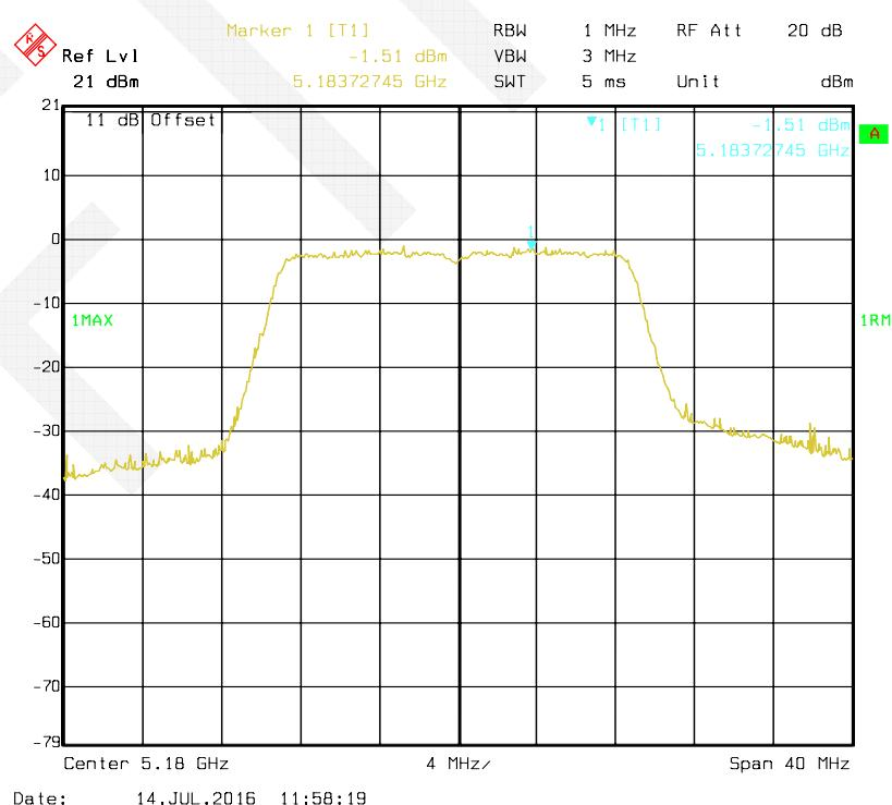
**802.11n HT20 mode, Antenna 1: Power Spectral Density-5220 MHz**
