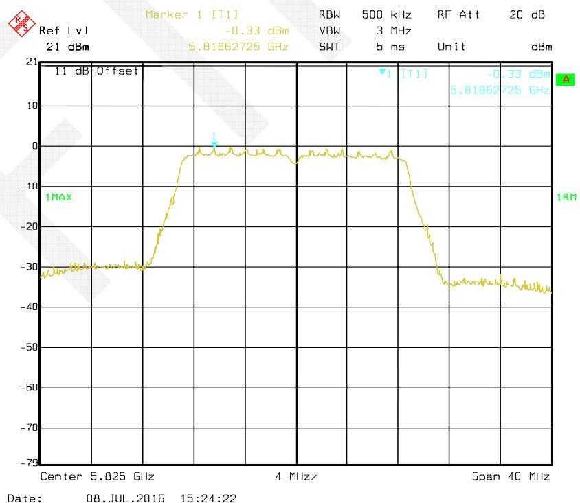
**802.11n HT40 mode, Antenna 1: Power Spectral Density-5755 MHz**
