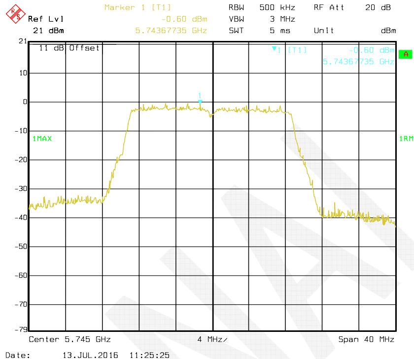
**802.11n HT20 mode, Antenna 2: Power Spectral Density-5785 MHz**
