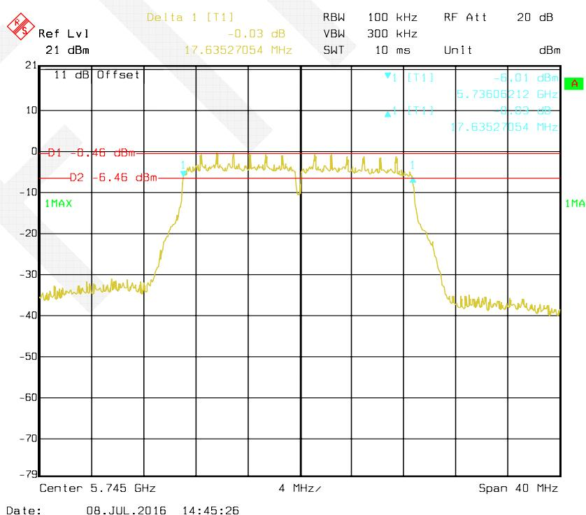
**802.11n HT20 mode, Antenna 1: 6 dB Bandwidth-5785 MHz**
