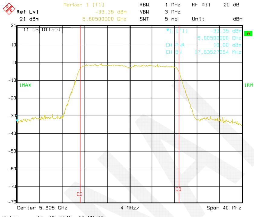
**802.11n HT40 mode, Antenna 2: RF Output Power-5755 MHz**
