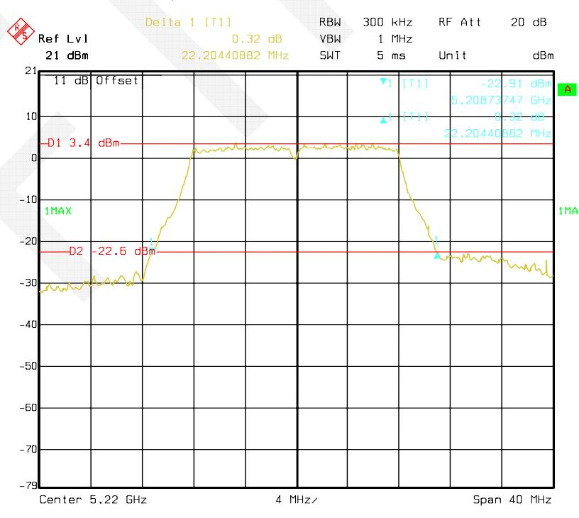
**802.11a mode, Antenna 1: 26 dB Bandwidth-5240 MHz**
