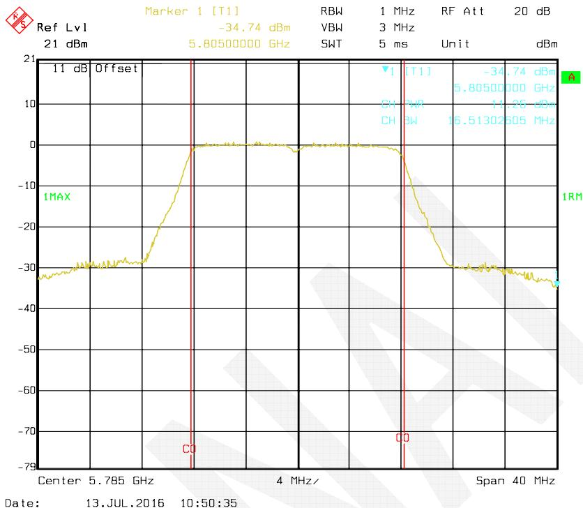
**802.11a, Antenna 2: RF Output Power-5825 MHz**
