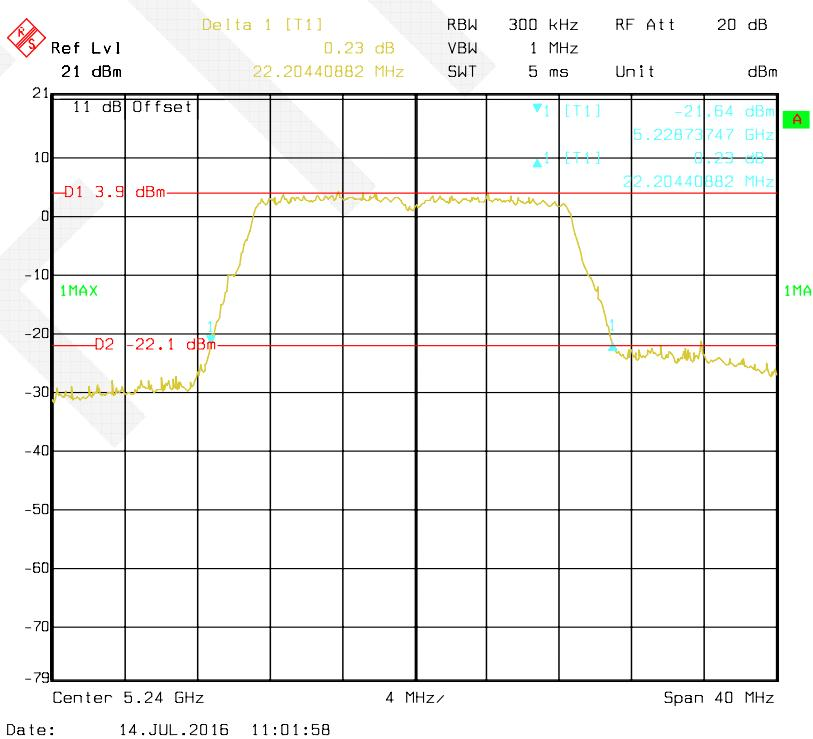
**802.11n HT40 mode, Antenna 1: 26 dB Bandwidth-5190 MHz**
