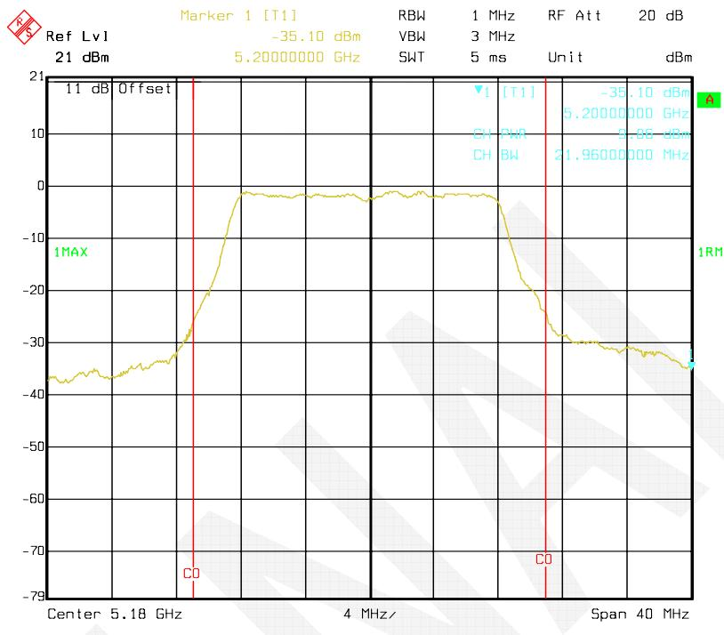
**802.11a, Antenna 1: RF Output Power-5220 MHz**
