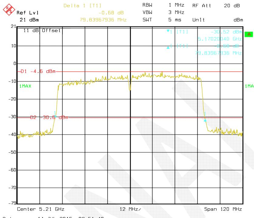
**802.11a mode, Antenna 2: 26 dB Bandwidth-5180 MHz**
