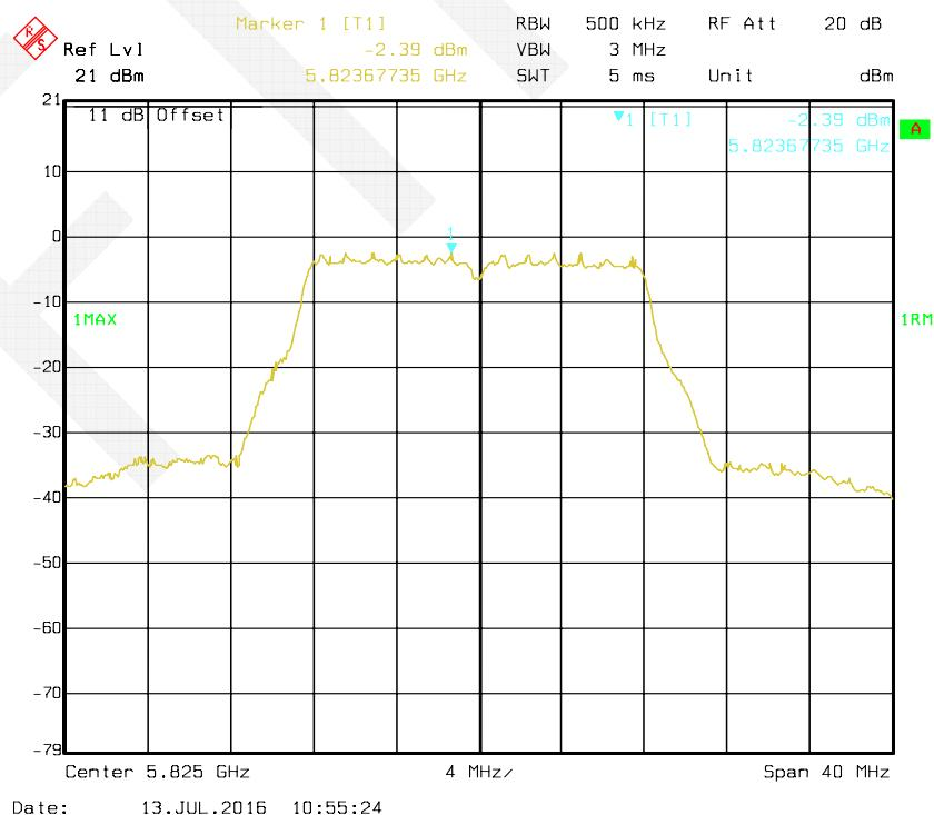
**802.11n HT20 mode, Antenna 2: Power Spectral Density-5745 MHz**
