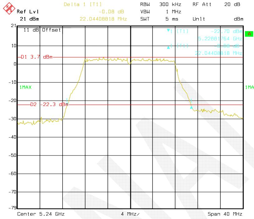
**802.11n HT20 mode, Antenna 1: 26 dB Bandwidth-5180 MHz**
