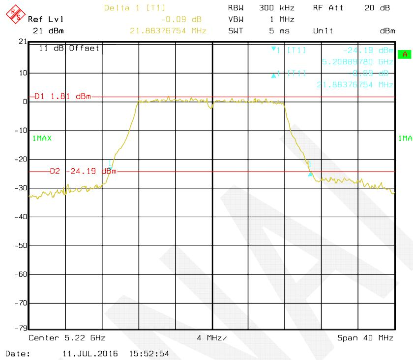
**802.11a mode, Antenna 2: 26 dB Bandwidth-5240 MHz**
