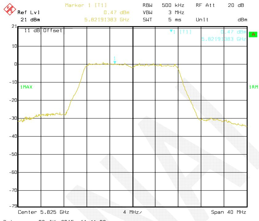
**802.11n HT20 mode, Antenna 1: Power Spectral Density-5745 MHz**
