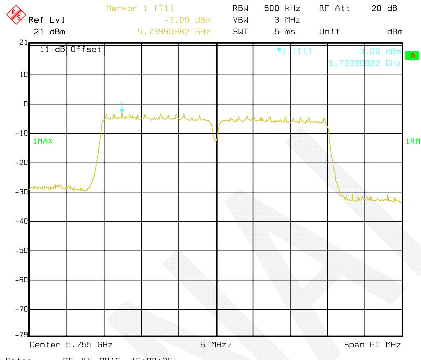
**802.11n HT40 mode, Antenna 1: Power Spectral Density-5795 MHz**
