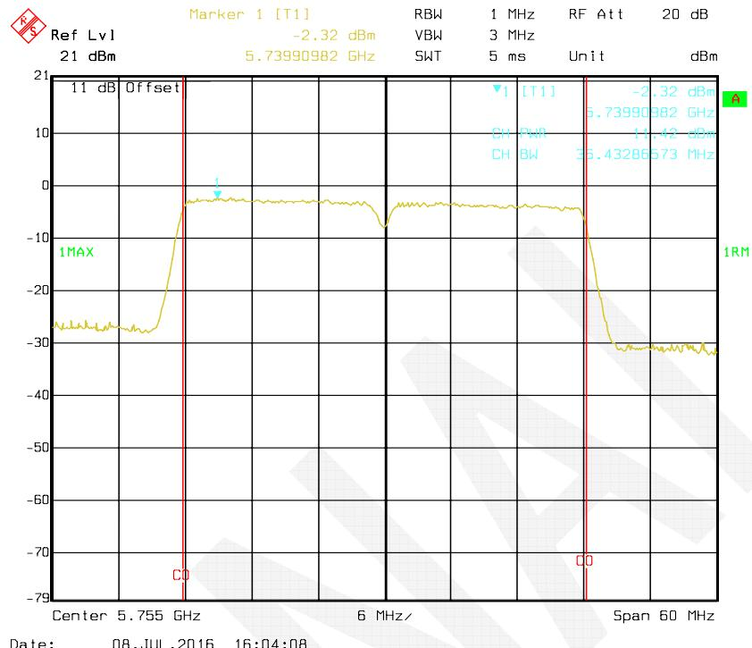
**802.11n HT40 mode, Antenna 1: RF Output Power-5795 MHz**
