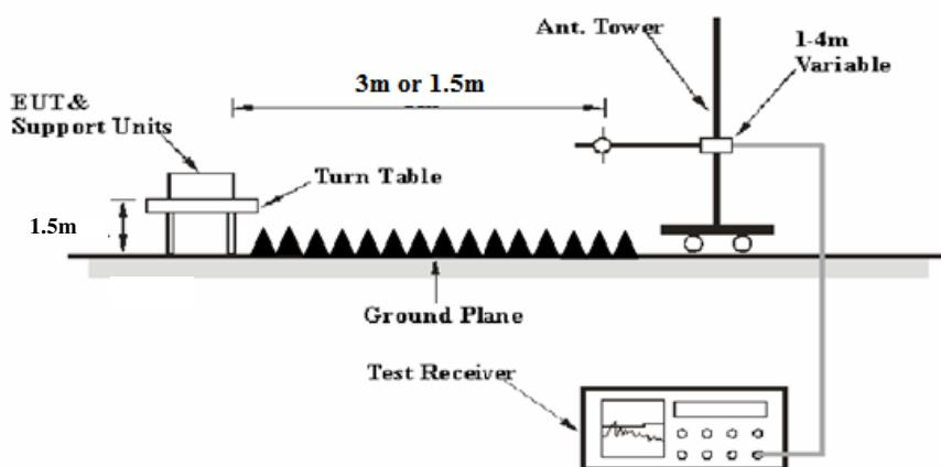
The radiated emission tests were performed in the 3 meters semi-anechoic chamber, using the setup accordance with the ANSI C63.10-2013. The specification used was the FCC 15.209 and FCC 15.407 limits.
