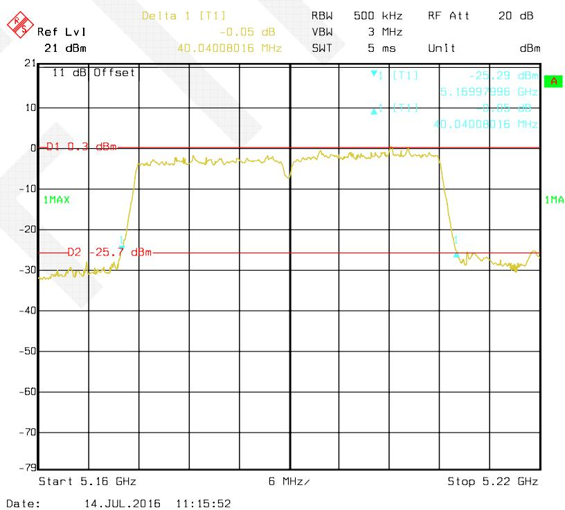
**802.11n HT40 mode, Antenna 2: 26 dB Bandwidth-5230 MHz**
