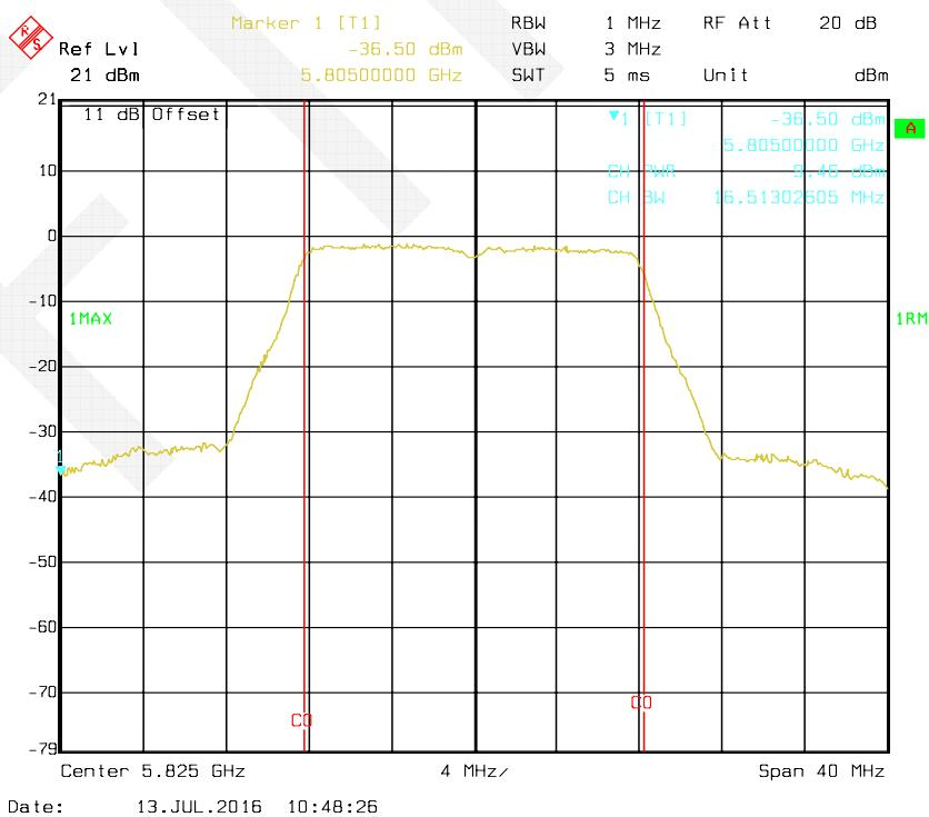
**802.11n HT20 mode, Antenna 2: RF Output Power-5745 MHz**
