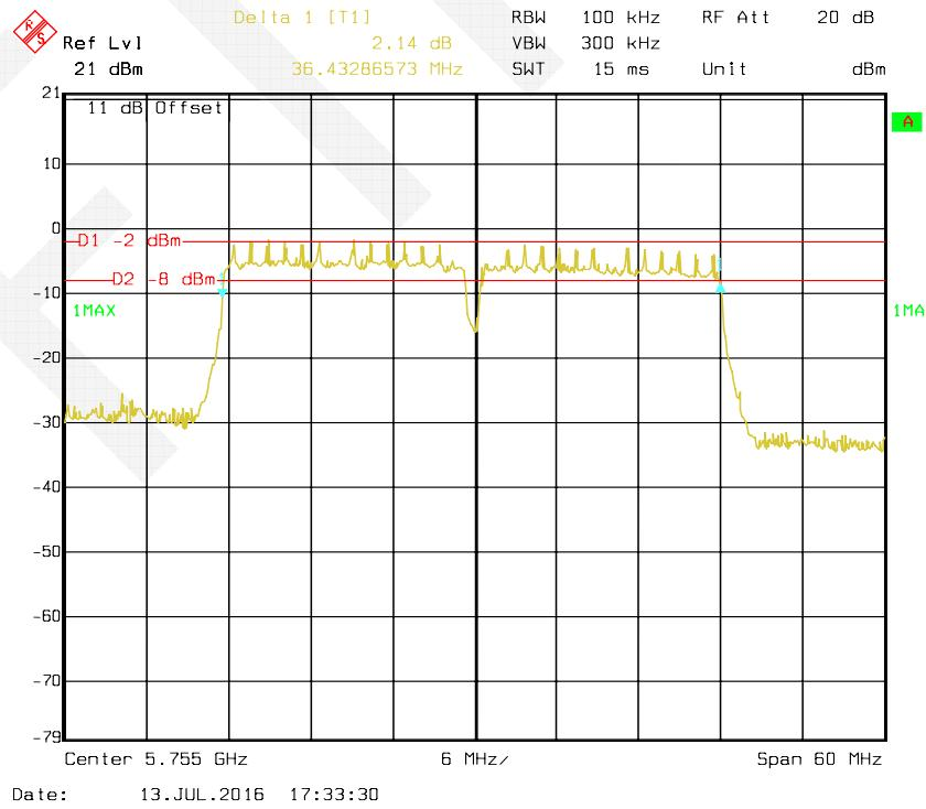
**802.11n HT40 mode, Antenna 2: 6 dB Bandwidth-5795 MHz**
