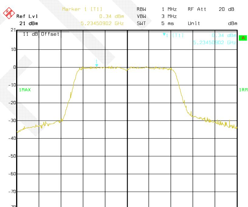
**802.11n HT40 mode, Antenna 1: Power Spectral Density-5190 MHz**
