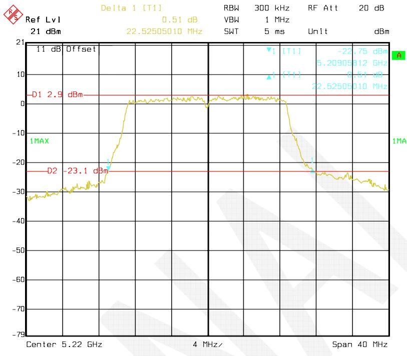
**802.11n HT20 mode, Antenna 1: 26 dB Bandwidth-5240 MHz**
