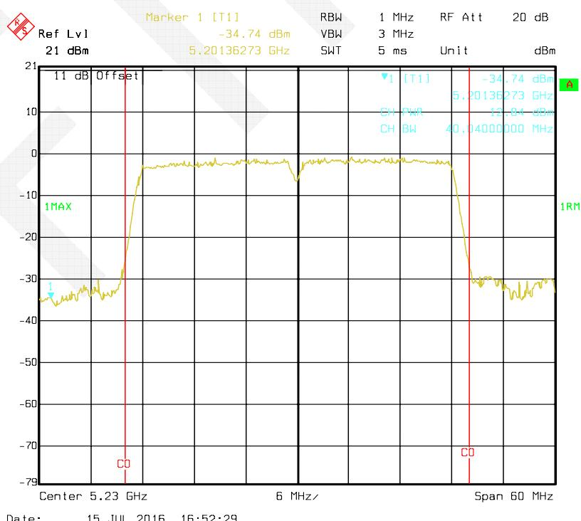
**802.11VHT80, Antenna 1: RF Output Power-5210 MHz**
