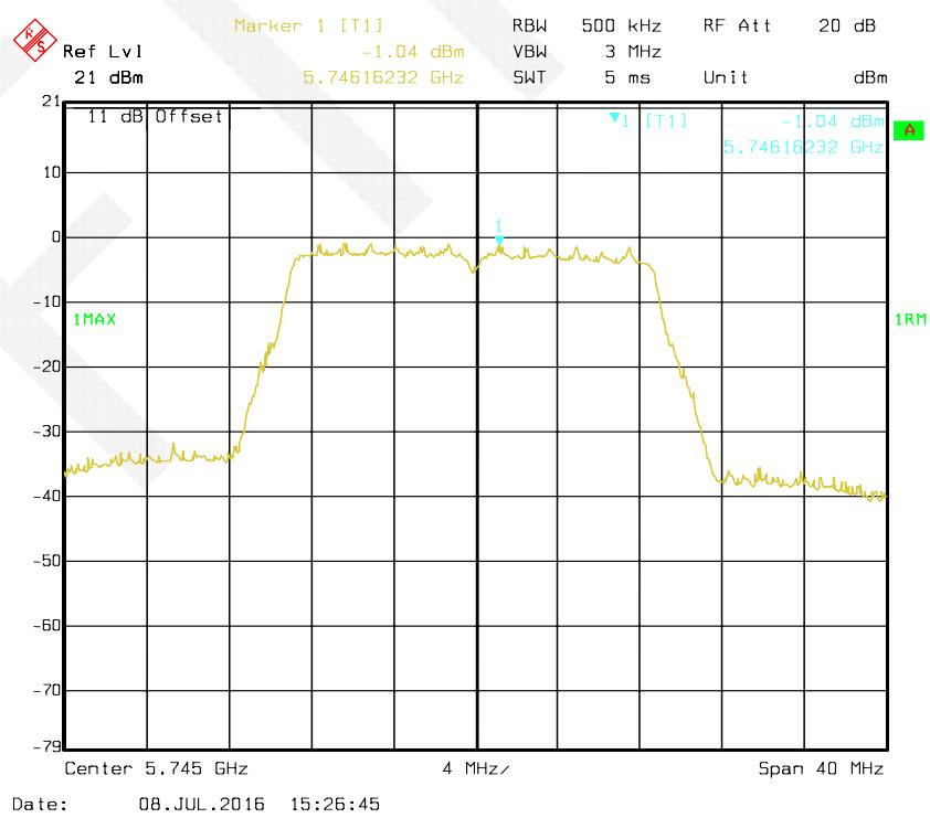
**802.11n HT20 mode, Antenna 1: Power Spectral Density-5785 MHz**
