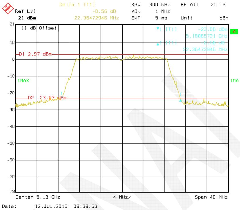
**802.11n HT20 mode, Antenna 2: 26 dB Bandwidth-5220 MHz**
