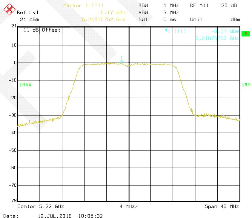
**802.11n HT20 mode, Antenna 2: Power Spectral Density-5240 MHz**
