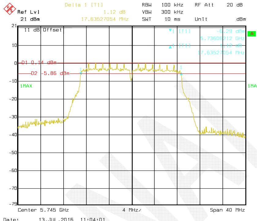
**802.11n HT20 mode, Antenna 2: 6 dB Bandwidth-5785 MHz**
