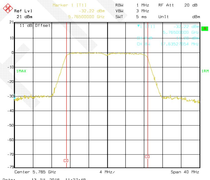
**802.11n HT20 mode, Antenna 2: RF Output Power-5825 MHz**
