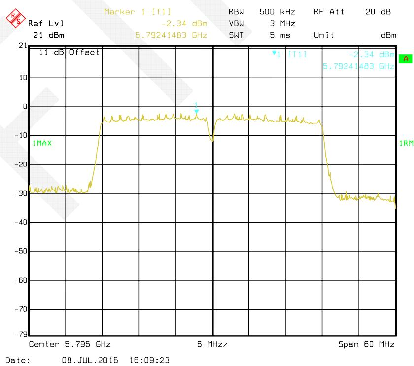
**802.11ac 80 mode, Antenna 1: Power Spectral Density-5775 MHz**
