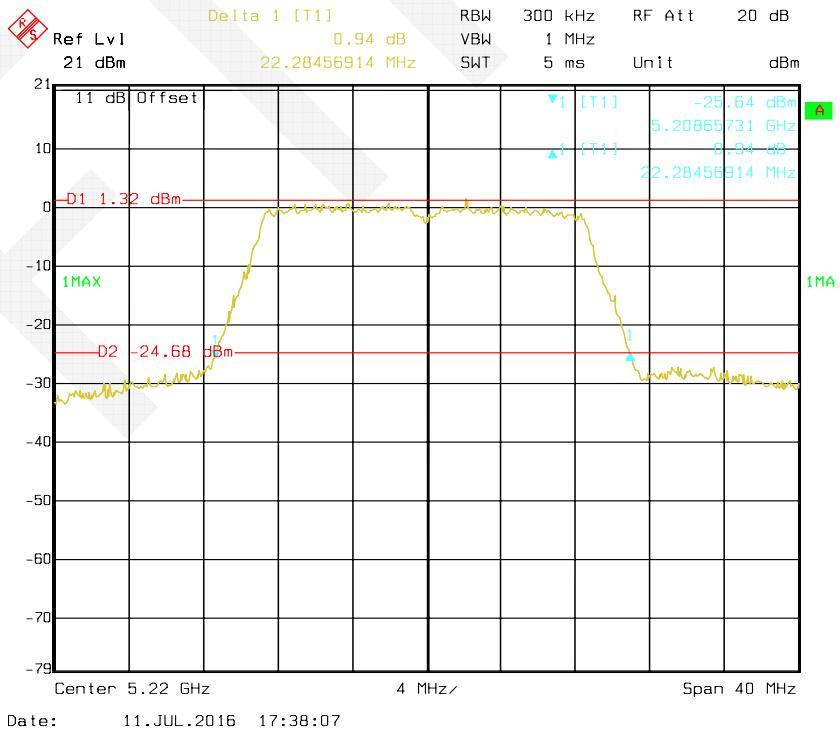
**802.11n HT20 mode, Antenna 2: 26 dB Bandwidth-5240 MHz**
