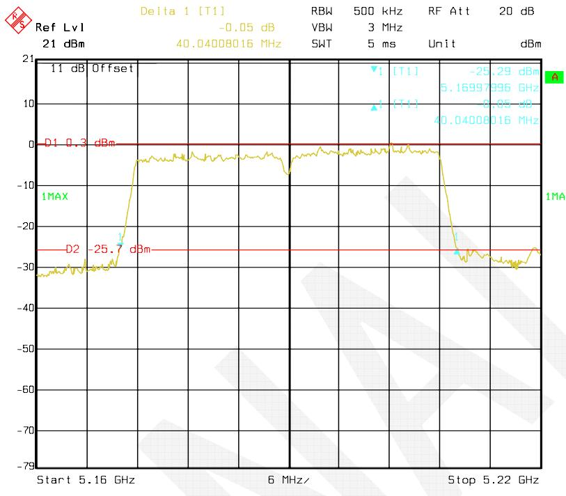
**802.11n HT40 mode, Antenna 1: 26 dB Bandwidth-5230 MHz**
