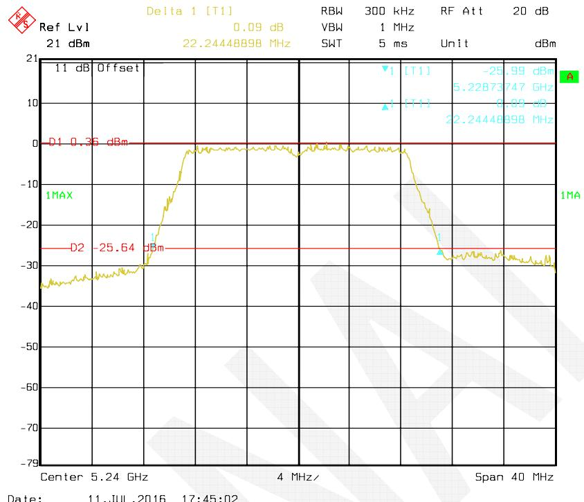
**802.11n HT40 mode, Antenna 2: 26 dB Bandwidth-5190 MHz**
