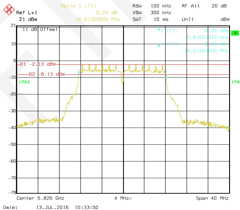
**802.11n HT20 mode, Antenna 2: 6 dB Bandwidth-5745 MHz**
