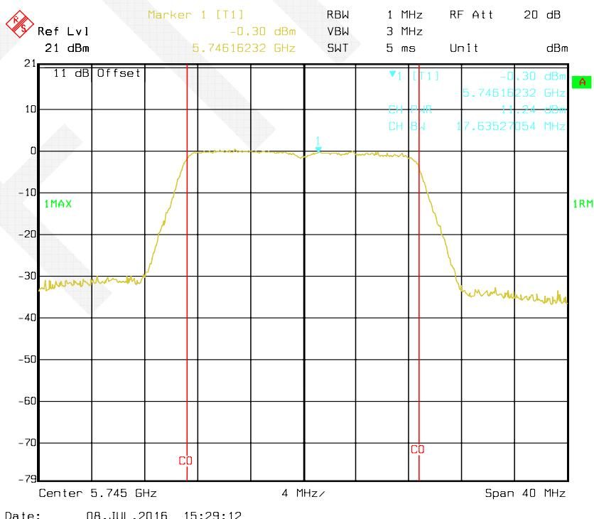
**802.11n HT20 mode, Antenna 1: RF Output Power-5785 MHz**
