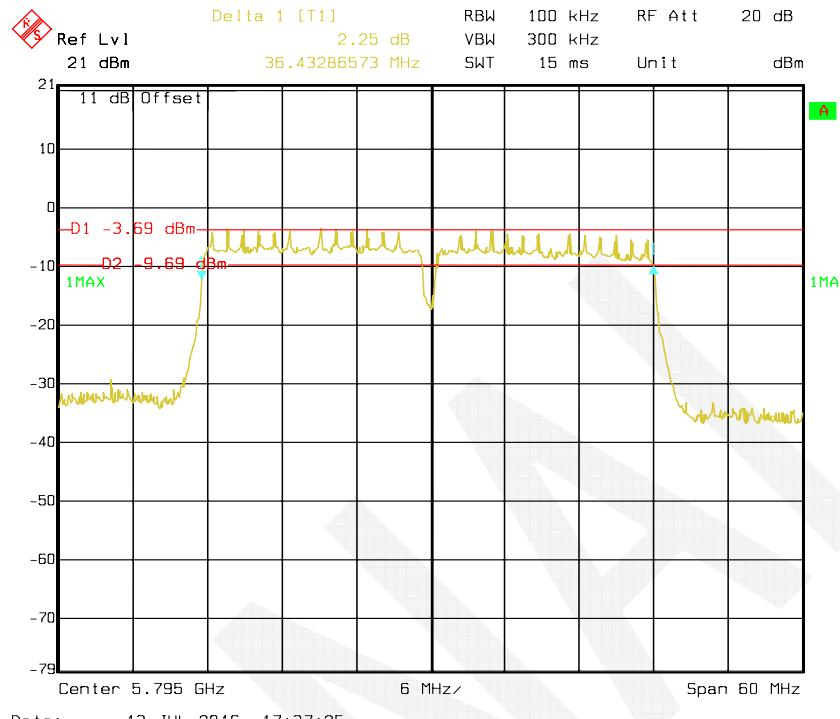
**802.11ac 80 mode, Antenna 2: 6 dB Bandwidth-5775 MHz**
