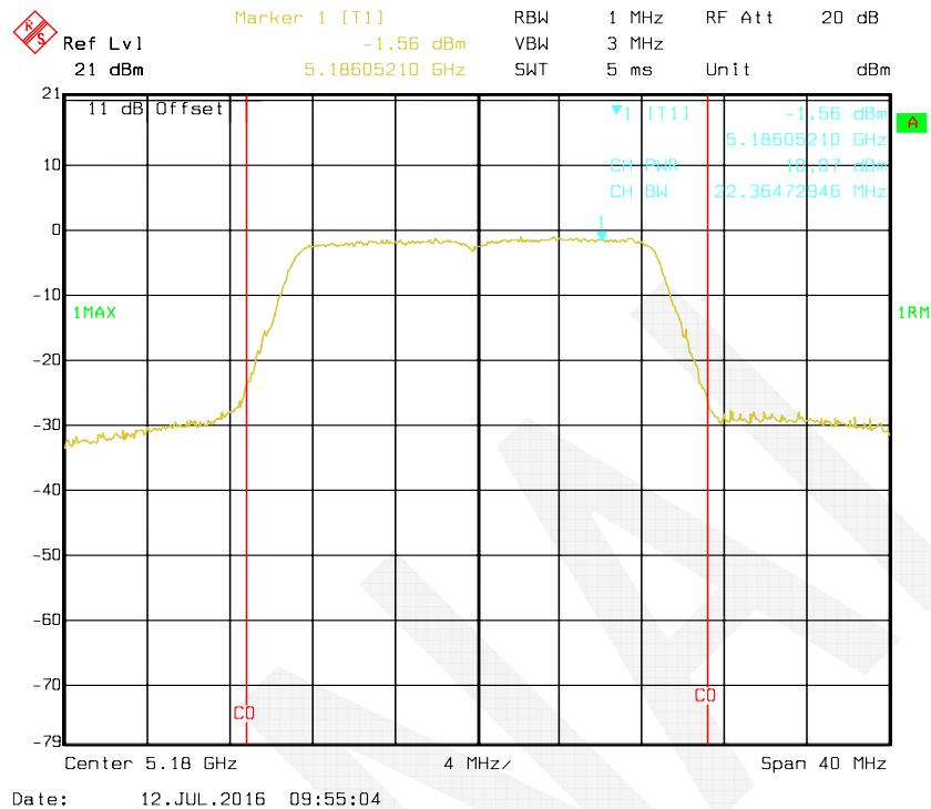
**802.11n HT20 mode, Antenna 2: RF Output Power-5220 MHz**
