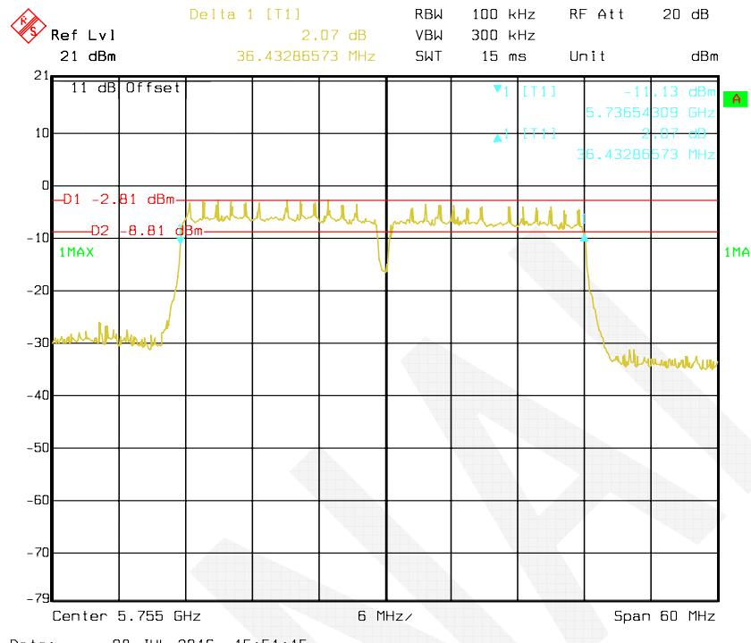
**802.11n HT40 mode, Antenna 1: 6 dB Bandwidth-5795 MHz**
