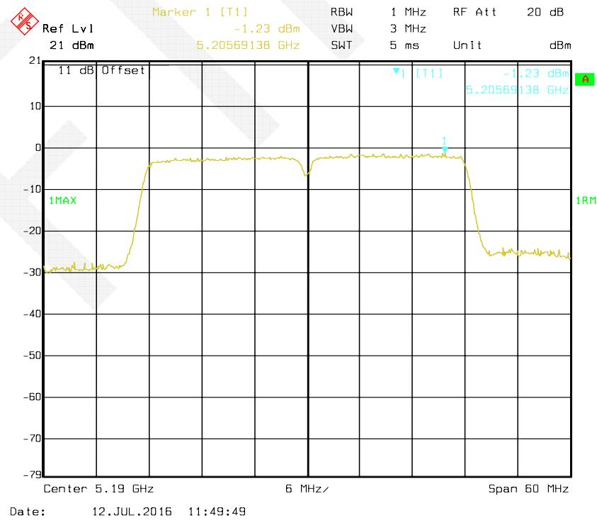
**802.11n HT40 mode, Antenna 2: Power Spectral Density-5230 MHz**
