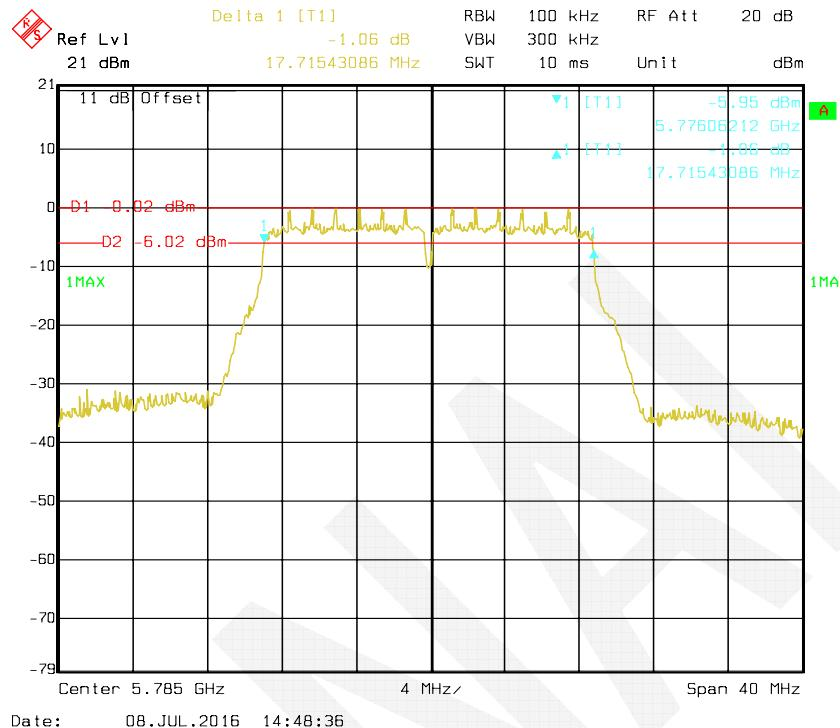
**802.11n HT20 mode, Antenna 1: 6 dB Bandwidth-5825 MHz**
