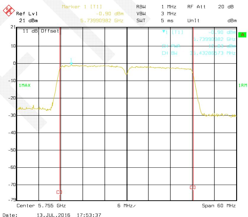
**802.11n HT40 mode, Antenna 2: RF Output Power-5795 MHz**
