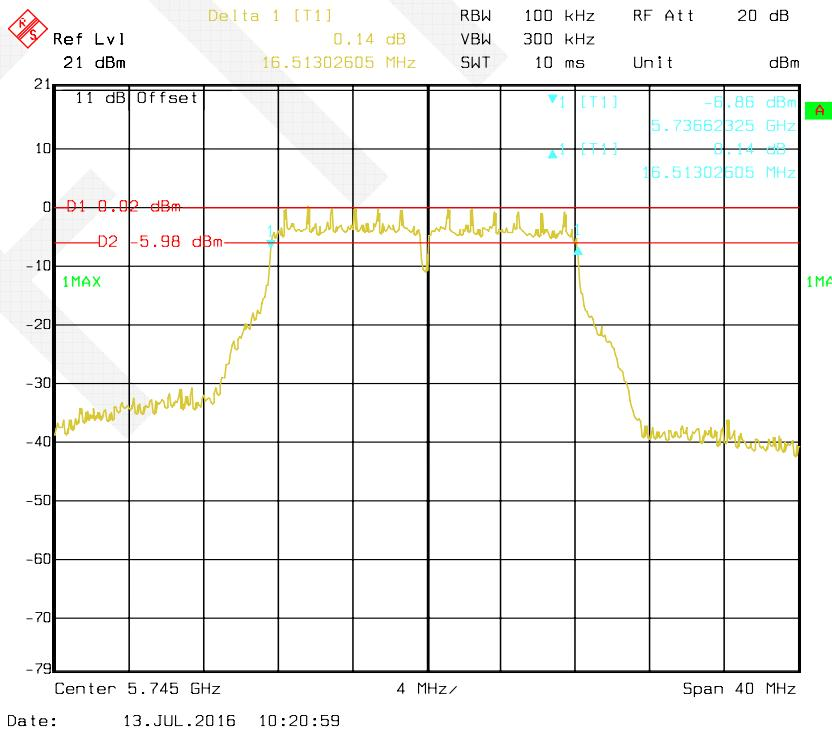
**802.11a mode, Antenna 2: 6 dB Bandwidth-5785 MHz**
