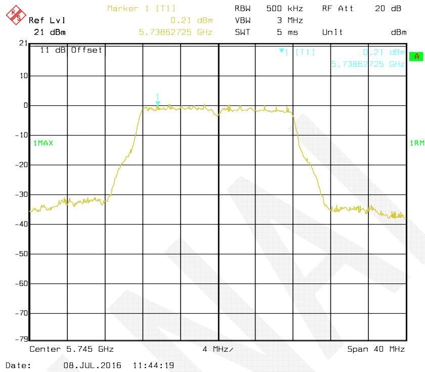
**802.11a mode, Antenna 1: Power Spectral Density-5785 MHz**
