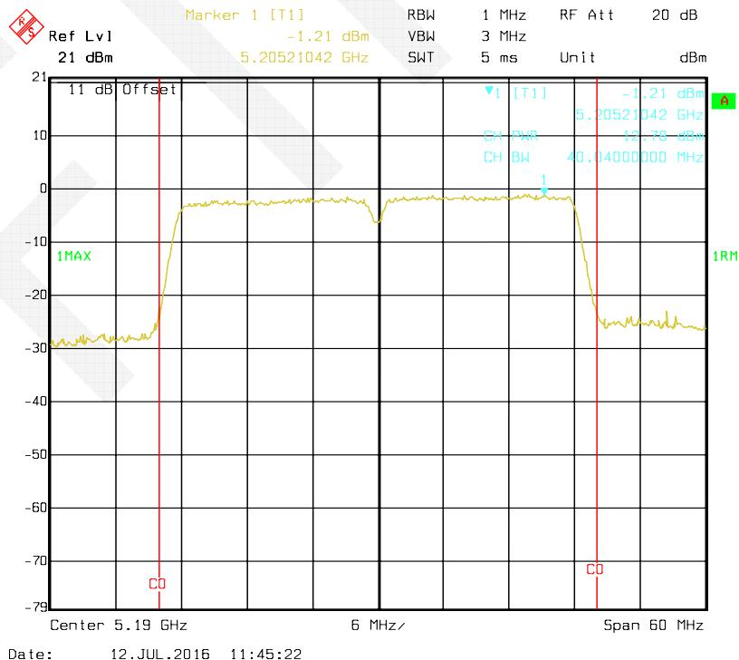
**802.11n HT40 mode, Antenna 2: RF Output Power-5230 MHz**
