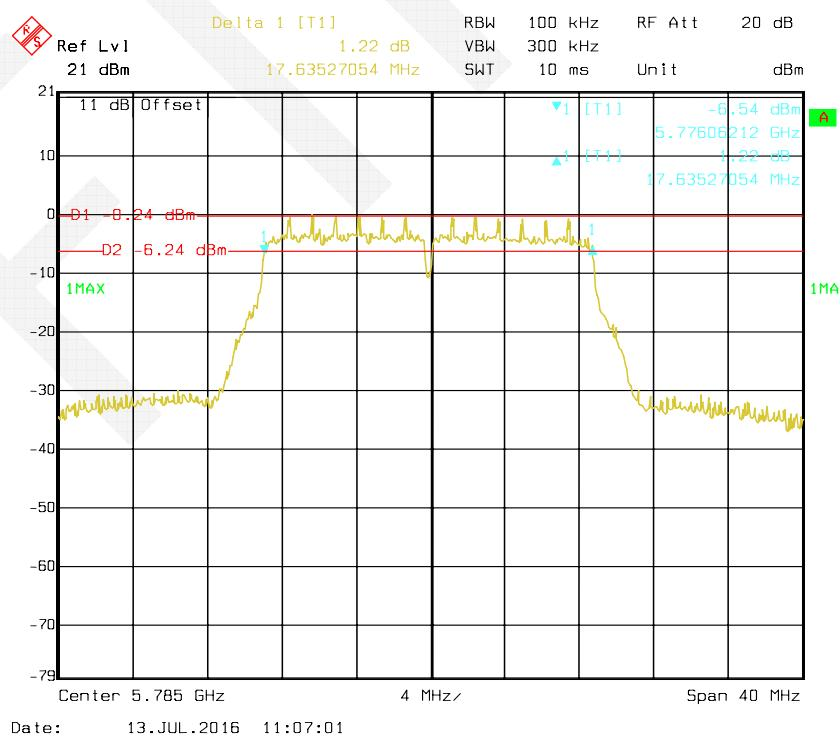
**802.11n HT20 mode, Antenna 2: 6 dB Bandwidth-5825 MHz**
