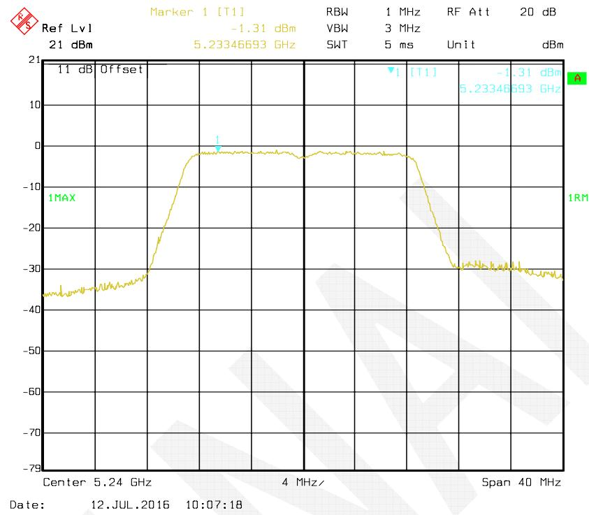
**802.11n HT40 mode, Antenna 2: Power Spectral Density-5190 MHz**
