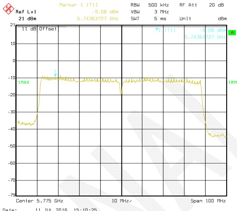
**802.11a mode, Antenna 2: Power Spectral Density-5745 MHz**
