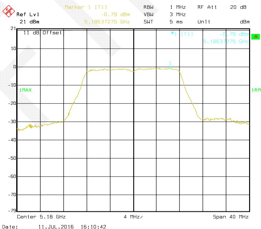
**802.11a mode, Antenna 2: Power Spectral Density-5220 MHz**
