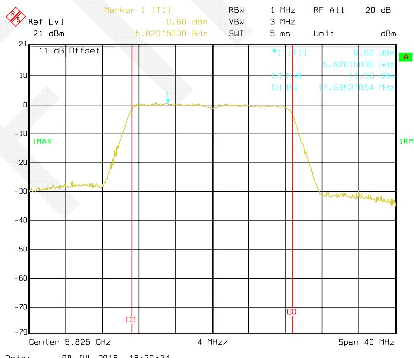
**802.11n HT40 mode, Antenna 1: RF Output Power-5755 MHz**
