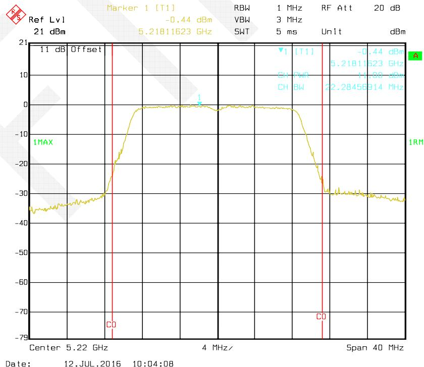
**802.11n HT20 mode, Antenna 2: RF Output Power-5240 MHz**
