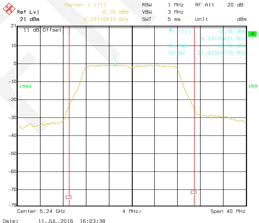
**802.11n HT20 mode, Antenna 2: RF Output Power-5180 MHz**
