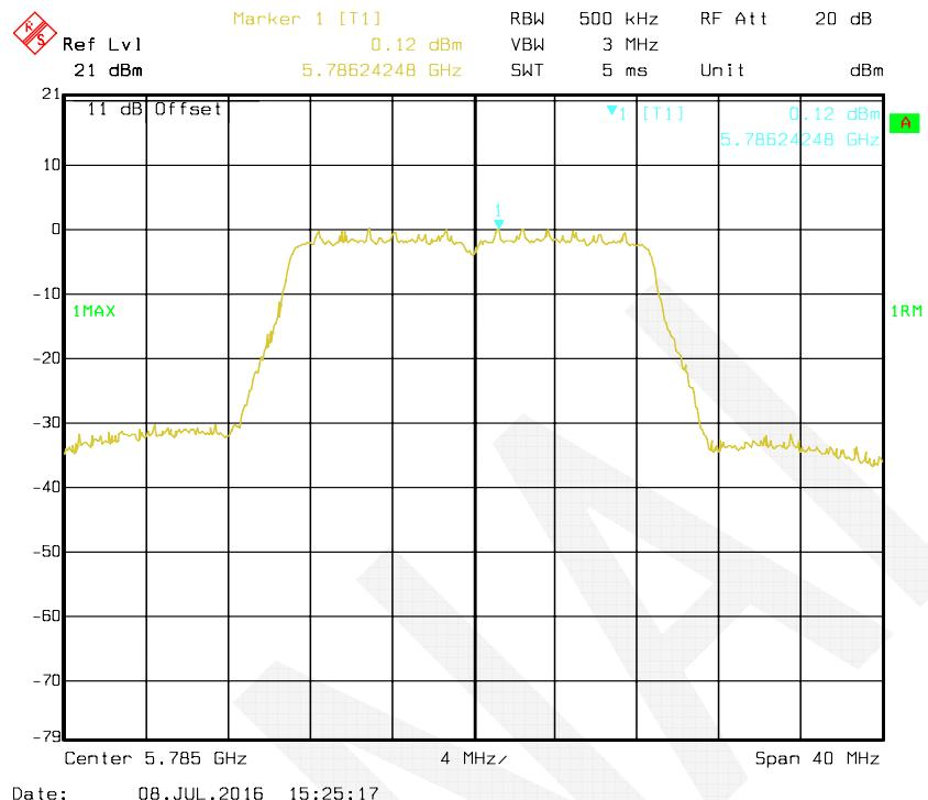
**802.11n HT20 mode, Antenna 1: Power Spectral Density-5825 MHz**
