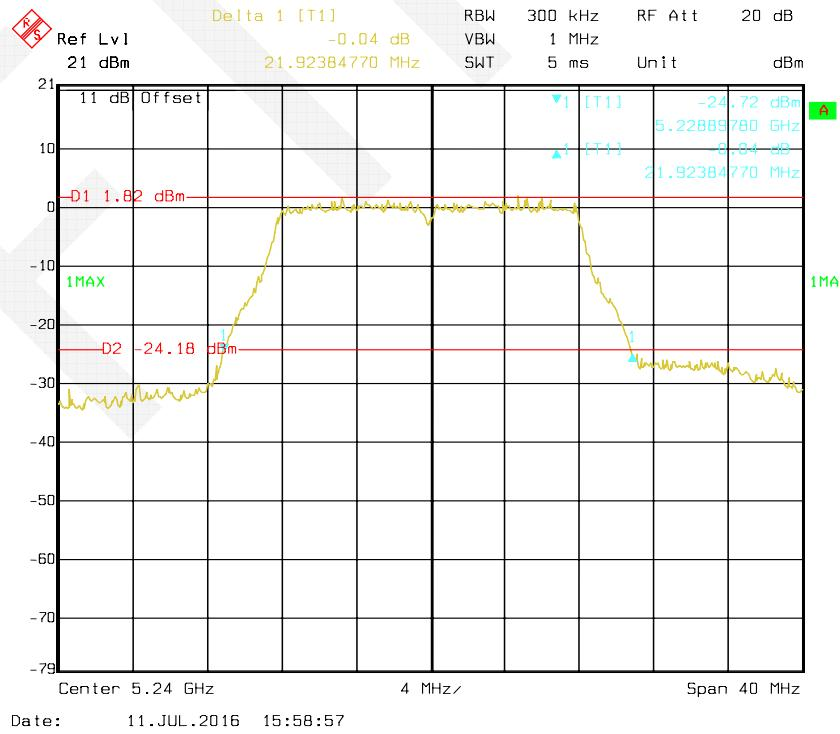
**802.11n HT20 mode, Antenna 2: 26 dB Bandwidth-5180 MHz**
