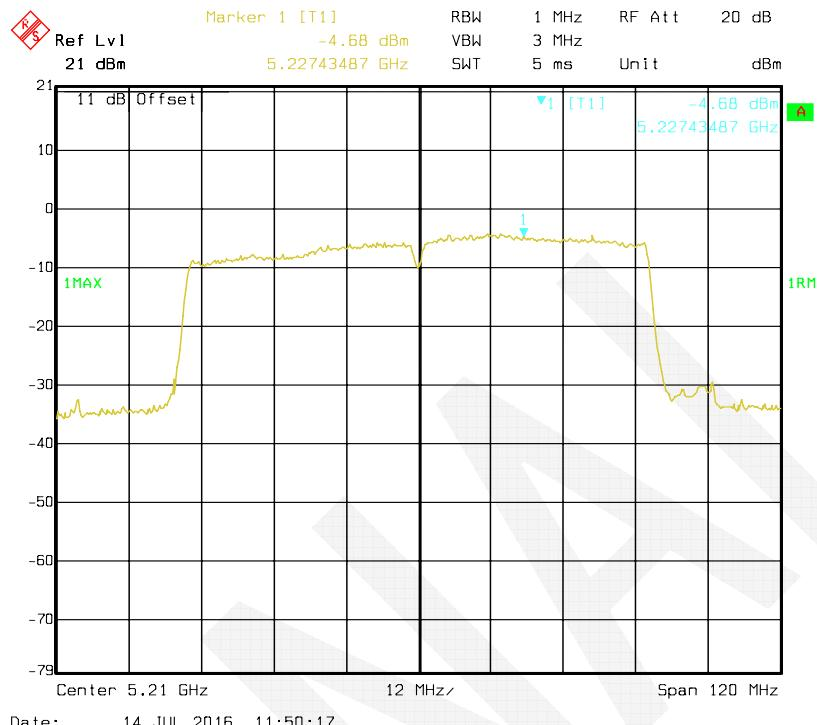
**802.11a mode, Antenna 2: Power Spectral Density-5180 MHz**
