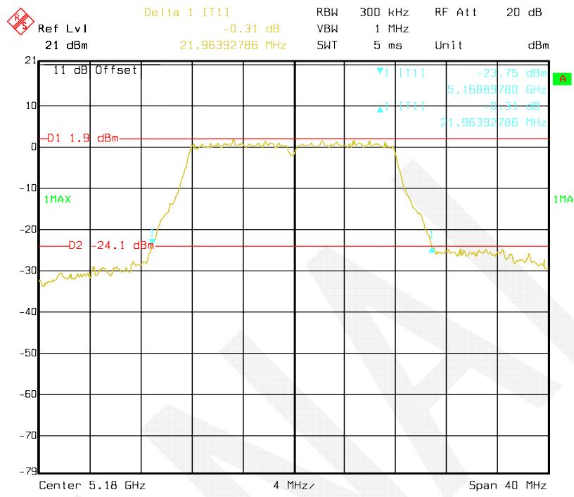
**802.11a mode, Antenna 1: 26 dB Bandwidth-5220 MHz**
