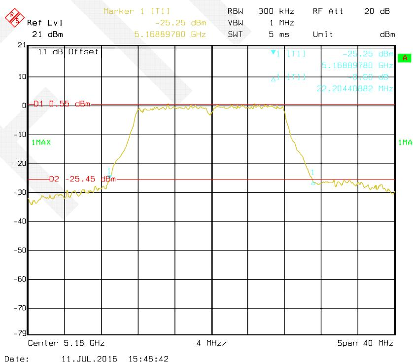
**802.11a mode, Antenna 2: 26 dB Bandwidth-5220 MHz**
