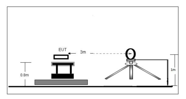
(B) Radiated Emission Test-Up Frequency 30MHz~1GHz
