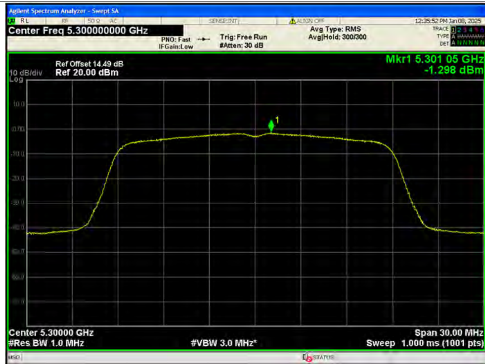
PSD NVNT ac20 5320MHz Ant0 SISO
