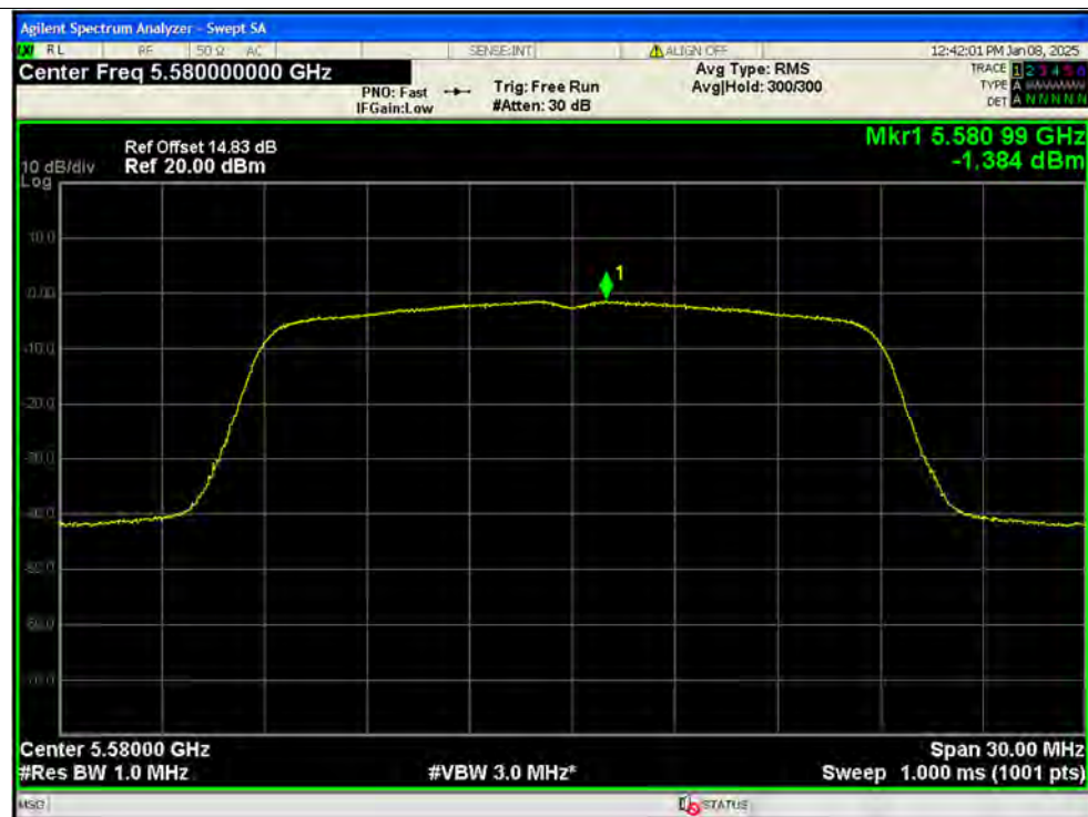
PSD NVNT ac20 5580MHz Ant0 SISO
