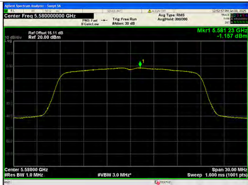
PSD NVNT ac20 5580MHz Ant1 SISO
