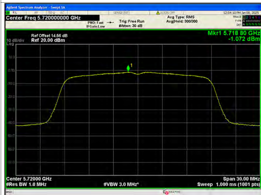
PSD NVNT ac20 5745MHz Ant1 SISO
