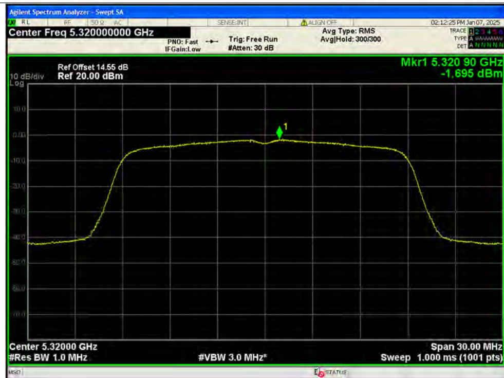
PSD NVNT ac20 5320MHz Ant1 MIMO
