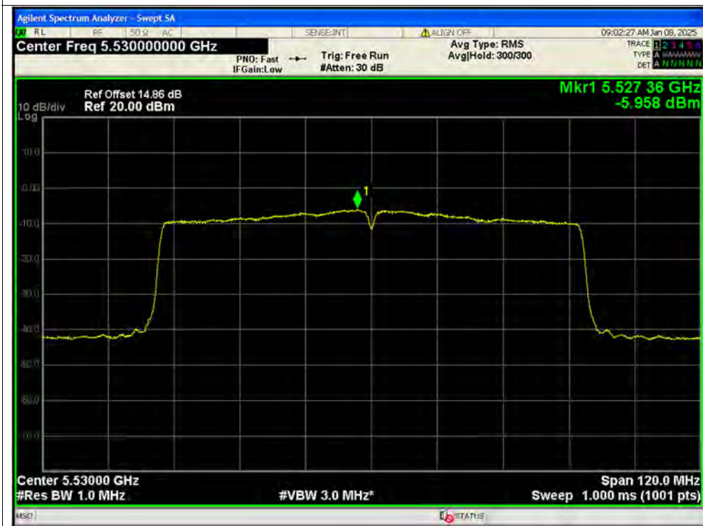
PSD NVNT ac80 5530MHz Ant1 SISO
