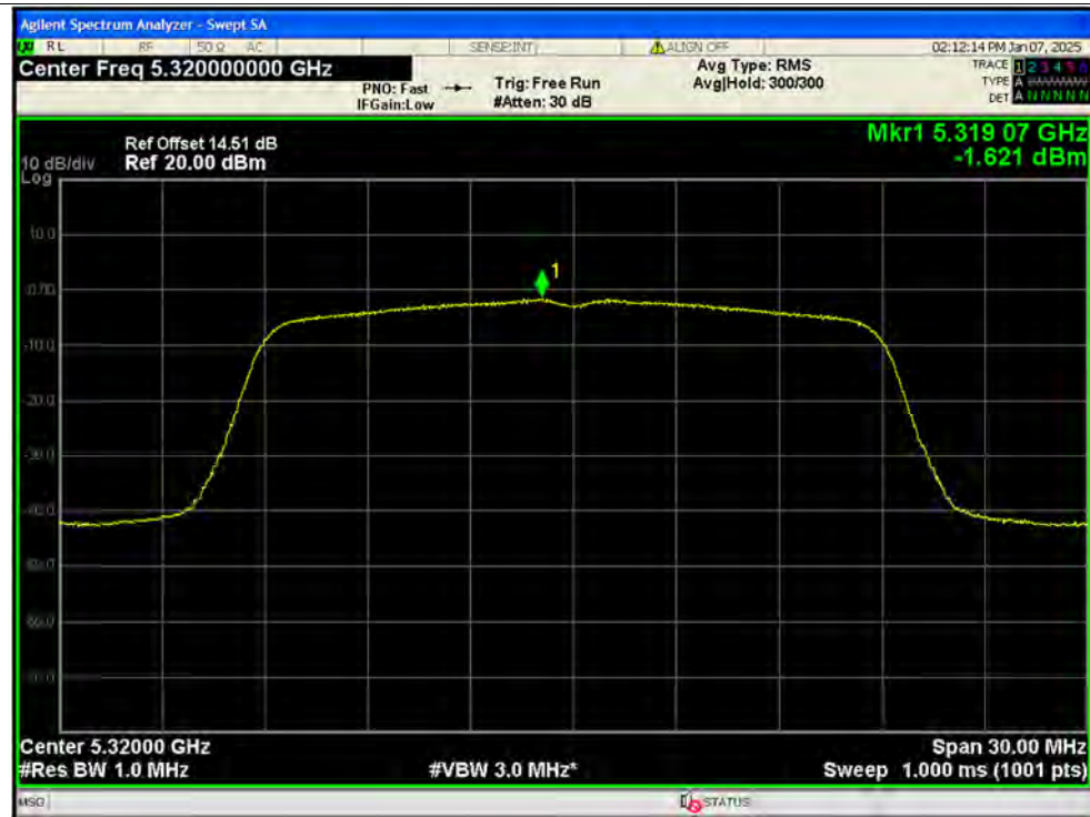
PSD NVNT ac20 5320MHz Ant1 MIMO
