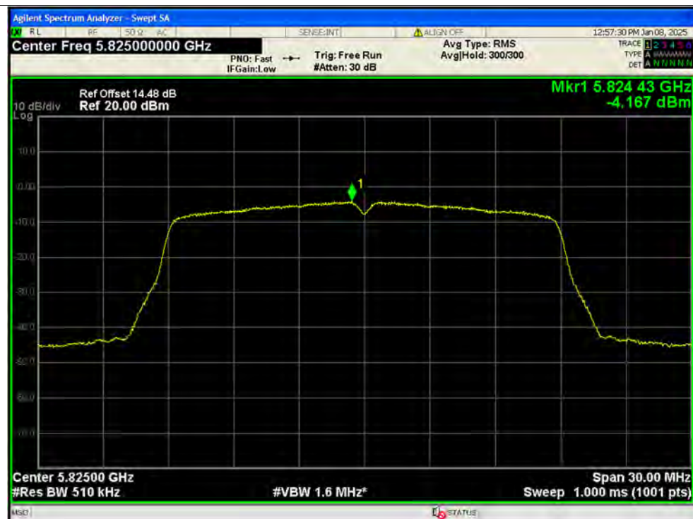
PSD NVNT ac20 5825MHz Ant1 SISO
