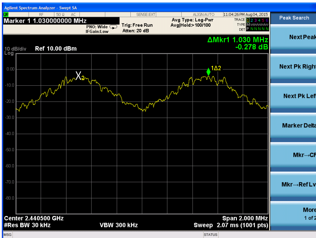
Fig 23. Carrier Frequency Separation in Middle channel, 1Mbps
