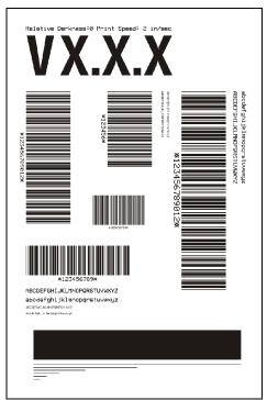
**3.** Inspect the labels and determine which one has the best darkness setting for your application. This value can be entered into the printer by setting the darkness during the configuration procedure.
