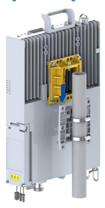
4. Tighten the captive screw on the RRU support with an M6 inner-hexagon wrench to fix the ZXSDR R8854, see Figure 4-31.
