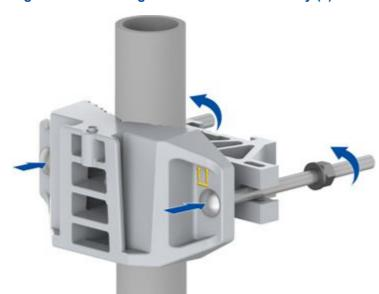
Figure 4-18 Installing the Pole Mount Assembly (2)
