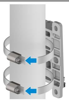
c. Tighten the screws on the pole hoops.
