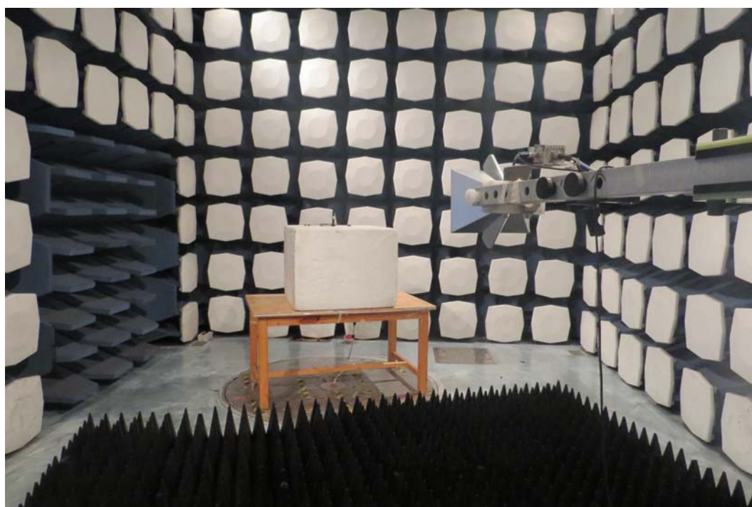
Picture 2: Radiated Spurious Emissions Test setup
