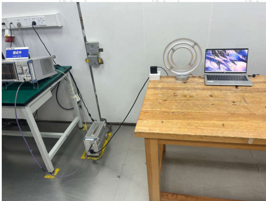
Conducted Emissions Test Setup-1
