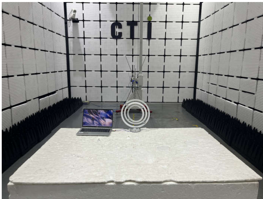
Radiated spurious emission Test Setup-1 (Below 1GHz)
