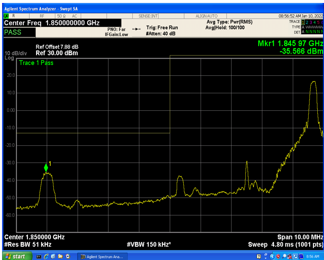
Band2 QAM16 BW=5MHz Channel=18625 RB Size=25 Position=#0
