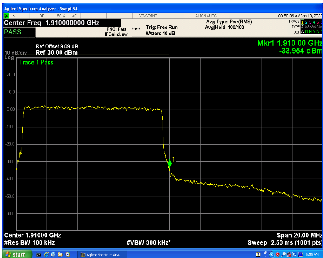
Band2 QPSK BW=15MHz Channel=18675 RB Size=1 Position=#0
