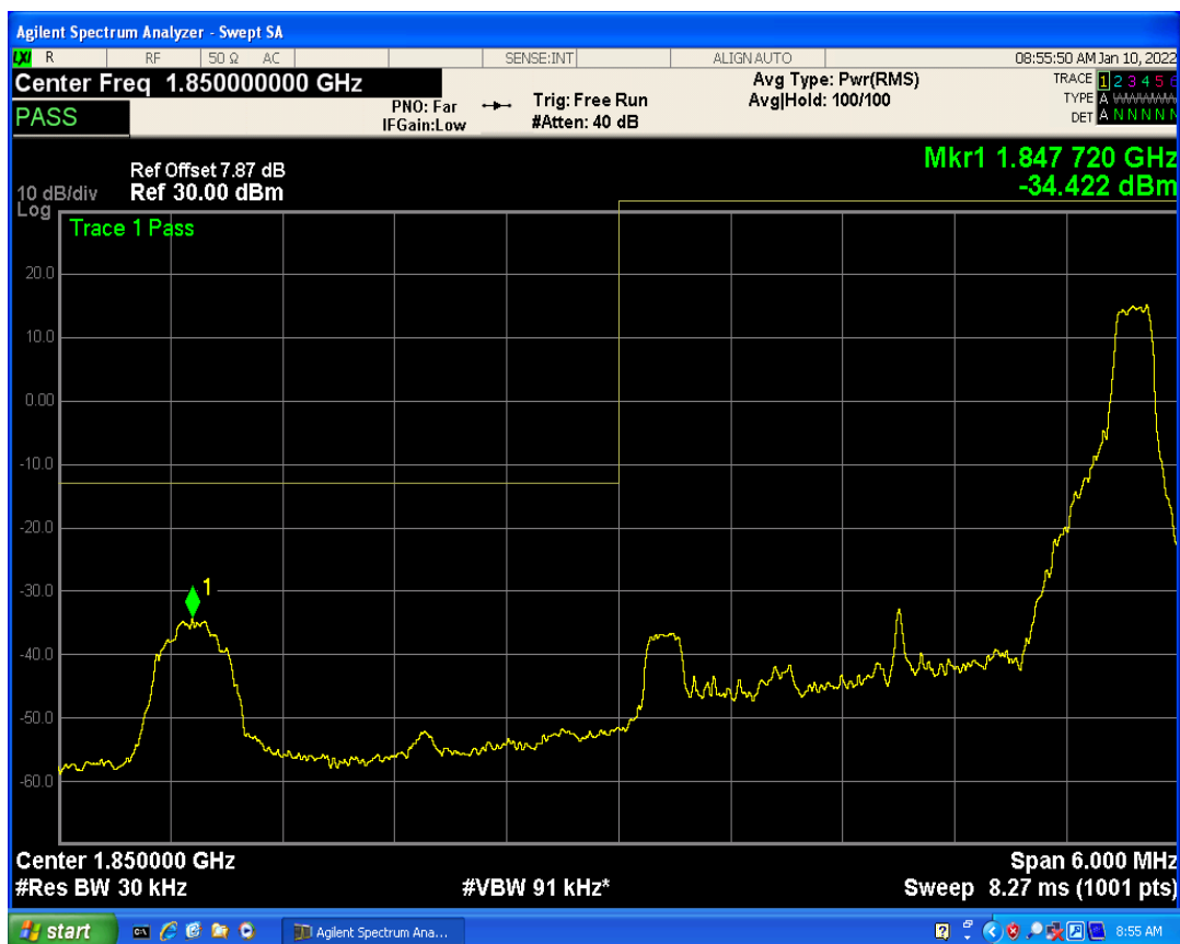
Band2 QAM16 BW=3MHz Channel=18615 RB Size=1 Position=#0
