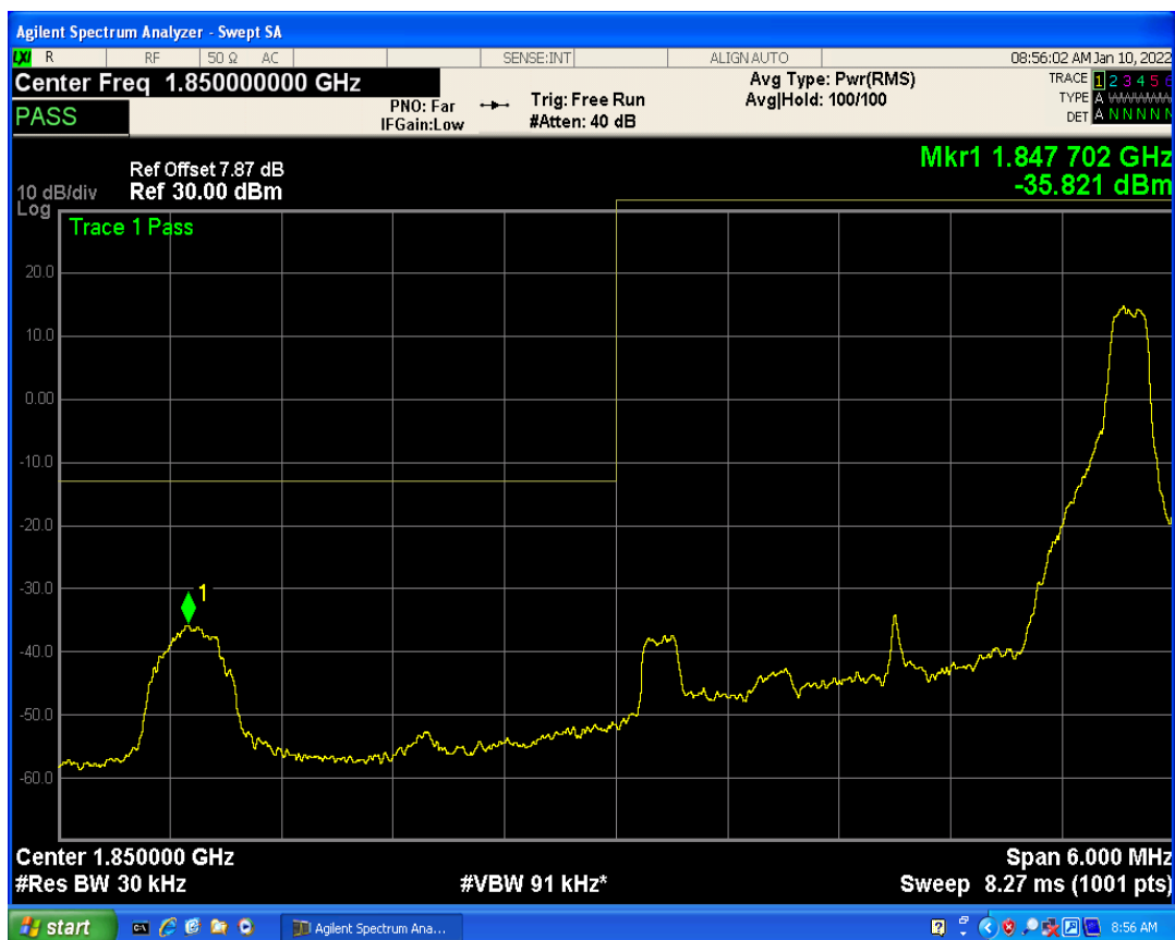
Band2 QPSK BW=3MHz Channel=19185 RB Size=1 Position=#0
