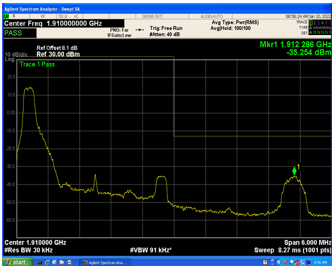
Band2 QPSK BW=3MHz Channel=19185 RB Size=15 Position=#0
