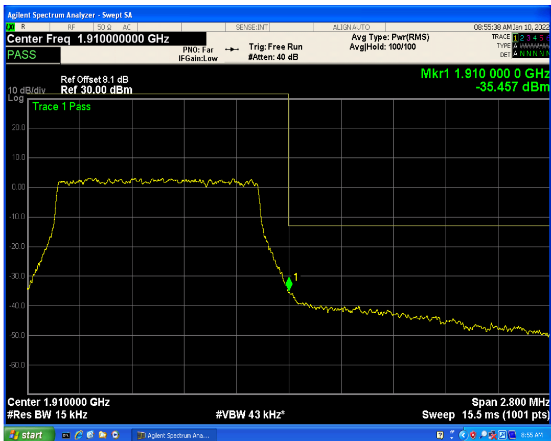
Band2 QPSK BW=3MHz Channel=18615 RB Size=1 Position=#Max
