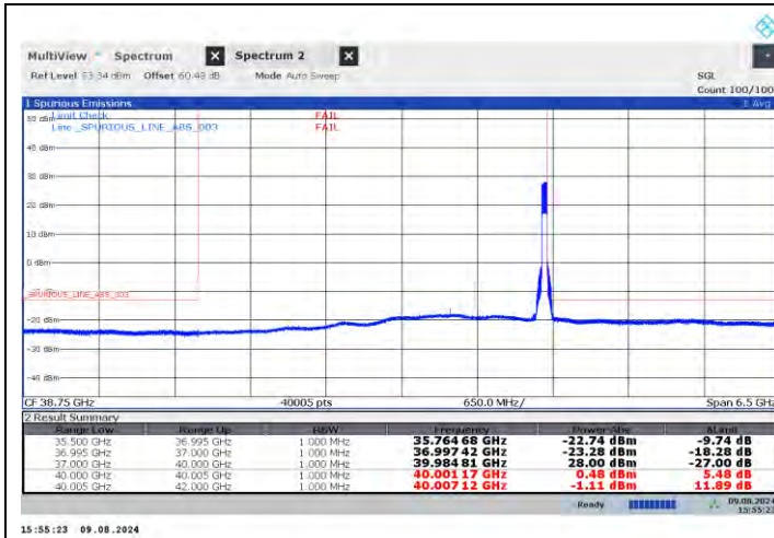
n260 50MHz-16QAM- High -H-1RB31
