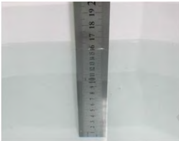
Liquid Height for Head SAR
