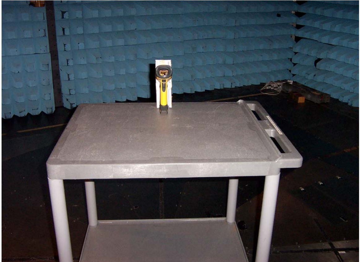
Spurious Radiated Emissions Set Up Photograph
