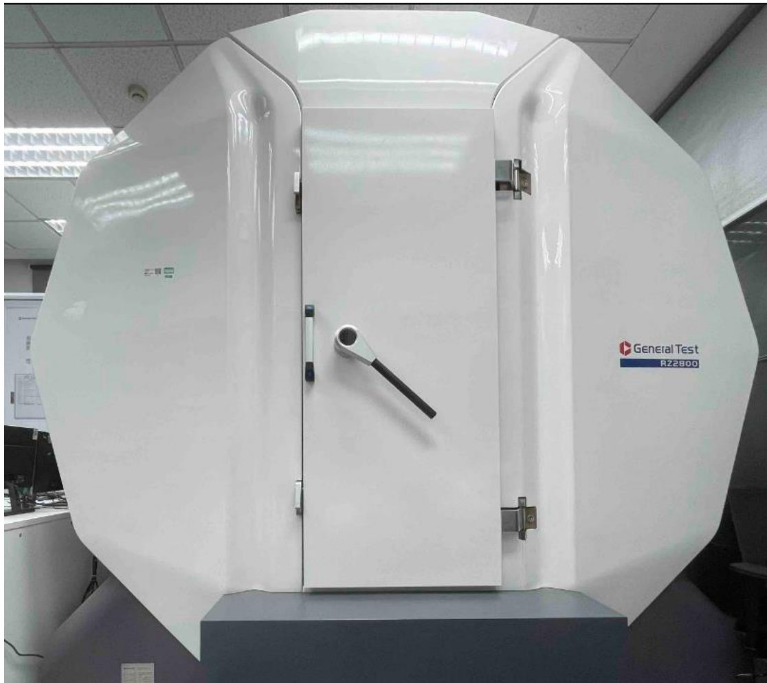
Fig. 5. The fully anechoic chamber
