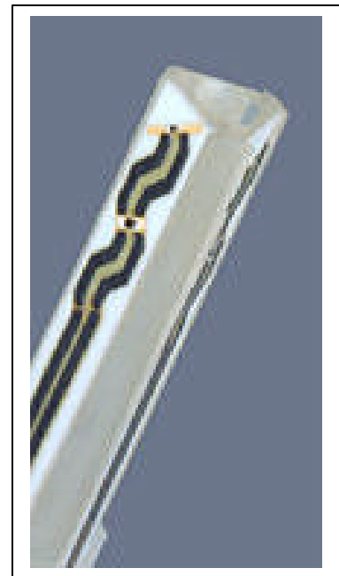
Inside view of ET3DV6 E-field Probe
