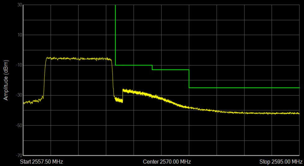
Band7 16QAM BW=10MHz Channel=21400 RB Size=50 Position=#0
