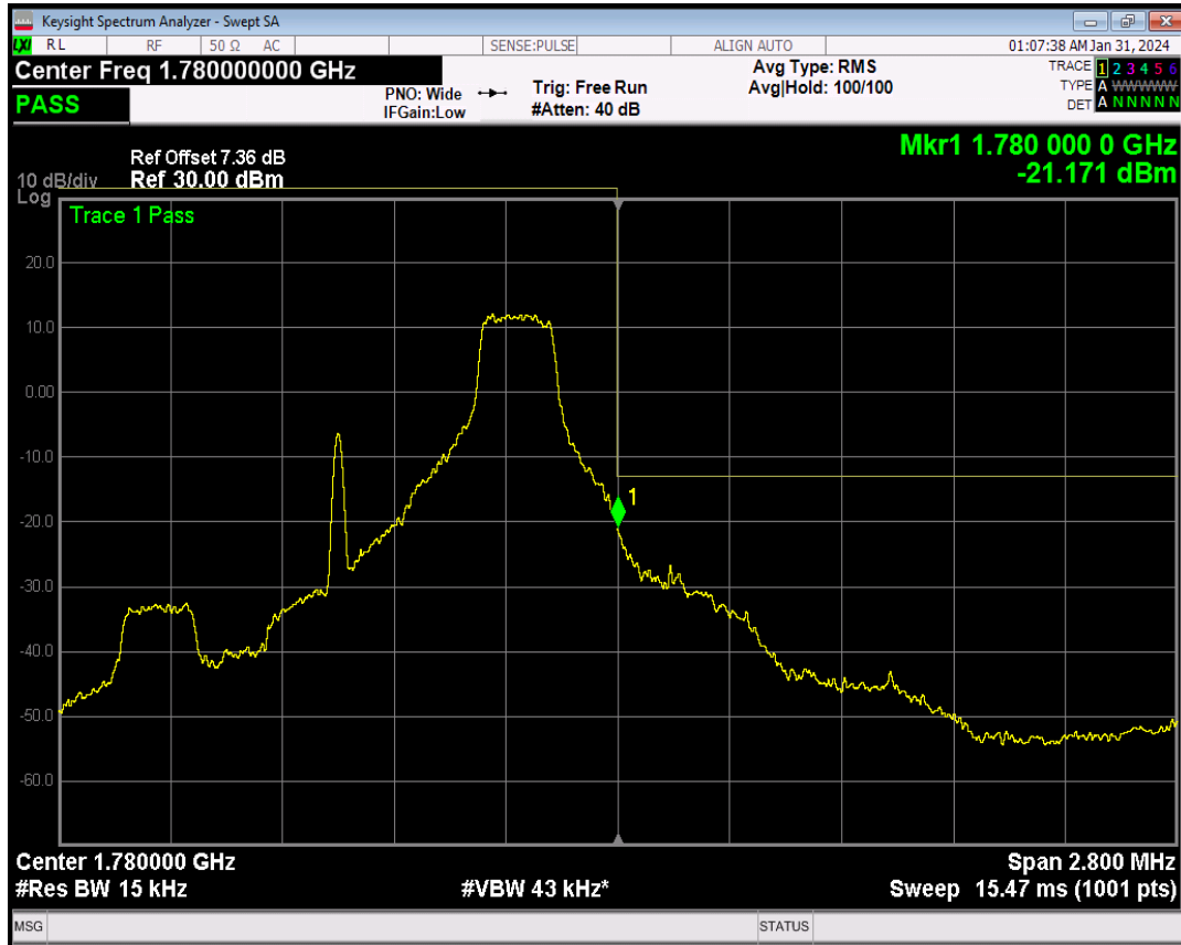
Band66 16QAM BW=1.4MHz Channel=132665 RB Size=6 Position=#0
