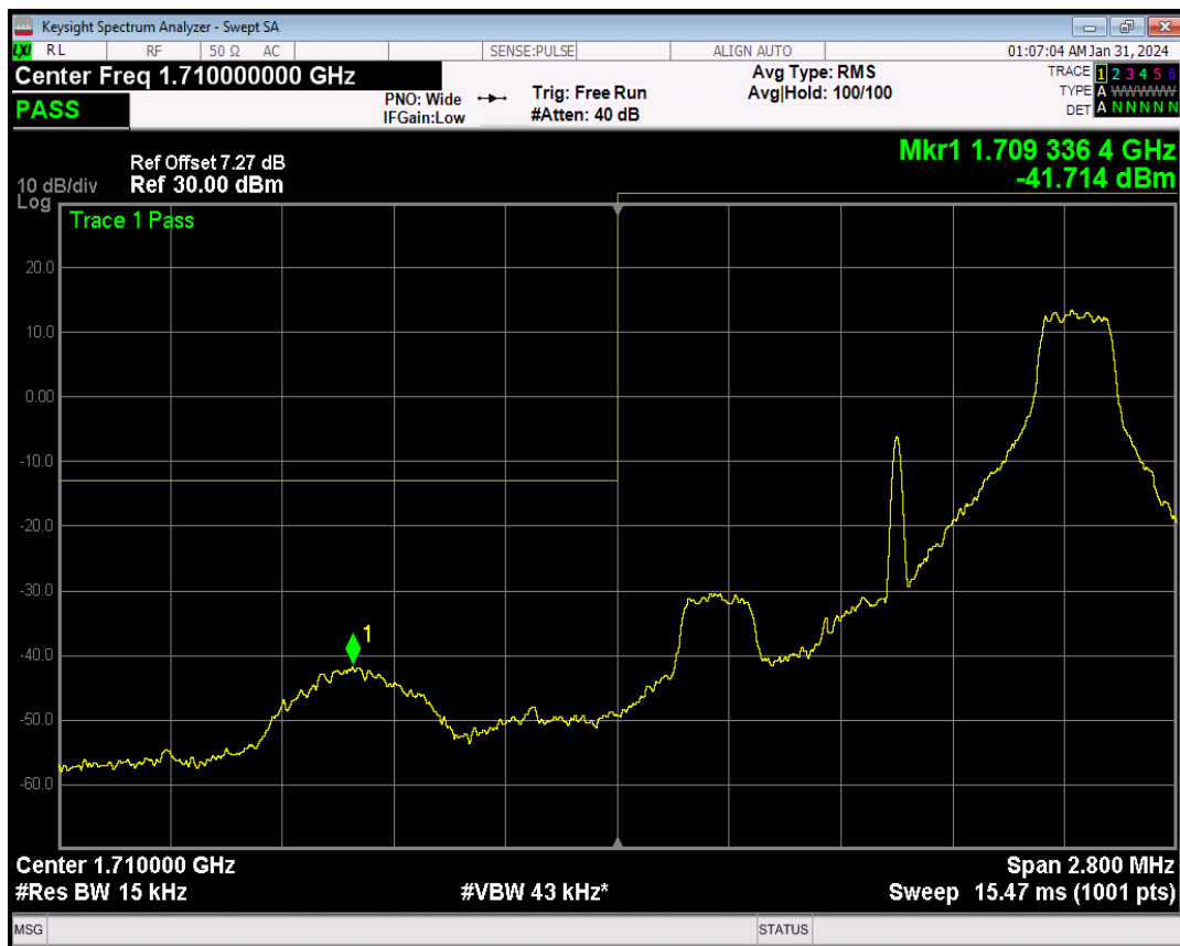
Band66 QPSK BW=1.4MHz Channel=131979 RB Size=6 Position=#0
