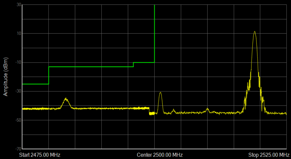
Band7 QPSK BW=20MHz Channel=20850 RB Size=1 Position=#Max
