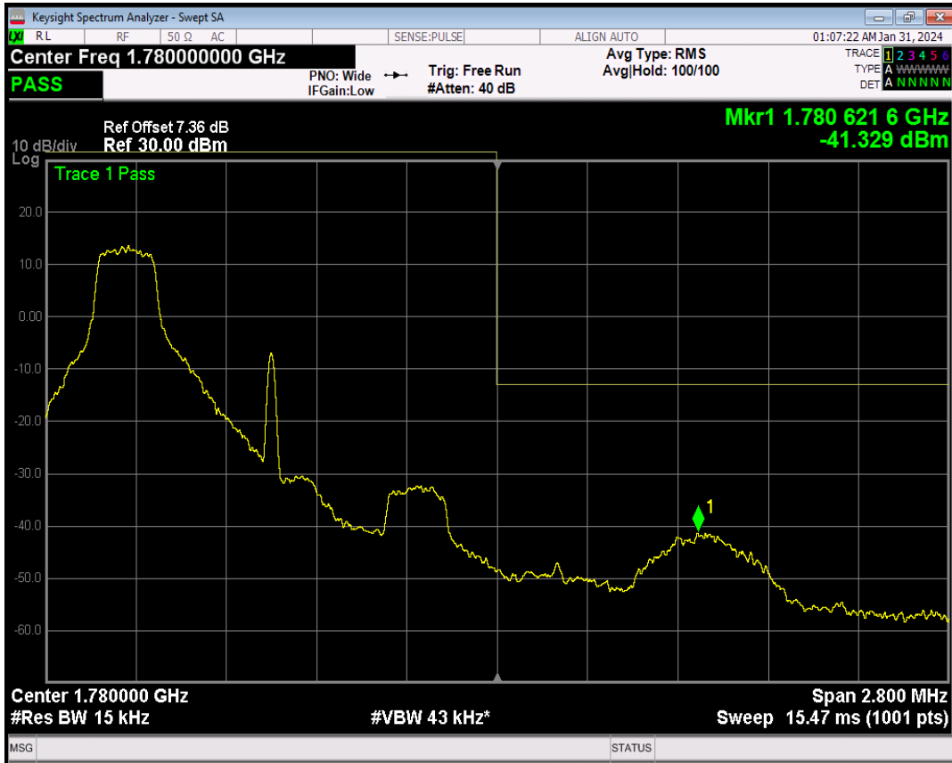
Band66 QPSK BW=1.4MHz Channel=132665 RB Size=1 Position=#Max
