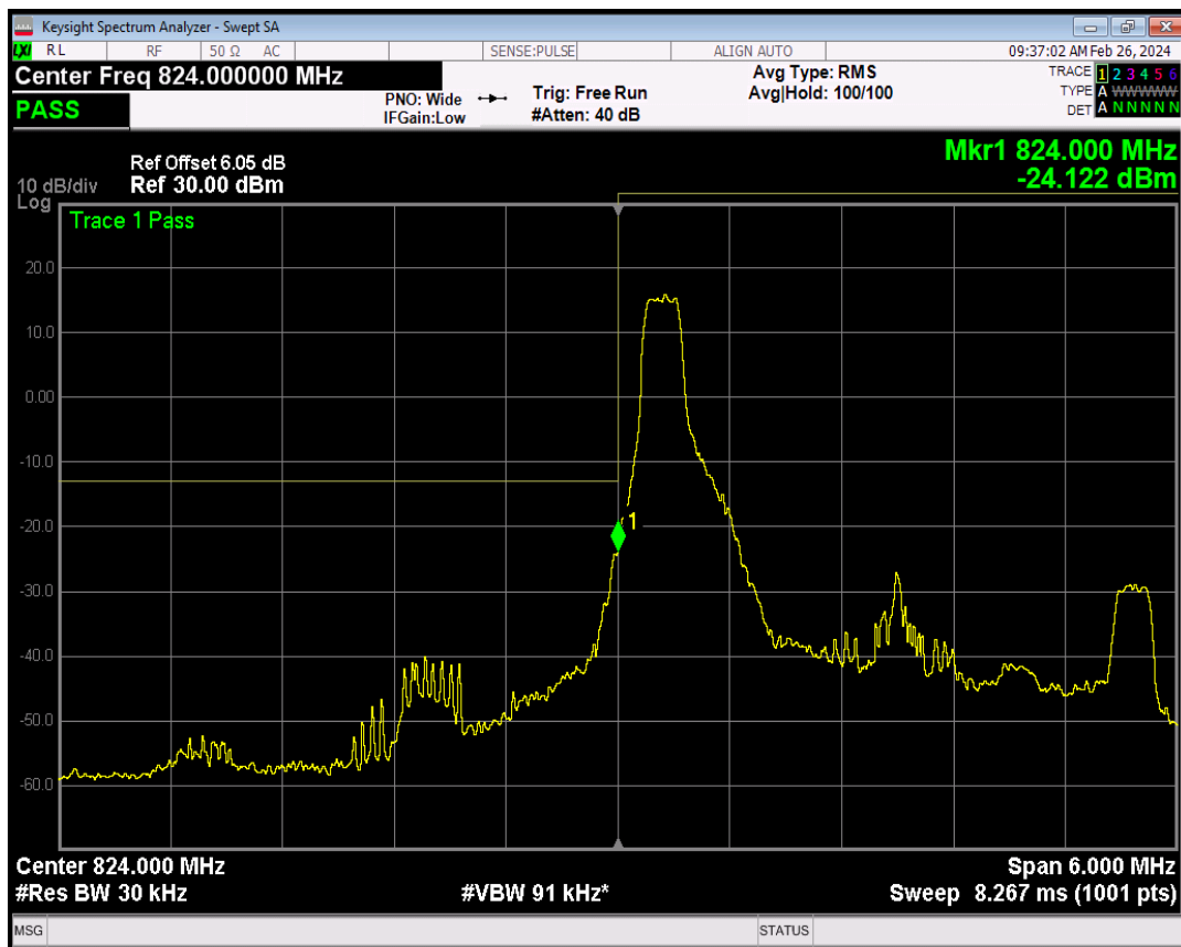
Band5 16QAM BW=3MHz Channel=20415 RB Size=1 Position=#Max
