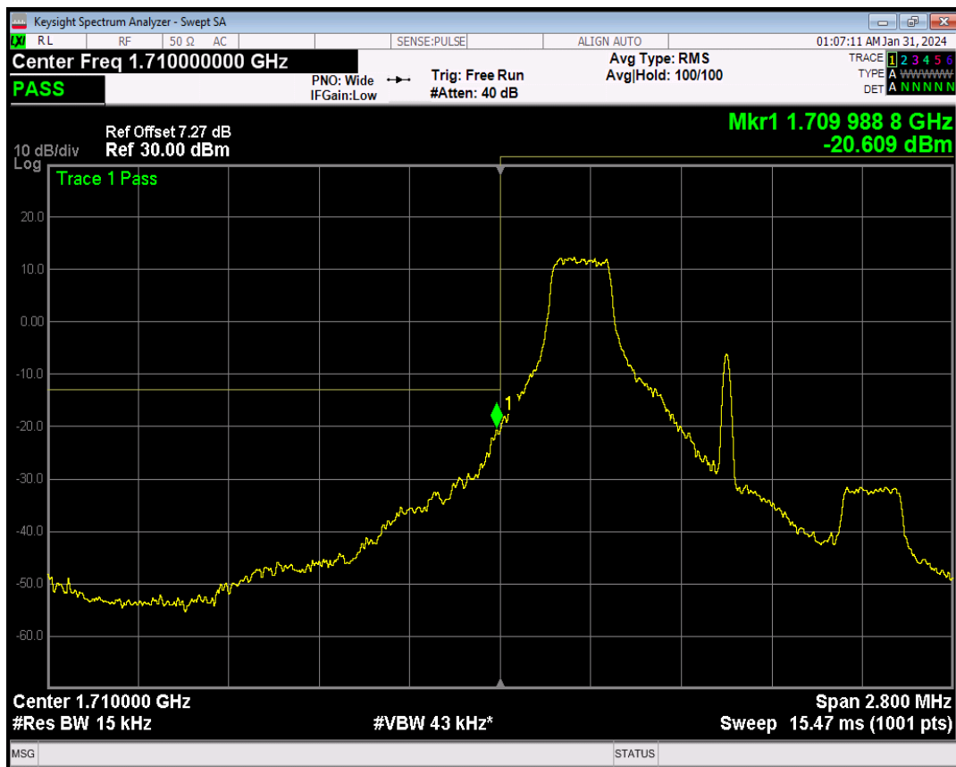
Band66 16QAM BW=1.4MHz Channel=131979 RB Size=1 Position=#Max
