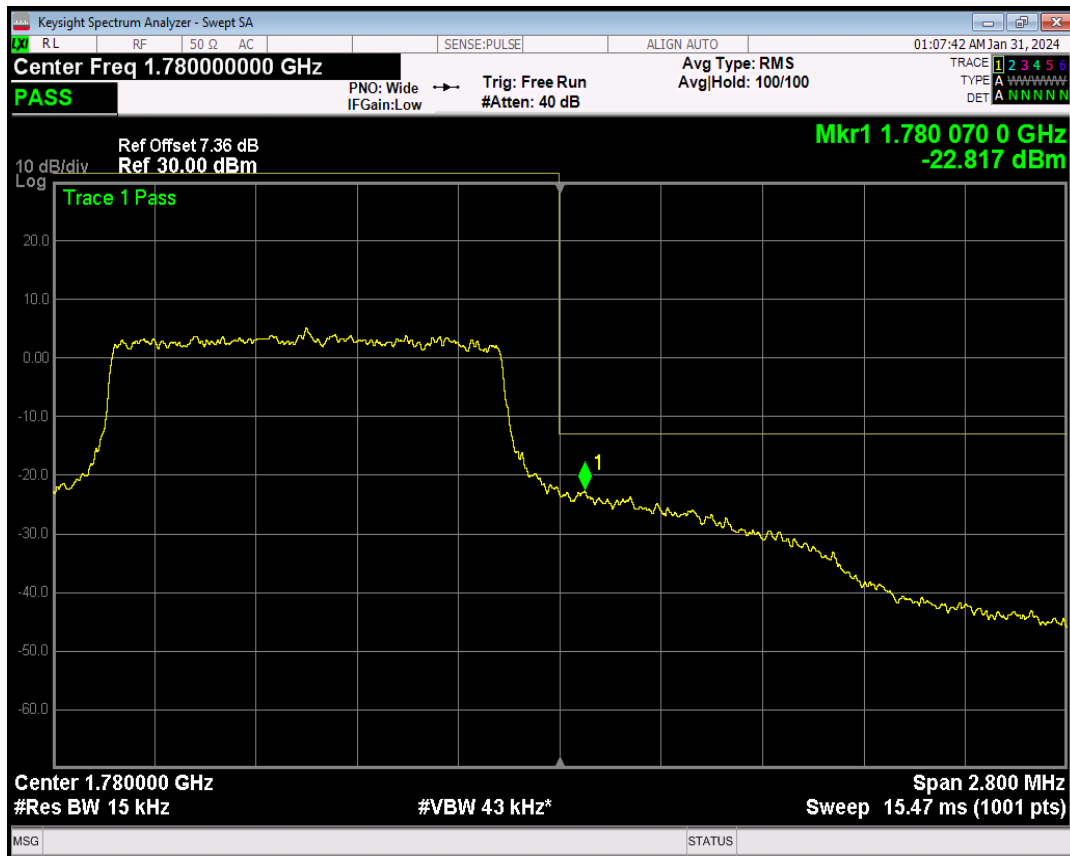
Band66 QPSK BW=3MHz Channel=131987 RB Size=1 Position=#0
