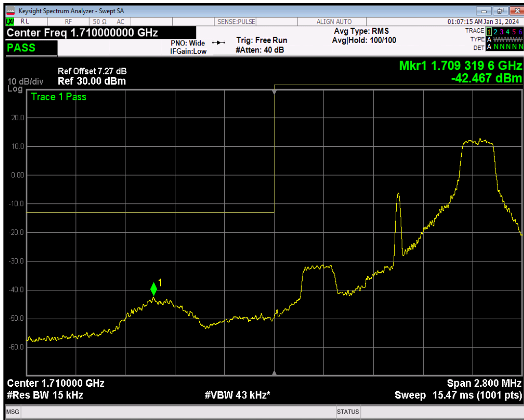
Band66 16QAM BW=1.4MHz Channel=131979 RB Size=6 Position=#0
