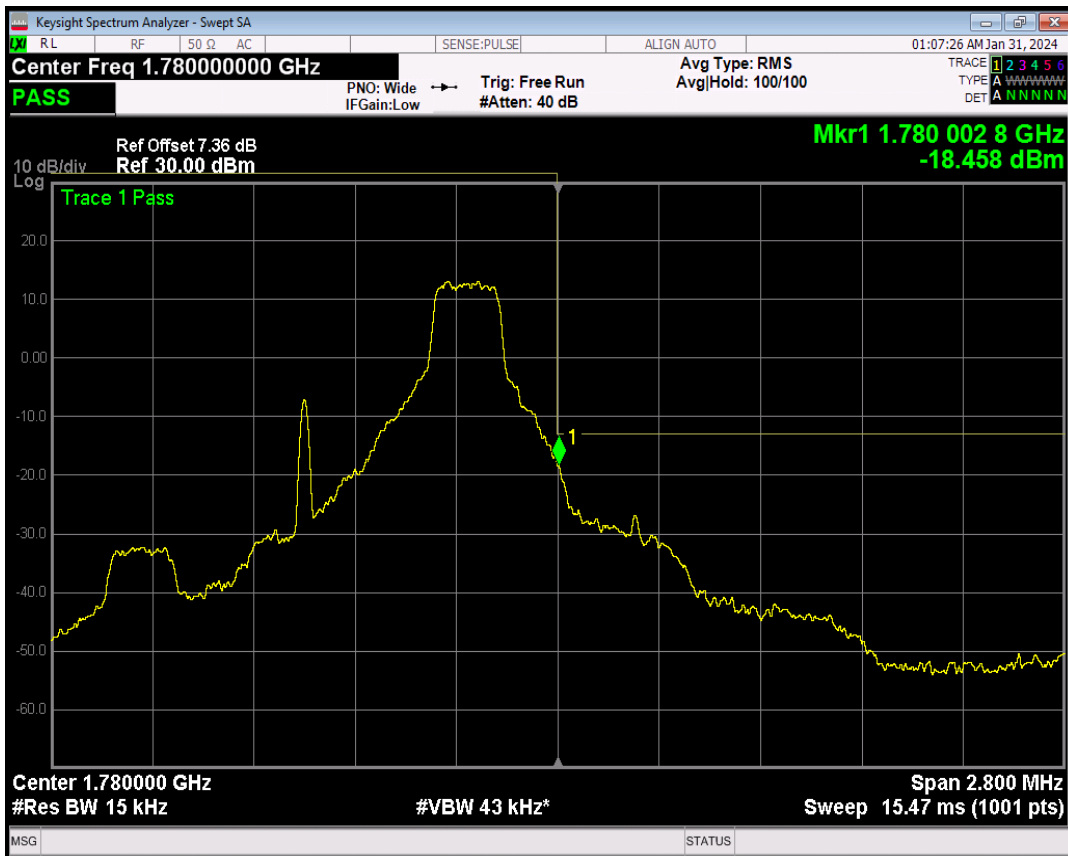
Band66 QPSK BW=1.4MHz Channel=132665 RB Size=6 Position=#0
