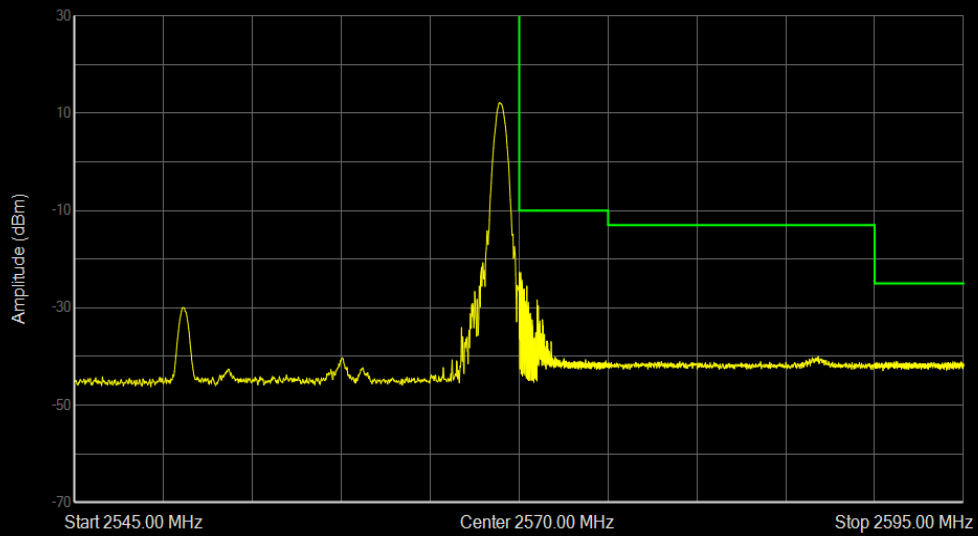
Band7 QPSK BW=20MHz Channel=21350 RB Size=1 Position=#Max
