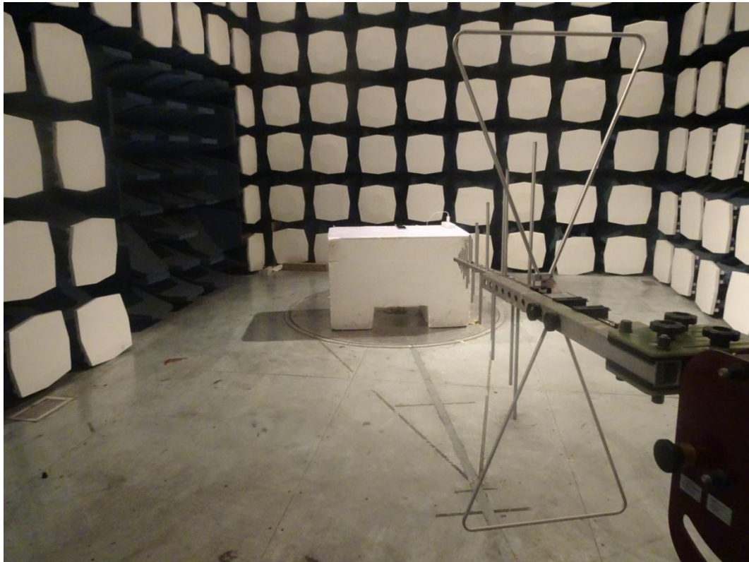
Picture 1: Radiated Emission Test Setup
