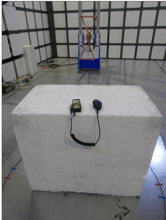
**Figure 1 - 30 MHz to 1 GHz - X Orientation**
