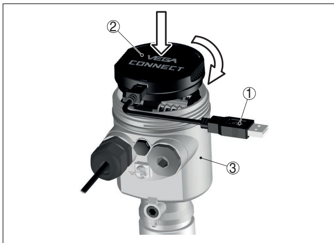
Fig. 38: Connection of the PC directly to the sensor via the interface adapter
