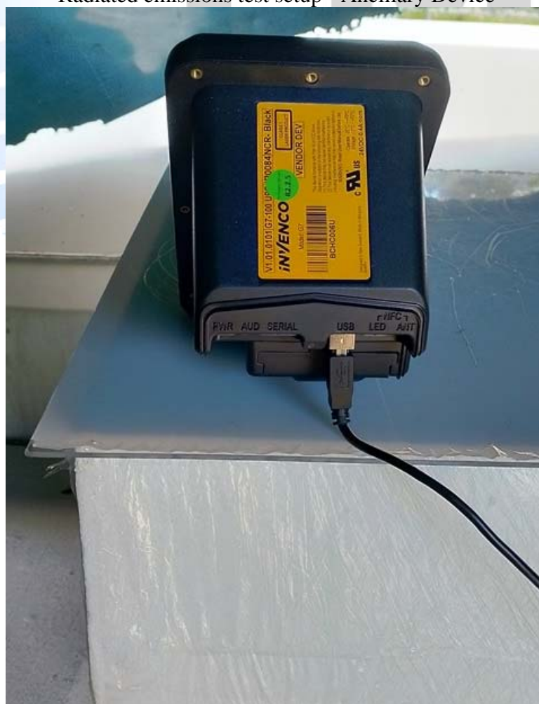
Radiated emissions test setup - Ancillary Device
