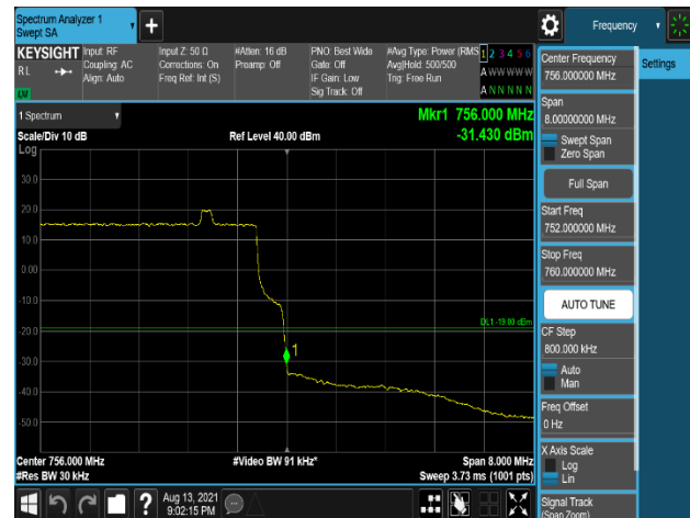
Plot 7-318. Band Edge Emission (756MHz to 757MHz) Plot (LTE_B13_10M+Low_NB-lot(IB)+High_NB-lot(IB)_1C – Port 3)
