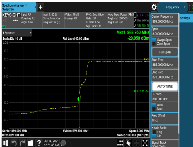
Plot 7-307. Band Edge Emission (868MHz to 869MHz) Plot (LTE_B5_10M+10M_2C_64QAM - Non-contiguous, Port 1)
