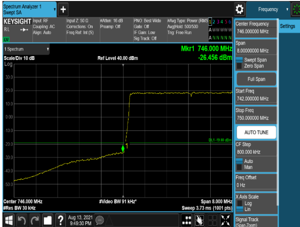
Plot 7-309. Band Edge Emission (745MHz to 746MHz) Plot (LTE_B5_5M_1C_64QAM - Low Channel, Port 1)
