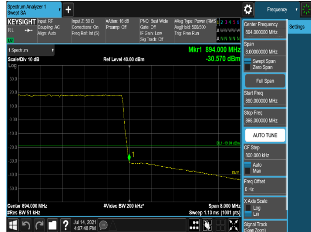
Plot 7-306. Band Edge Emission (894MHz to 895MHz) Plot (LTE_B5_5M+5M_2C_64QAM - Non-contiguous, Port 2)
