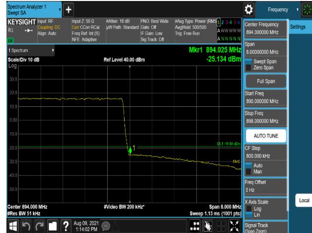
Plot 7-338. Band Edge Emission (894MHz to 895MHz) Plot (DSS_B5_10M+5M_2C_QPSK - High Channel, Port 2)
