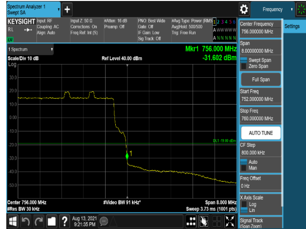
Plot 7-322. Band Edge Emission (756MHz to 757MHz) Plot (LTE_B13_10M+High_NB-lot(IB)+High_NB-lot(IB)_1C – Port 3)
