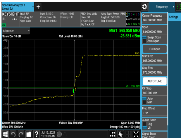
Plot 7-297. Band Edge Emission (868MHz to 869MHz) Plot (LTE_B5_10M_1C_QPSK - Low Channel, Port 0)
