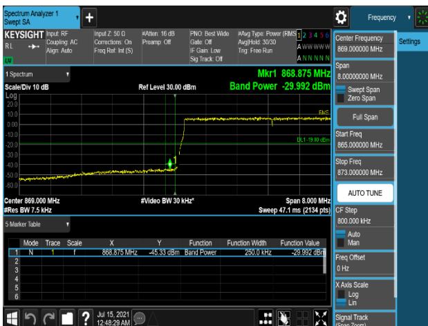
Plot 7-303. Band Edge Emission (868MHz to 869MHz) Integration method Plot (B2 5M+10M+10M 3C QPSK - Low Channel, Port 0)
