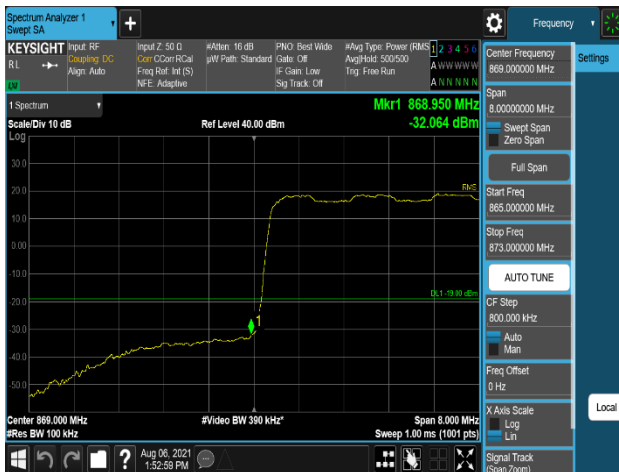
Plot 7-339. Band Edge Emission (868MHz to 869MHz) Plot (DSS_B5_10M+10M_2C_16QAM - Low Channel, Port 0)
