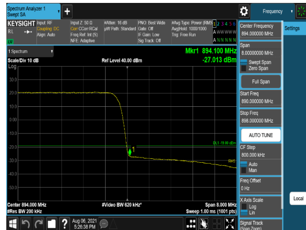
Plot 7-334. Band Edge Emission (894MHz to 895MHz) Plot (DSS_B5_10M+10M_2C_64QAM - High Channel, Port 0)
