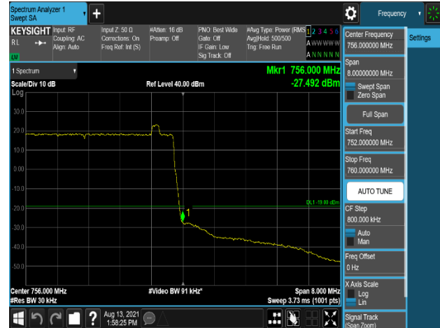
Plot 7-316. Band Edge Emission (756MHz to 757MHz) Plot (LTE_B13_5M+NB-lot(IB)_1C – Port 0)
