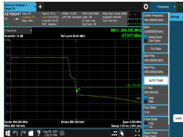
Plot 7-340. Band Edge Emission (894MHz to 895MHz) Plot (DSS_B5_10M+10M_2C_64QAM - High Channel, Port 2)
