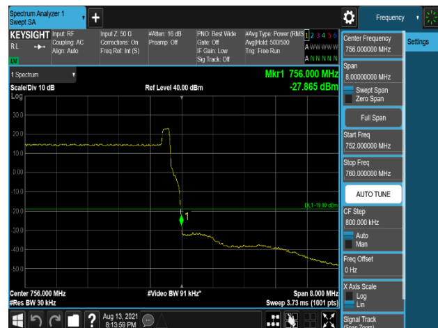
Plot 7-328. Band Edge Emission (756MHz to 757MHz) Plot (LTE_B13_10M+High_NB-lot(GB)+Low_NB-lot(IB)_2C – Port 2)
