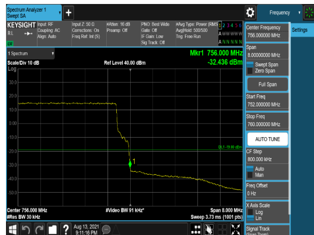
Plot 7-320. Band Edge Emission (756MHz to 757MHz) Plot (LTE_B13_10M+Low_NB-lot(IB)+Low_NB-lot(IB)_1C – Port 3)
