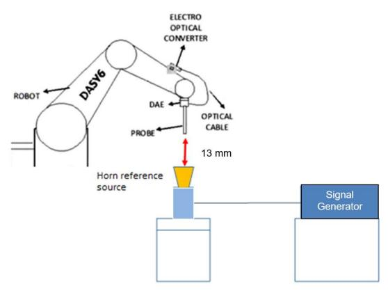
The output power on the reference source is set to 10.0 dBm (10 mW) and the measurement results E, H and Avg PD are compared with the Numerical modeling.
