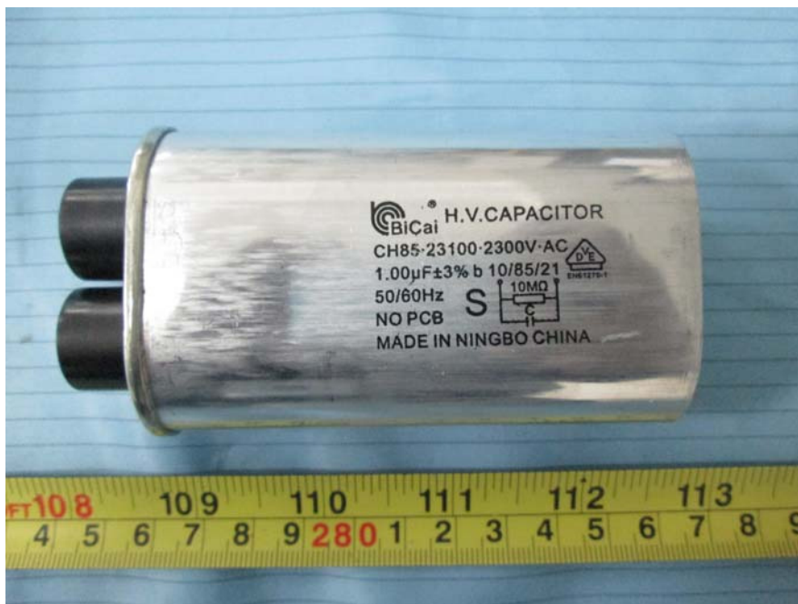
EUT – H.V. Capacitor View
