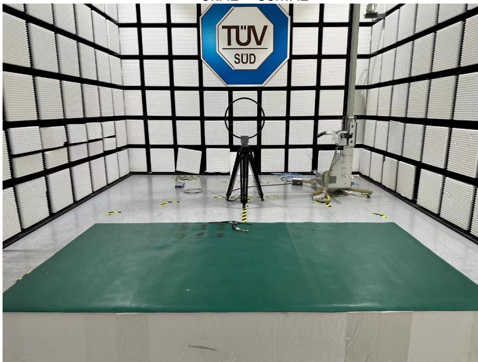
Radiated Emission Setup 9kHz ~ 30MHz
