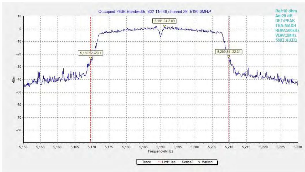
Fig.21 Occupied 26dB Bandwidth (802.11n-HT40, 5190MHz)
