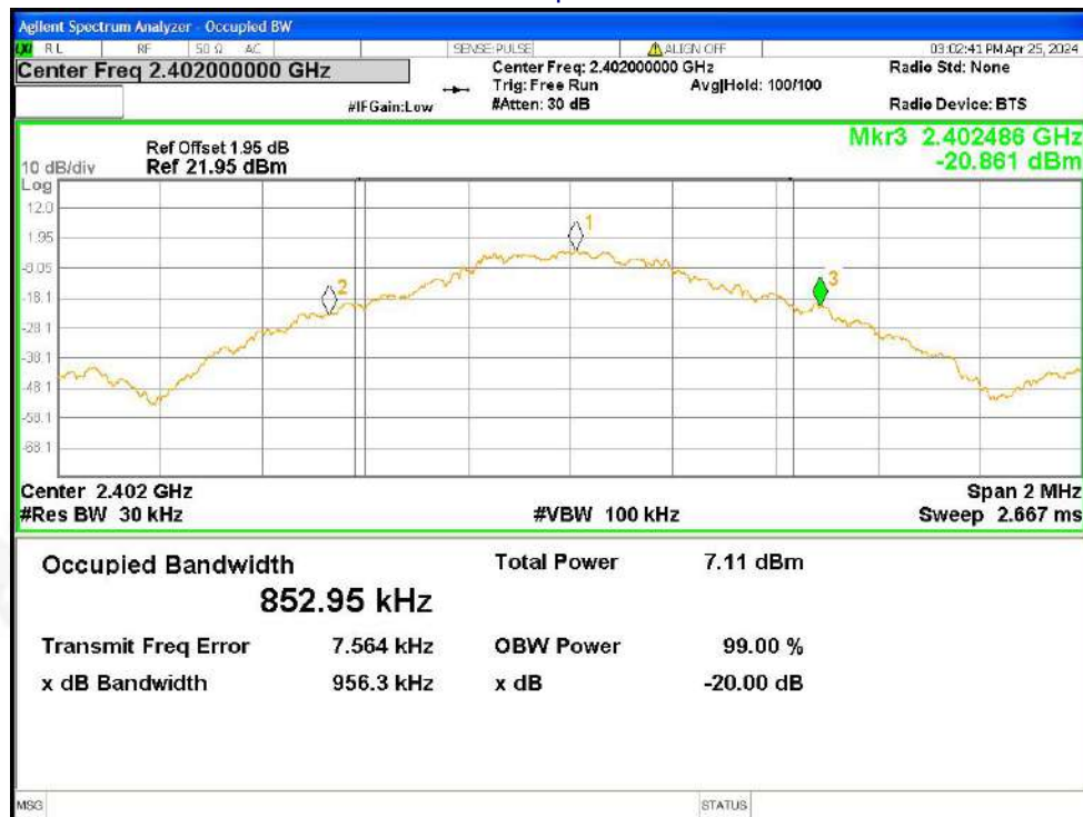
-20dB Bandwidth NVNT 1-DH5 2402MHz Ant1
