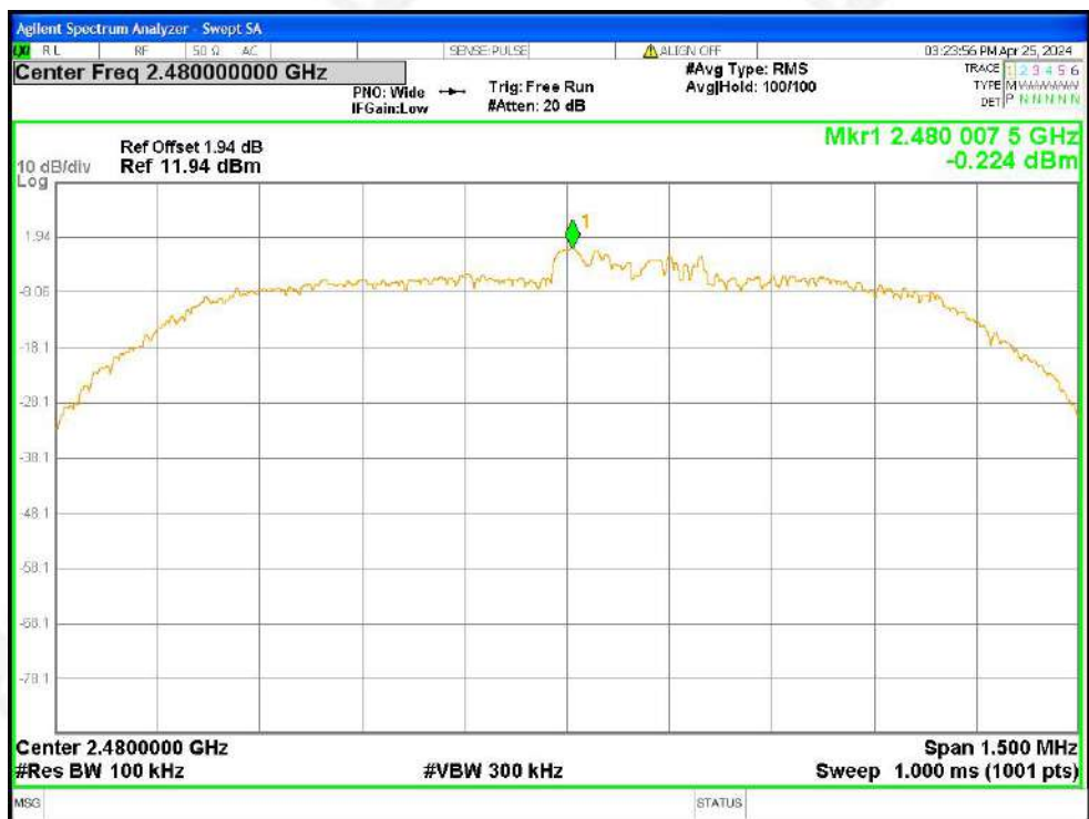
Tx. Spurious NVNT 2-DH5 2480MHz Ant1 Ref
