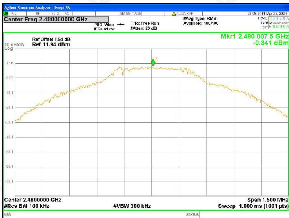
Tx. Spurious NVNT 1-DH5 2480MHz Ant1 Ref
