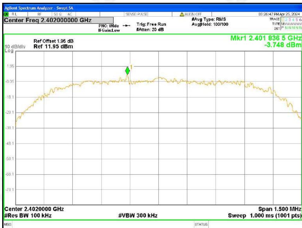
Tx. Spurious NVNT 3-DH5 2402MHz Ant1 Ref
