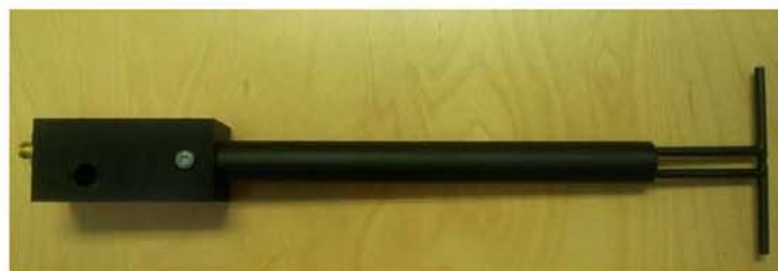
Figure 1 – MVG COMOSAR Validation Dipole
