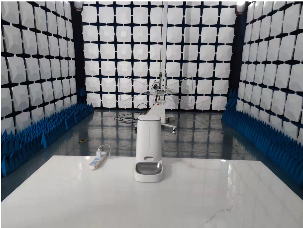
Below 1GHz for radiated emission test setup
