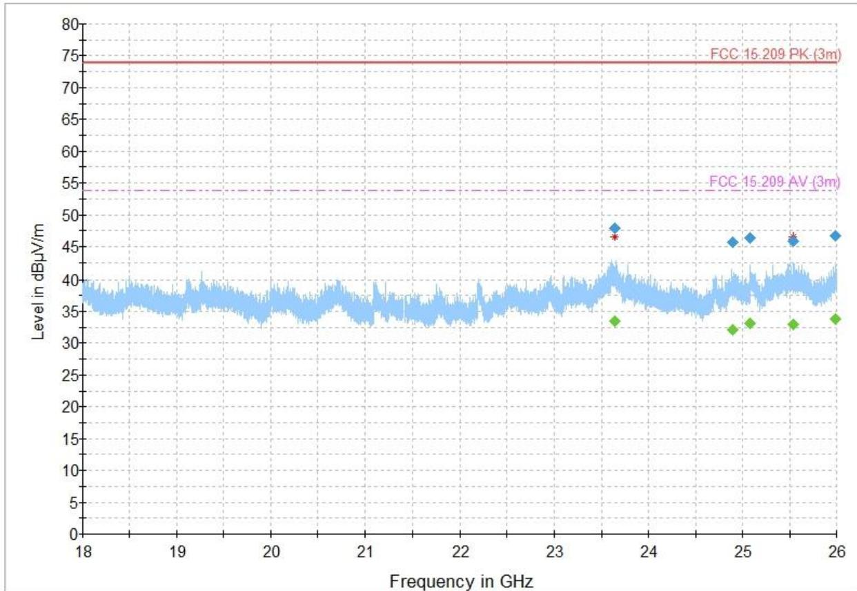
Figure 8.6-8: Radiated emissions, 2440 MHz, 18 - 26 GHz
