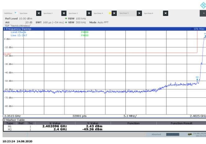
Figure 8.4-1: Conducted band edge measurement, 2402 MHz
