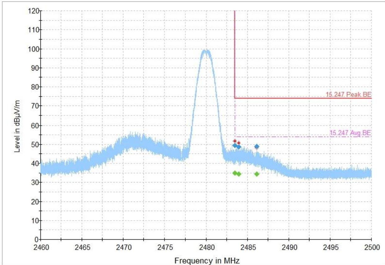
Figure 8.6-2: Radiated emissions, restricted band edge, high
