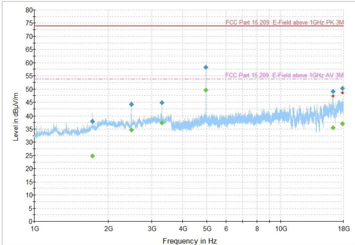
Figure 8.6-10: Radiated emissions, 2480 MHz, 1 - 18 GHz
