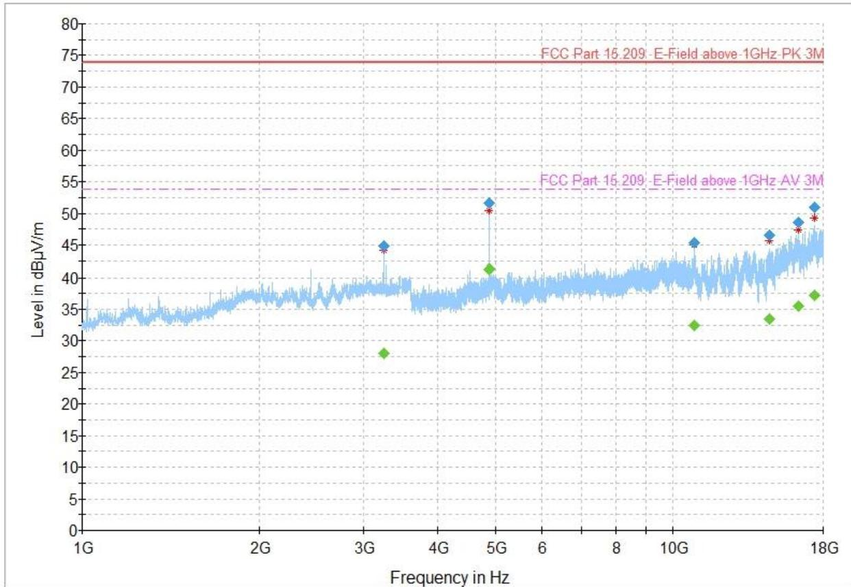
Figure 8.6-7: Radiated emissions, 2440 MHz, 1 - 18 GHz
