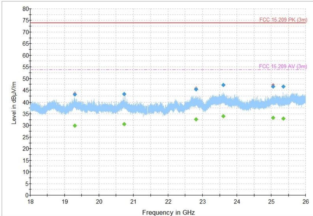
Figure 8.6-5: Radiated emissions, 2402 MHz, 18 - 26 GHz
