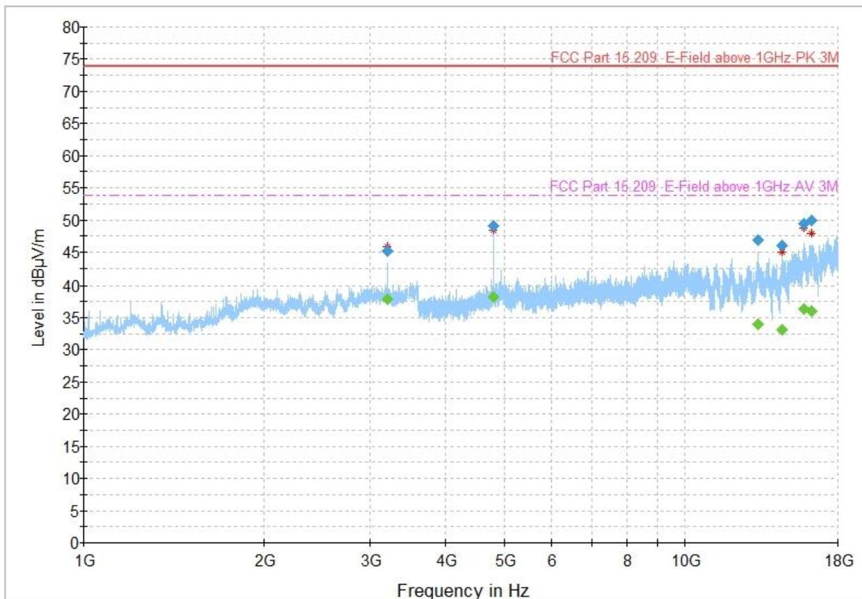
Figure 8.6-4: Radiated emissions, 2402 MHz, 1 - 18 GHz
