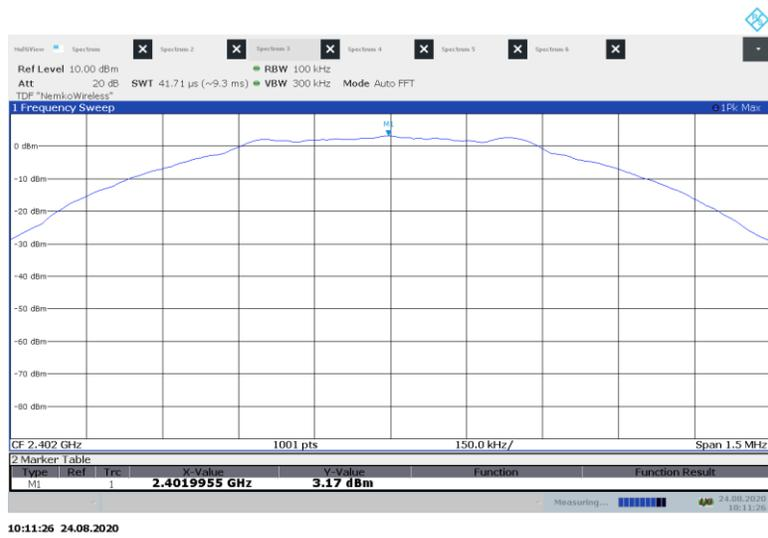
Figure 8.7-1: Power spectral density of digital transmission system, 2402 MHz
