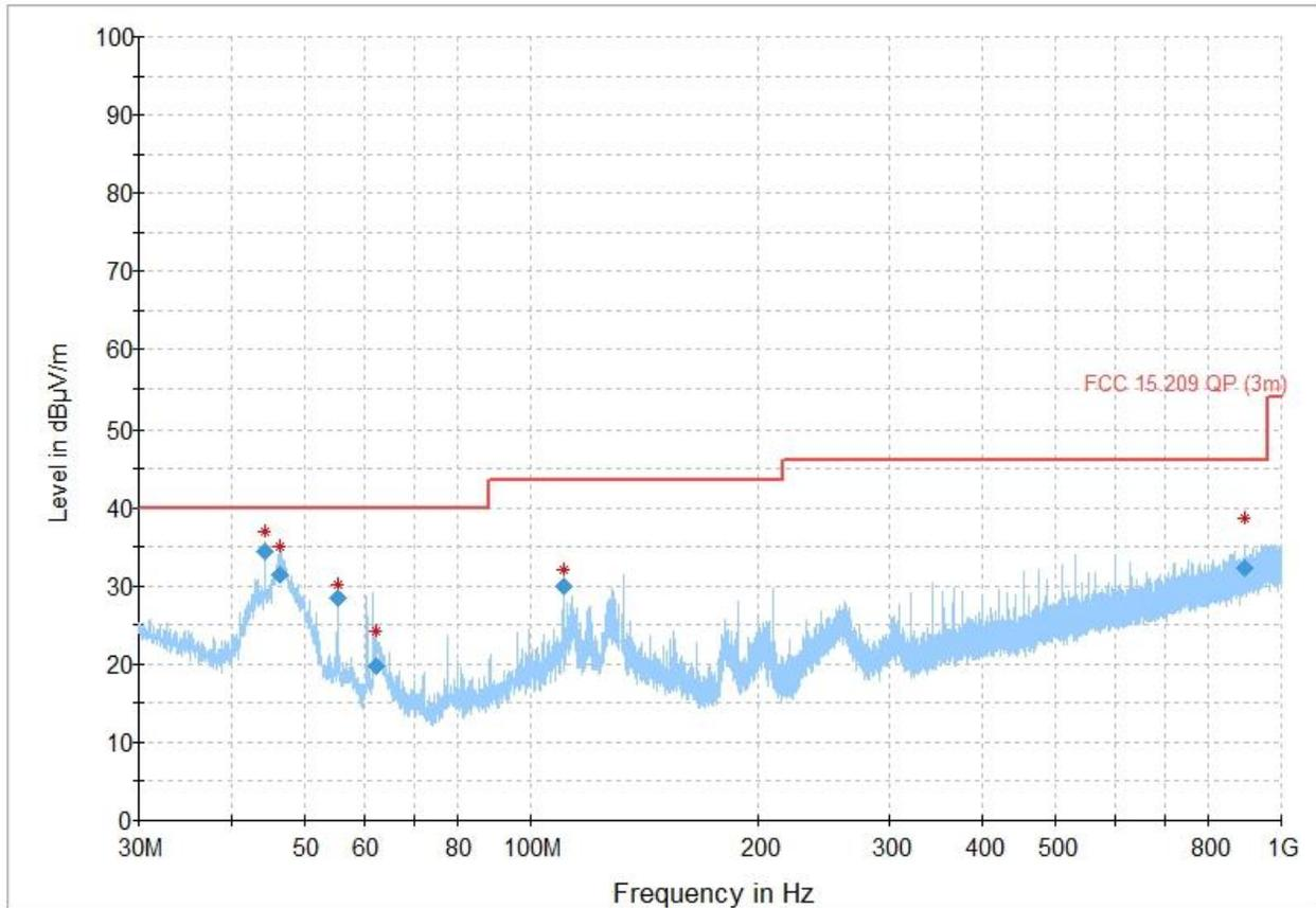
Figure 8.6-9: Radiated emissions, 2480 MHz, 30 – 1000 MHz
