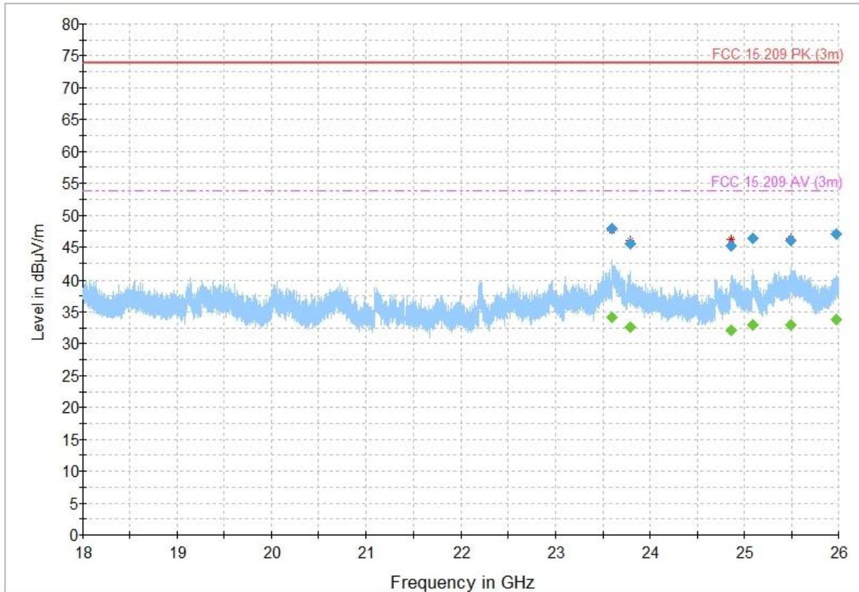
Figure 8.6-11: Radiated emissions, 2480 MHz, 18 - 26 GHz
