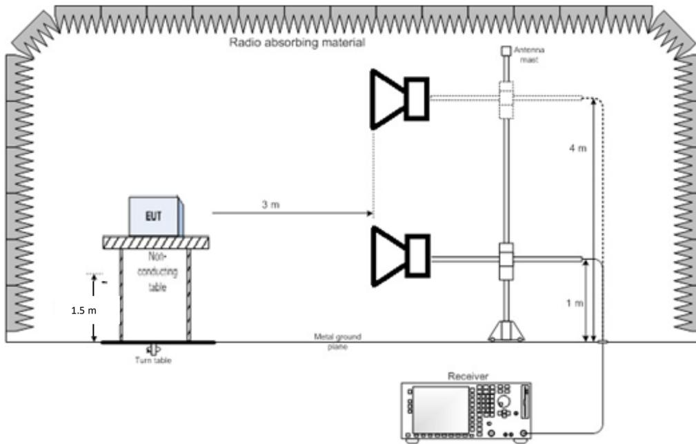
Figure 9.1-2 1 GHz - 26 GHz Setup
