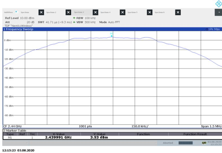
Figure 8.7-2: Power spectral density of digital transmission system, 2440 MHz
