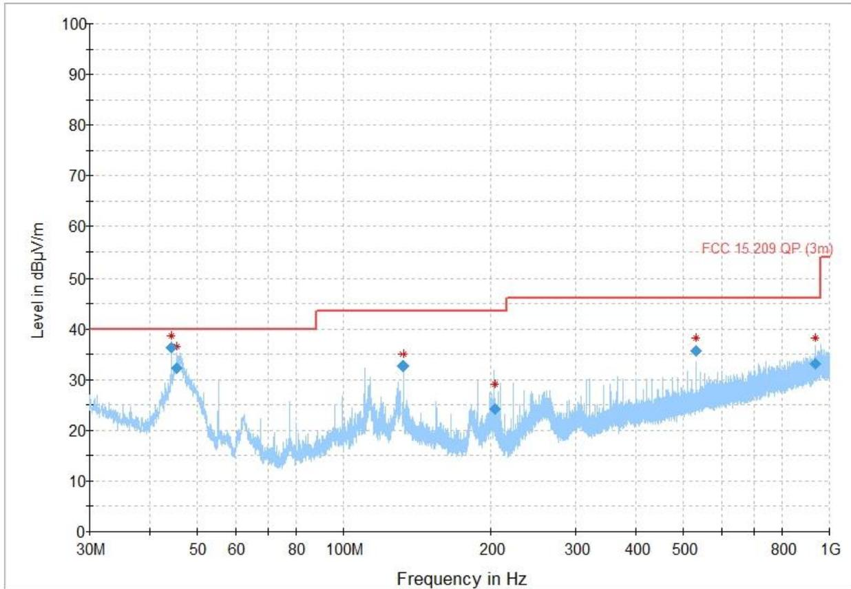
Figure 8.6-3: Radiated emissions, 2402 MHz, 30 – 1000 MHz
