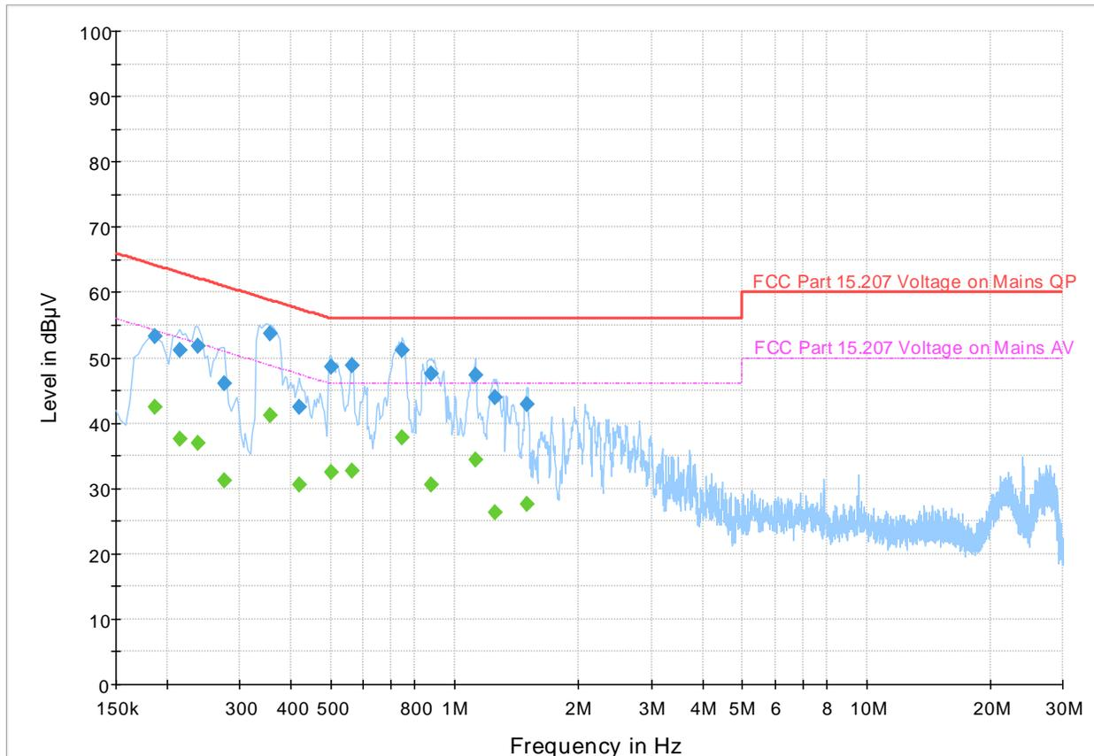
Figure 8.1-1: AC conducted emissions, 150 kHz – 30 MHz
