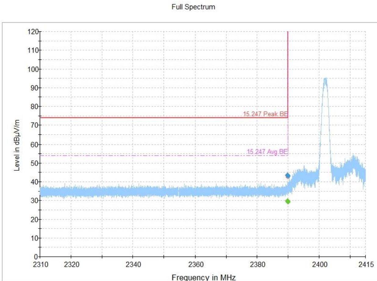
Figure 8.6-1: Radiated emissions, restricted band edge, low
