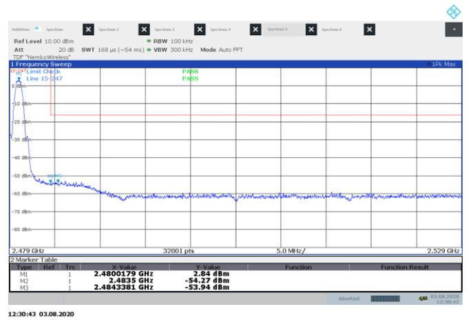
Figure 8.4-2: Conducted band edge measurement, 2480 MHz
