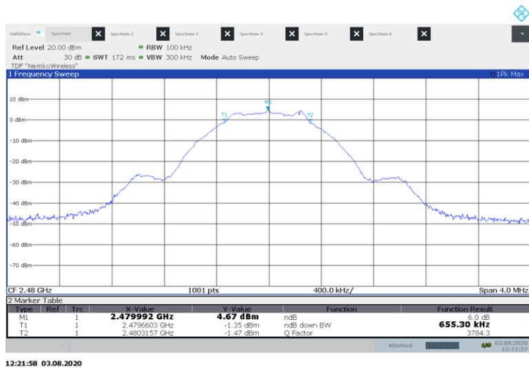
Figure 8.2-3: 6 dB occupied bandwidth, 2480 MHz
