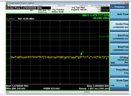
+3 dB above Out-of-band (single test signal) / 3.45 GHz Service (Ant2) / Downlink / 5G NR 40 MHz / Middle / Upper
