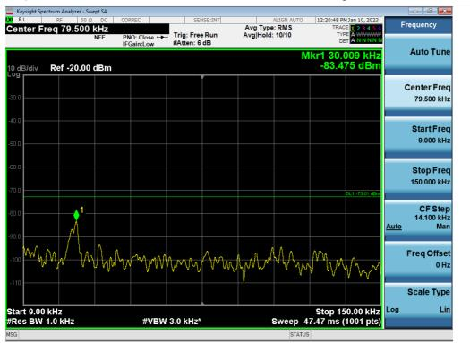
Spurious / 3.45 GHz Service (Ant1) / Downlink / 5G NR 60 MHz / High / 9 kHz ~ 150 kHz
