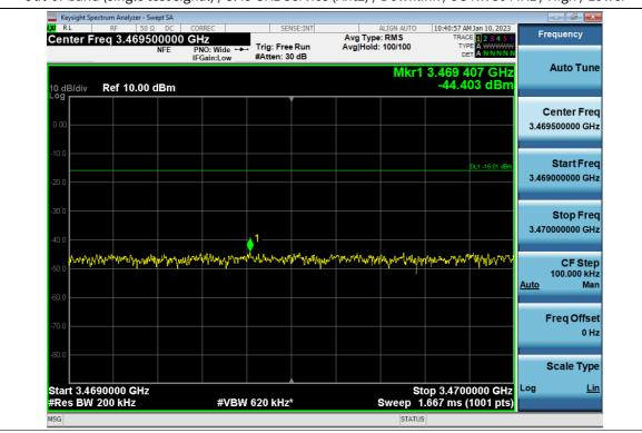
Out-of-band (single test signal) / 3.45 GHz Service (Ant2) / Downlink / 5G NR 80 MHz / High / Lower
