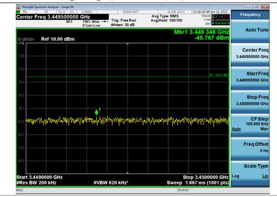
+3 dB above Out-of-band (single test signal) / 3.45 GHz Service (Ant1) / Downlink / 5G NR 80 MHz / Low / Lower
