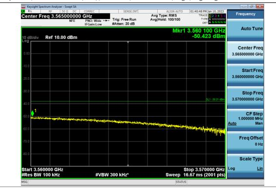
Spurious / 3.45 GHz Service (Ant2) / Downlink / 5G NR 20 MHz / High / High Edge + 10 MHz ~ 3 570 MHz
