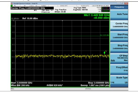
Out-of-band (single test signal) / 3.45 GHz Service (Ant1) / Downlink / 5G NR 80 MHz / Low / Lower
