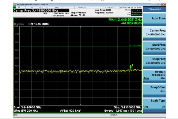
Out-of-band (single test signal) / 3.45 GHz Service (Ant2) / Downlink / 5G NR 40 MHz / Low / Lower
