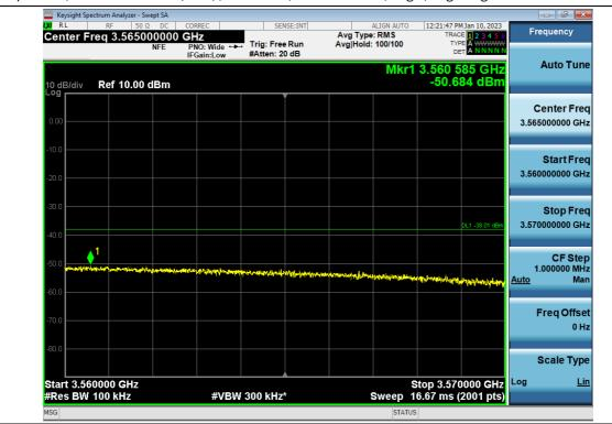
Spurious / 3.45 GHz Service (Ant1) / Downlink / 5G NR 60 MHz / High / High Edge + 10 MHz ~ 3 570 MHz
