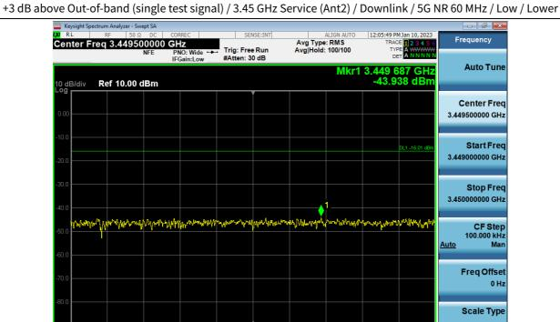
+3 dB above Out-of-band (single test signal) / 3.45 GHz Service (Ant2) / Downlink / 5G NR 60 MHz / Low / Upper
