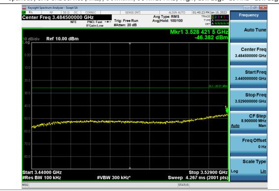
Spurious / 3.45 GHz Service (Ant2) / Downlink / 5G NR 20 MHz / High / Low Edge - 10 MHz ~ Low Edge
