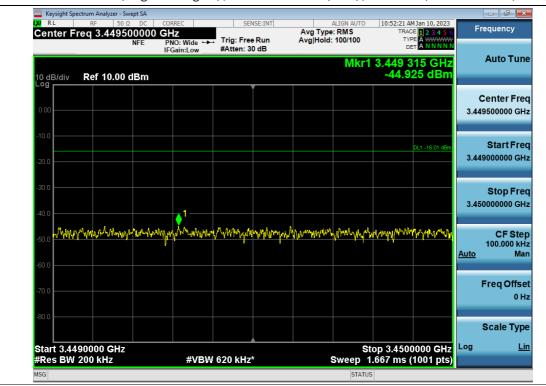
+3 dB above Out-of-band (single test signal) / 3.45 GHz Service (Ant2) / Downlink / 5G NR 80 MHz / Low / Lower
