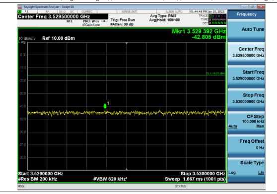
+3 dB above Out-of-band (single test signal) / 3.45 GHz Service (Ant2) / Downlink / 5G NR 20 MHz / High / Lower
