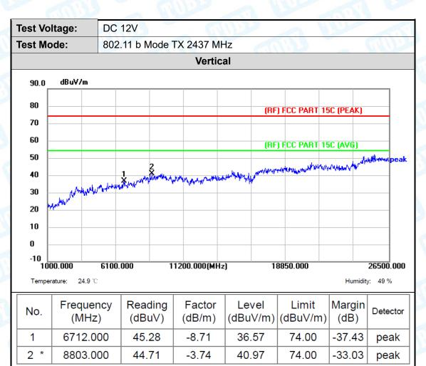
1. Corr. = Antenna Factor (dB/m) + Cable Loss (dB)
