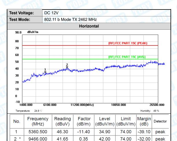
1. Corr. = Antenna Factor (dB/m) + Cable Loss (dB)
