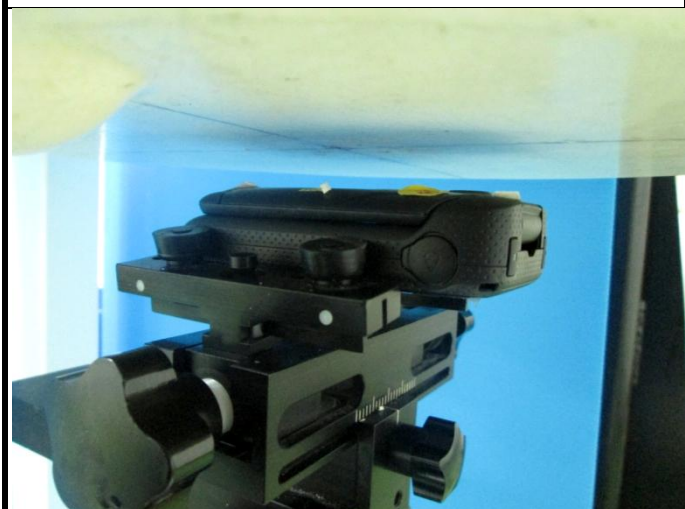
Front Face of EUT with 1.5 cm Gap
