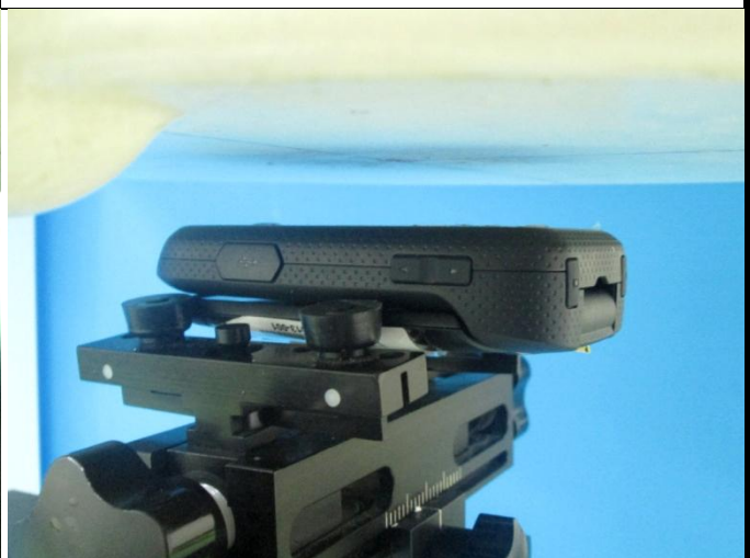
Rear Face of EUT with 1.5 cm Gap
