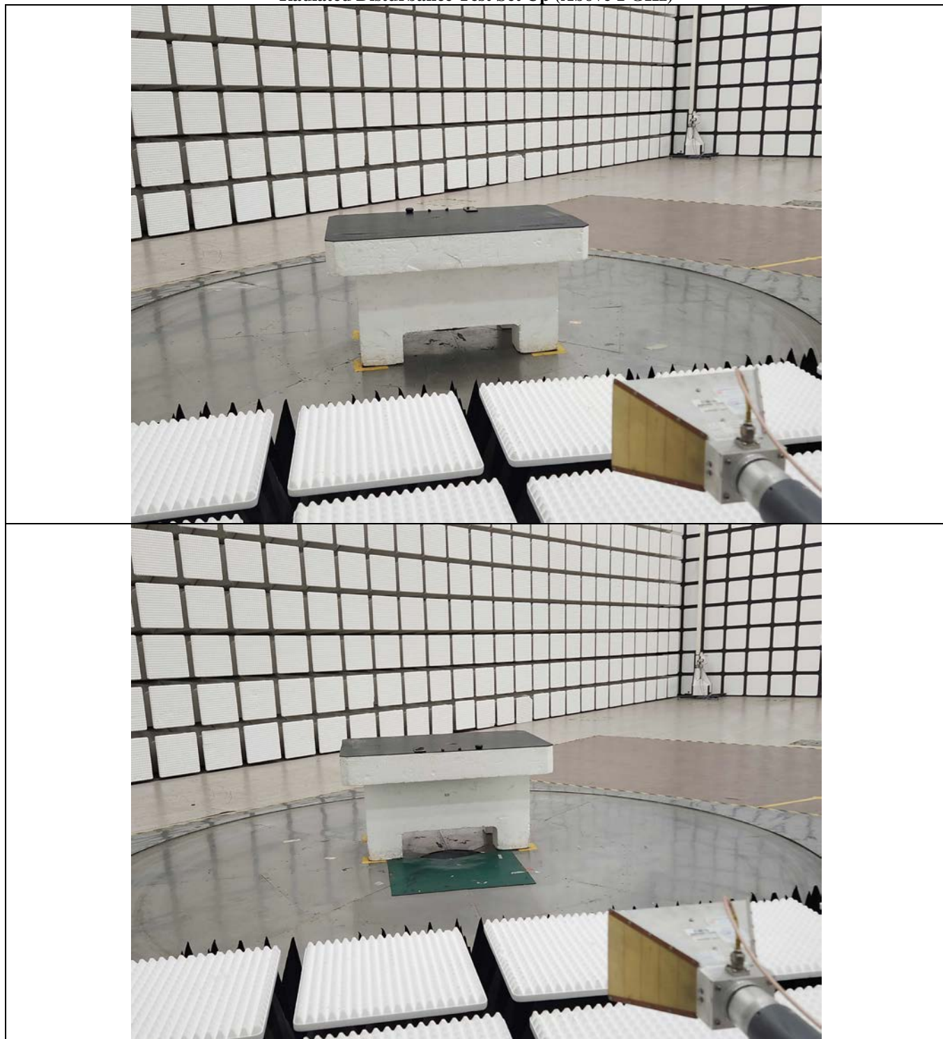
Radiated Disturbance Test Set Up (Above 1 GHz)
