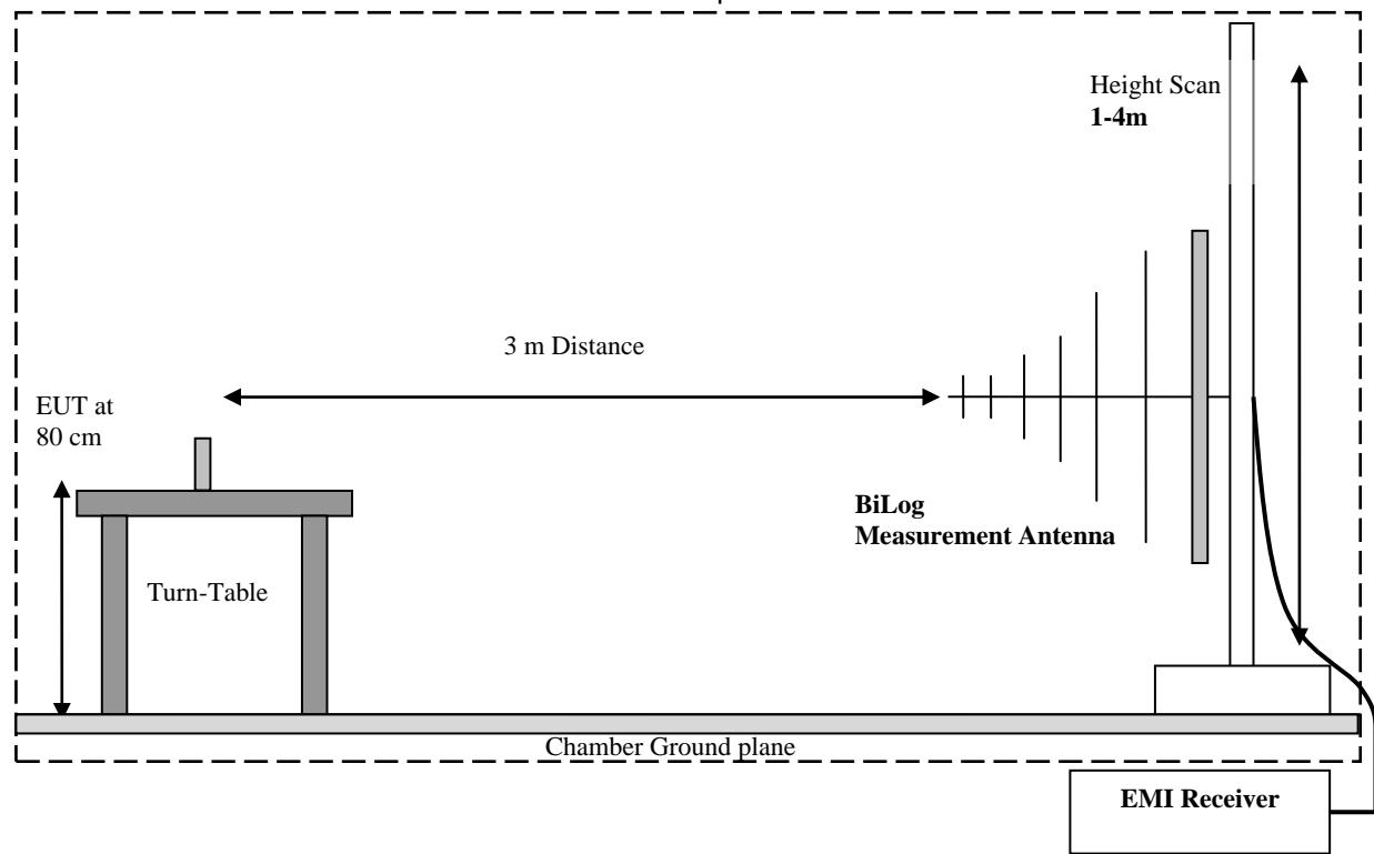
**Radiated Emissions Test Setup above 1GHz Measurements**
