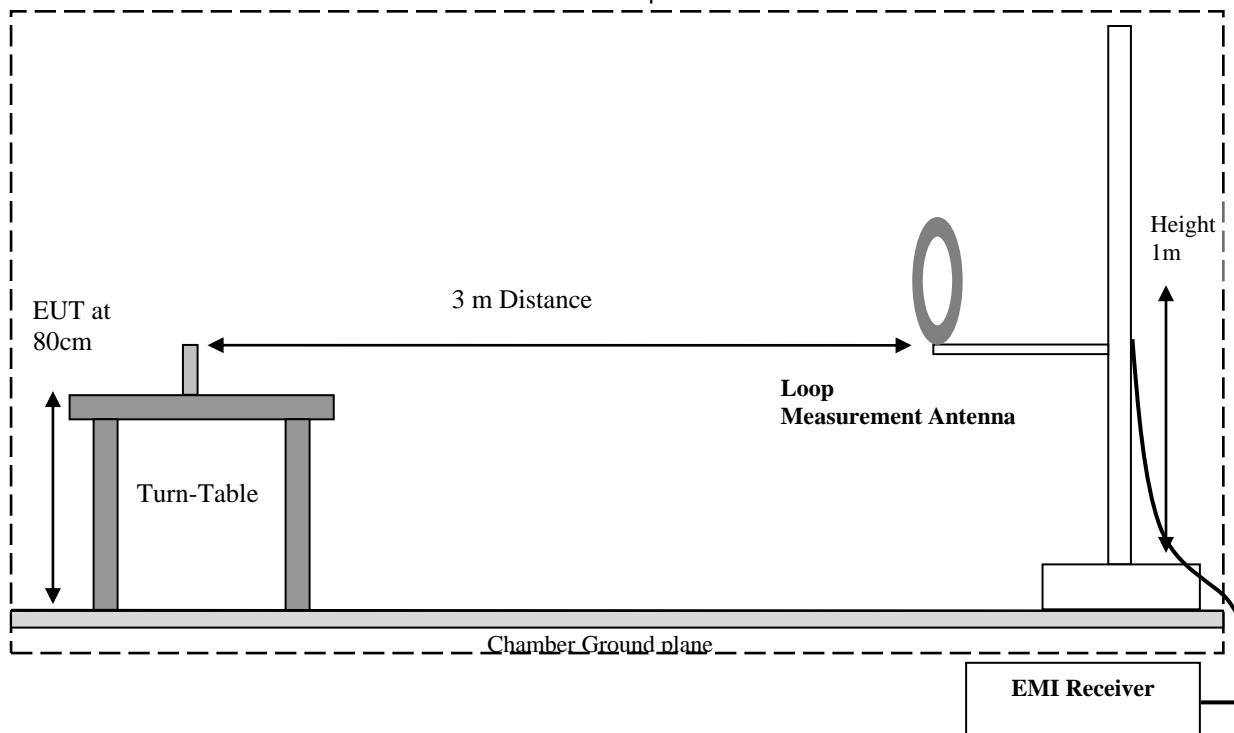
**Radiated Emissions Test Setup 30MHz-1GHz Measurements**
