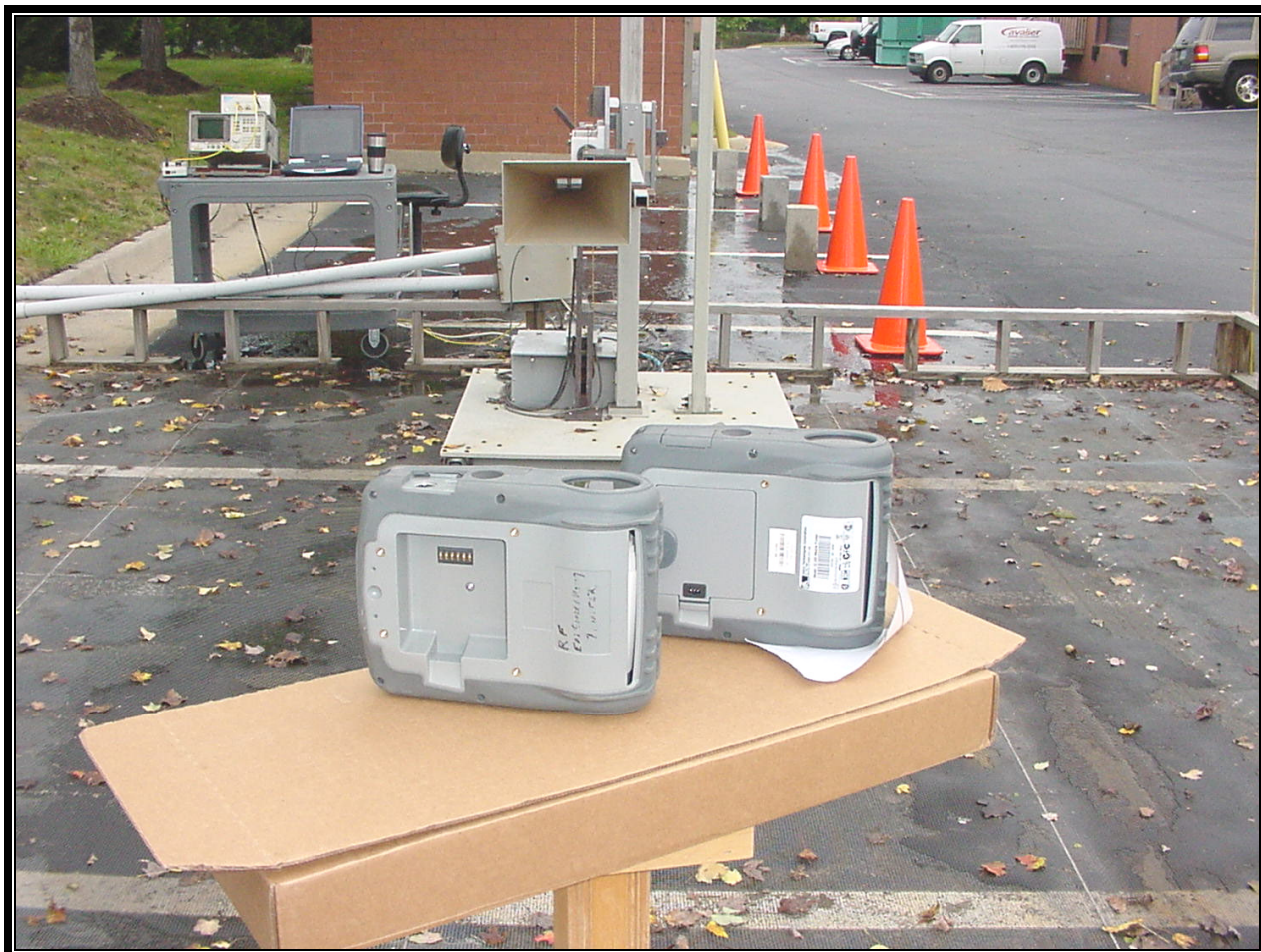
PHOTOGRAPH 17: RADIATED EMISSION REAR VIEW, WORST CASE CONFIGURATION QL FAMILY SECOND GENERATION BLUETOOTH (CQ17383-1) ANTENNA
