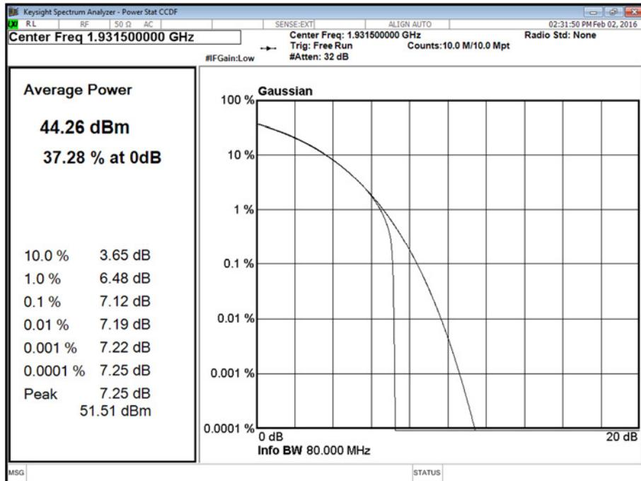
Channel Position B - Bandwidth 5.0 MHz - Antenna A
