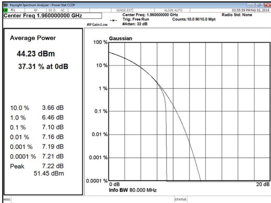
Channel Position M - Bandwidth 15.0 MHz - Antenna A
