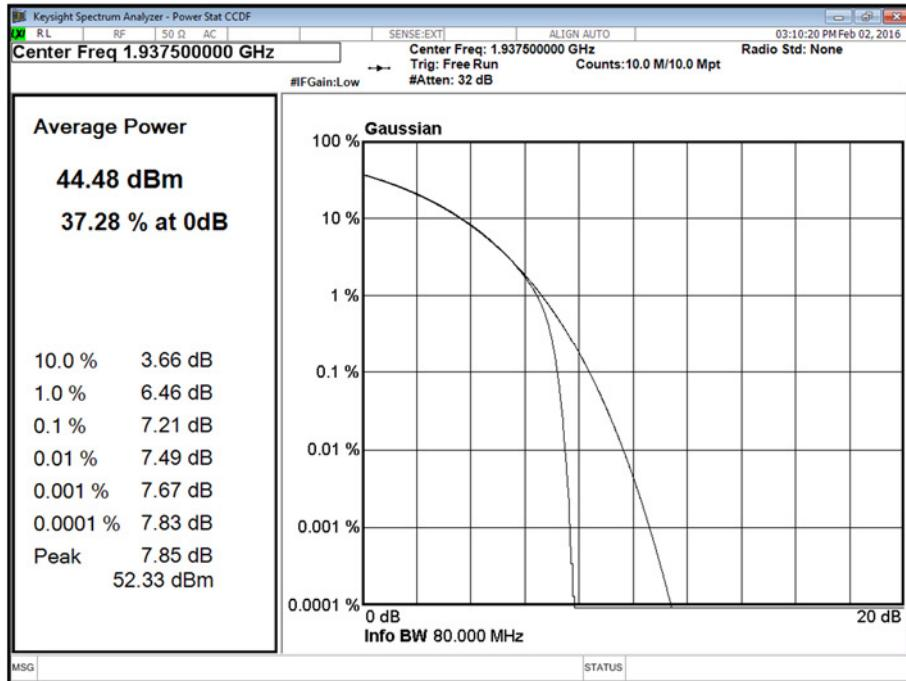
Channel Position B - Bandwidth 15.0 MHz - Antenna D
