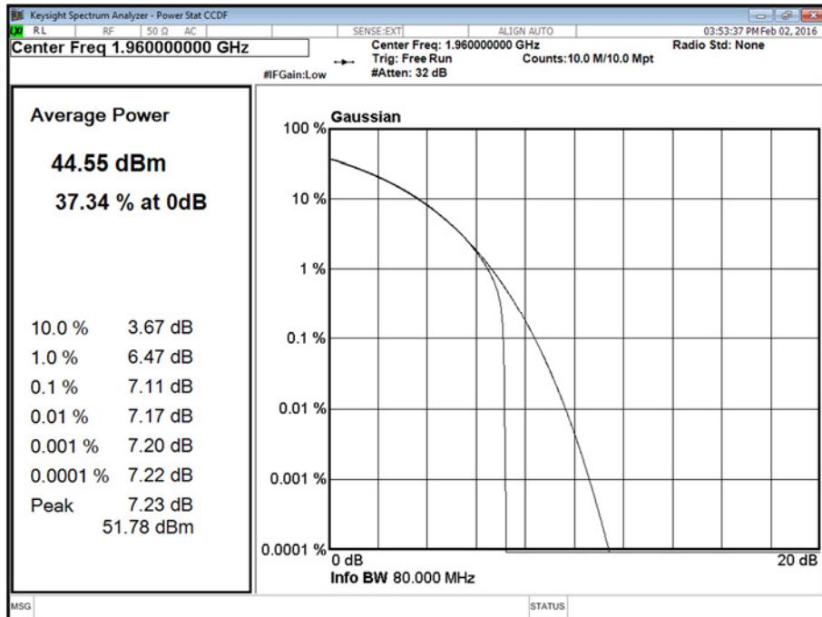
Channel Position M - Bandwidth 10.0 MHz - Antenna C
