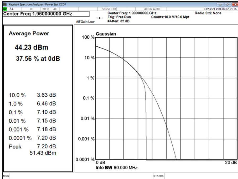
Channel Position M - Bandwidth 10.0 MHz - Antenna A
