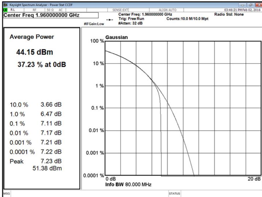
Channel Position M - Bandwidth 20.0 MHz - Antenna A
