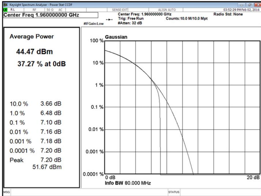
Channel Position M - Bandwidth 10.0 MHz - Antenna B
