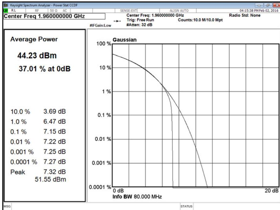
Channel Position M - Bandwidth 3.0 MHz - Antenna A
