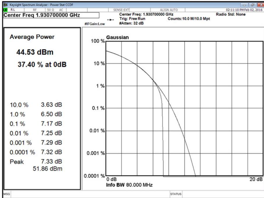
Channel Position B - Bandwidth 1.4 MHz - Antenna B
