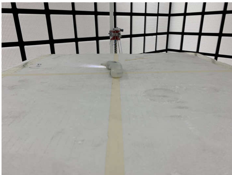
Radiated spurious emission Test Setup-2(Above 1GHz)
