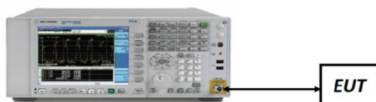
Figure 7-1. Test Instrument & Measurement Setup
