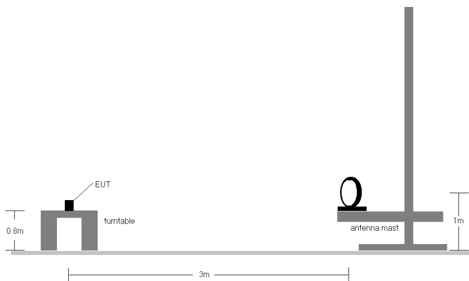
Figure 7-7. Radiated Test Setup < 30Mhz
