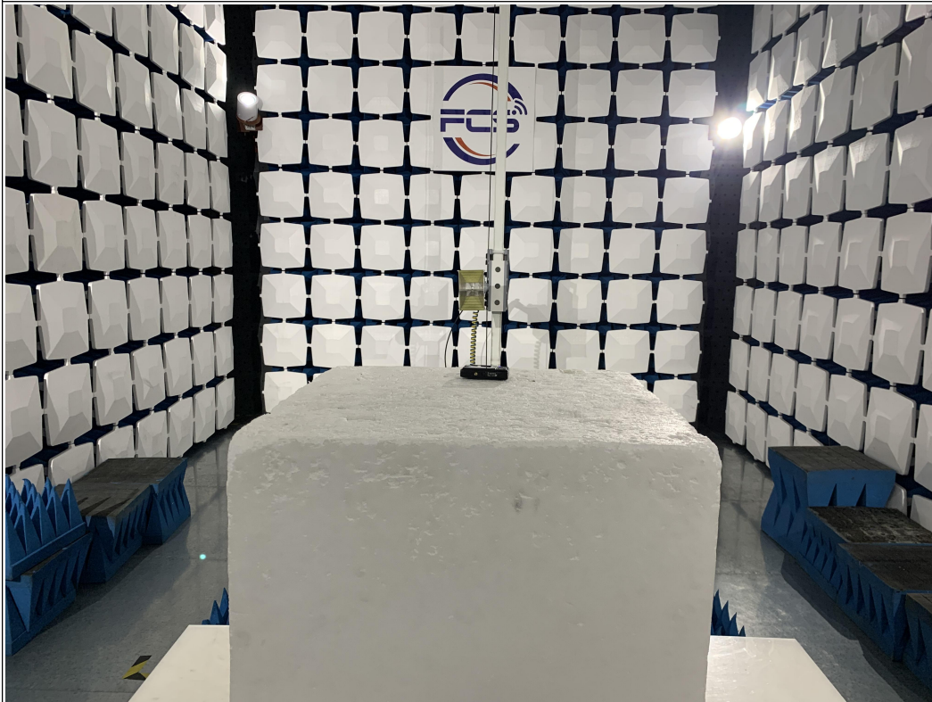
Above 1GHz for radiated emission test setup
