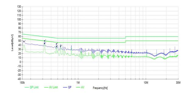
During the test, the Conducted Emission from 150kHz to 30MHz was performed in all modes with all channels, and all antennas. Bluetooth(LE\_1M), Channel 0, Antenna 1 are selected as the worst condition. The test data of the worst-case condition was recorded in this report.
