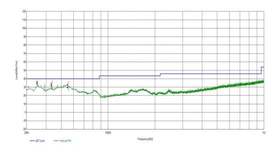
During the test, the Radiates Emission from 1GHz to 40GHz was performed in WIFI all modes with all channels and all antennas. BLE(1Mbps), Highest, medium, lowest channels, antenna 1 are selected as the worst condition. The test data of the worst-case condition was recorded in this report.
